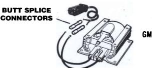
NOTE: CAREFULLY ROUTE THE ACCEL COIL HARNESS AWAY FROM ANY LINKAGE, AIR CONDITION LINES, HEATER HOSES, EXHAUST MANIFOLDS, ETC. BY USING THE MOUNTING HARDWARE INCLUDED IN THE KIT.
