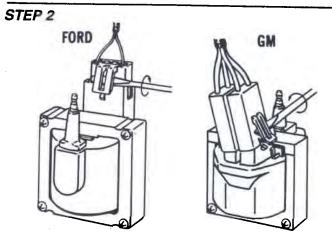
Remove electrical connector by carefully inserting a screwdriver between the connector lock tabs and with a twisting motion carefully pull outward.
