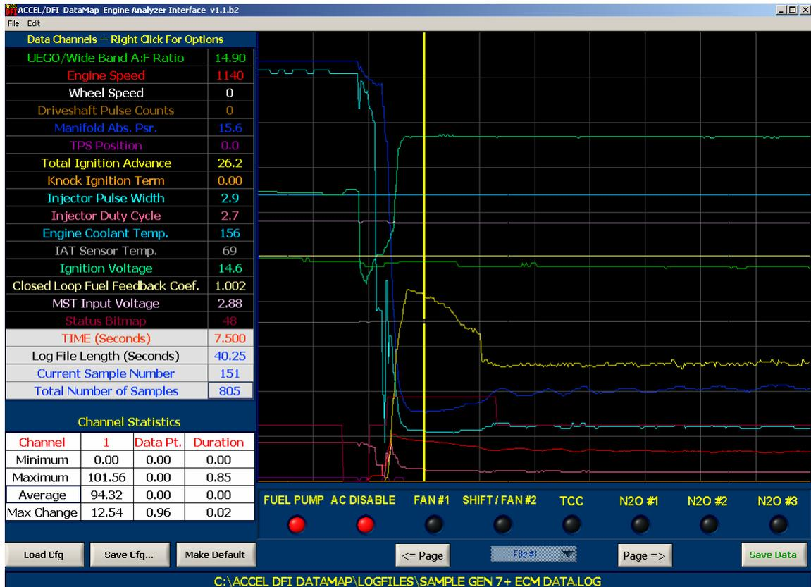
The DataMap software includes a 16-channel graph for displaying and analyzing the data recorded by your Engine Analyzer. From the File menu, select File->Graph Log File, or press the Analyze button after reading data from your Engine Analyzer to enter the DataMap Analysis screen.
