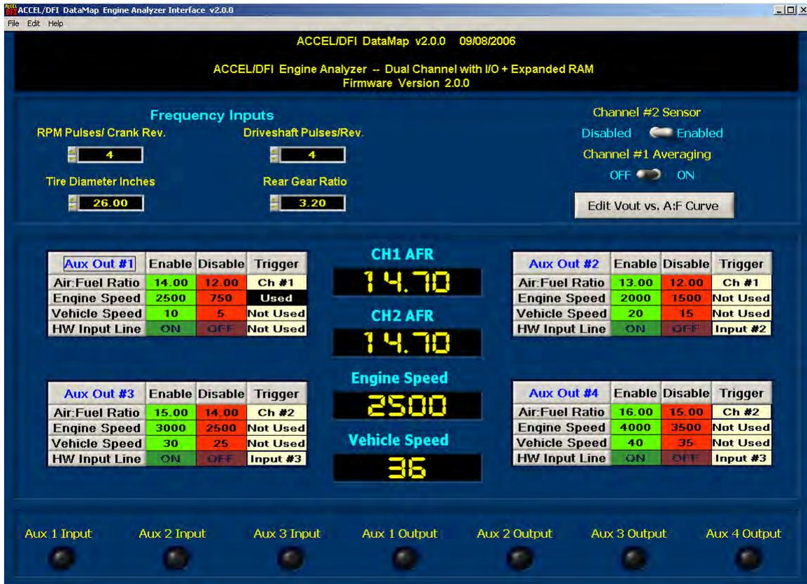
The Dual Channel Engine Analyzer includes 3 Auxiliary Inputs and 4 Auxiliary Output lines for controlling a wide variety of external functions. Each output is independently configurable and can utilize any input line as its hardware enable switch. The Dual Channel I/O Configuration Screen can be accessed by pressing the CTRL + I keys, or selecting the File->Configure Dual Channel I/O menu item.
