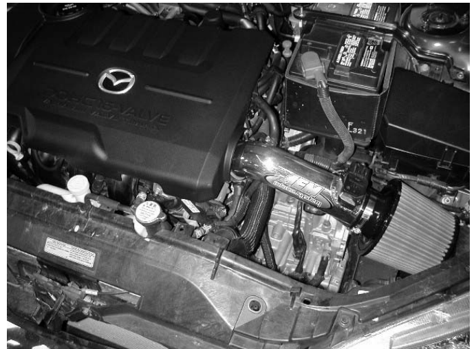
n) Reinstall engine cover. AEM SRS kit installed.
