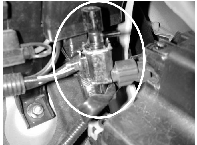
h) Remove the vacuum solenoid from the air box. Remove all vacuum lines from the solenoid. Plug green connector back into solenoid and secure it to a wiring harness utilizing the supplied zip tie.
