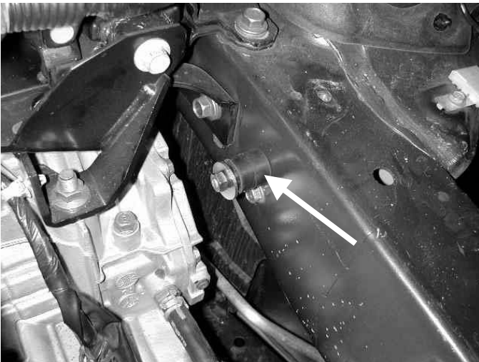
g) Install supplied rubber mount as shown.
