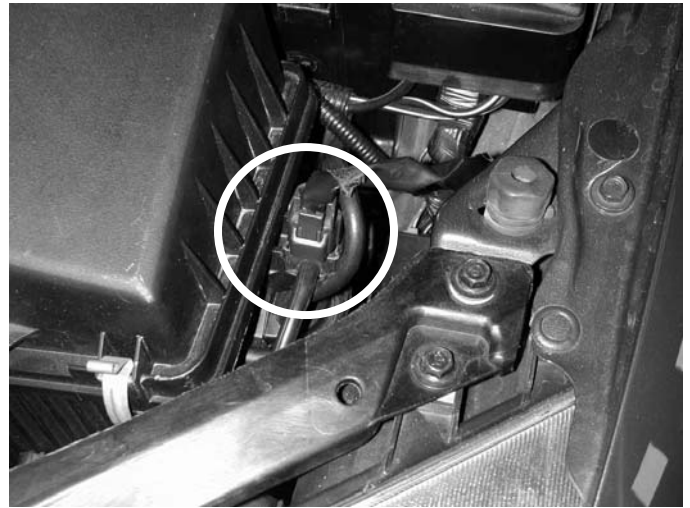
b) Release the green plug on the vacuum solenoid located next to the air box.
