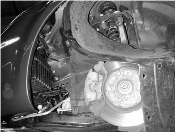
l) Place the fender liner as shown.
