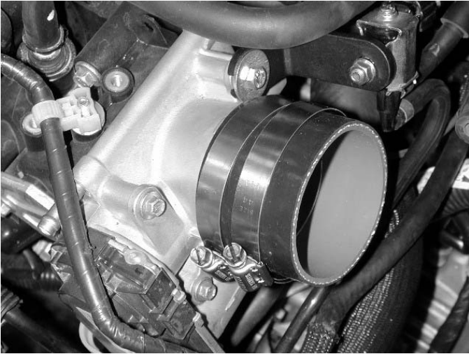
e) Install the supplied silicone hose onto throttle body.
