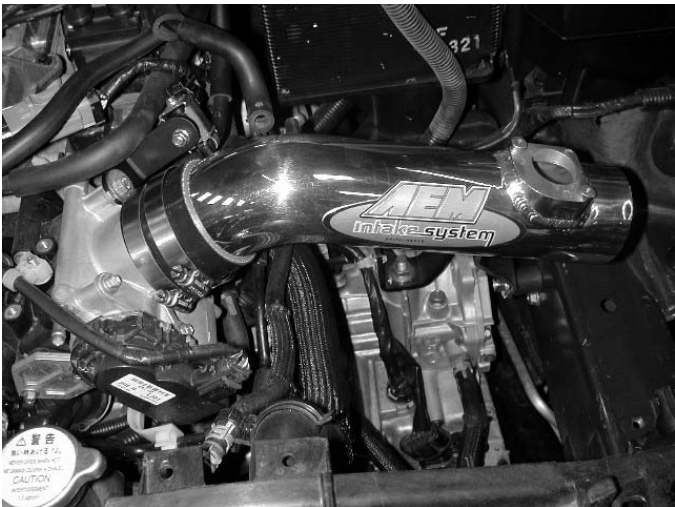
h) Install pipe as shown. Do not tighten hose clamps!
