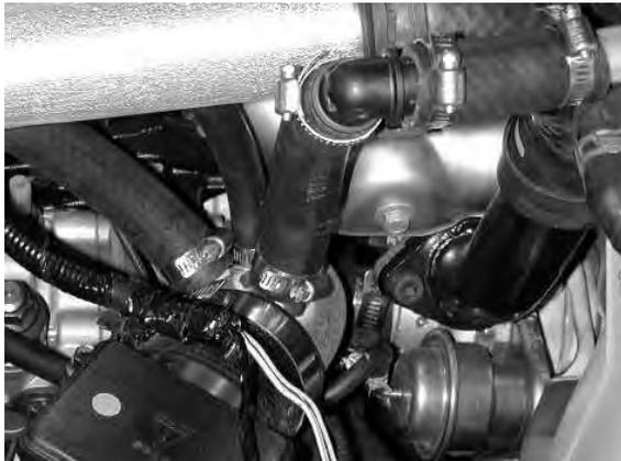
k. Install supplied 3/4" and 5/16" hoses onto inlet pipe as shown. Use supplied spring clamps and screw clamps as shown.
