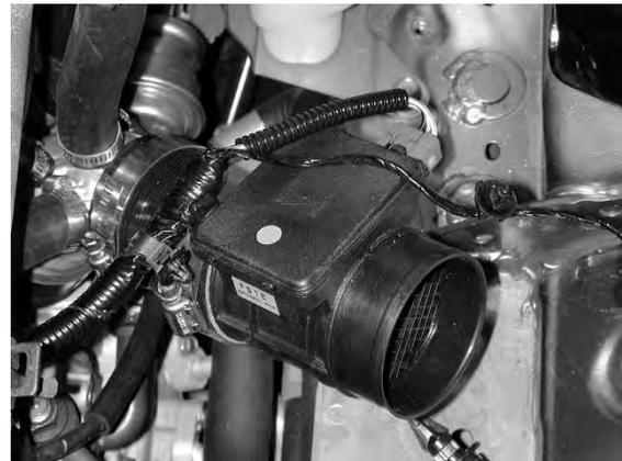
e. Install the MAF assembly from step 3C onto inlet pipe. The MAF bracket will install on to the rubber mount using the supplied M6 Nylok nut.
