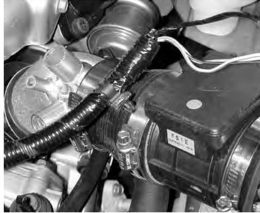
g. Remove the electrical tape as shown.
