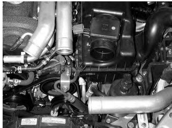
d. Remove the boost pipe elbow and the inlet tube. You will reuse the boost side elbow during the **AEM** intake install.
