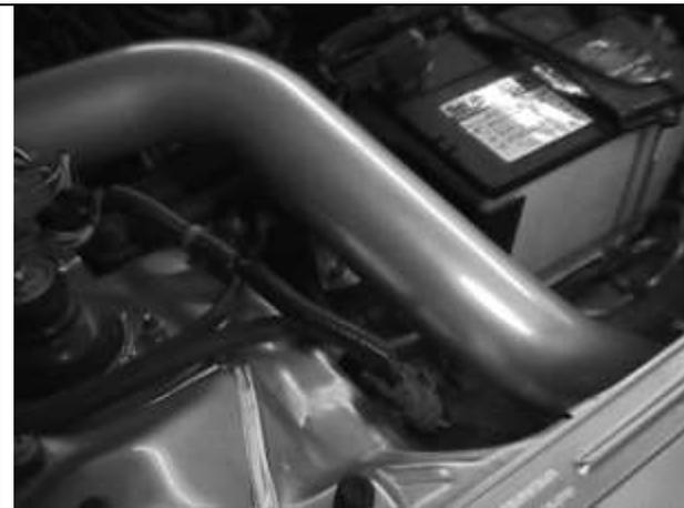
Fig 11: Intake pipe installed. Note mounting bolt.
