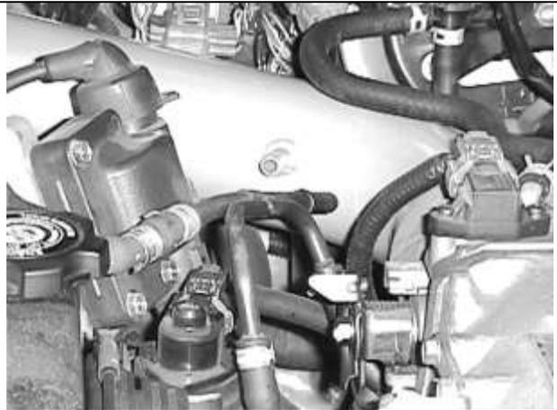
Fig 10: Breather tube and port on intake tube.
