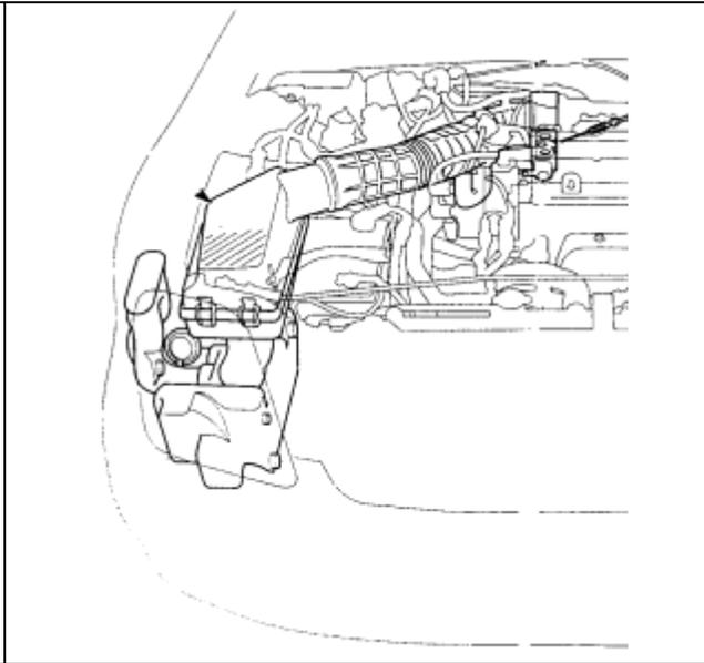
Fig 4: Air box system layout (front)
