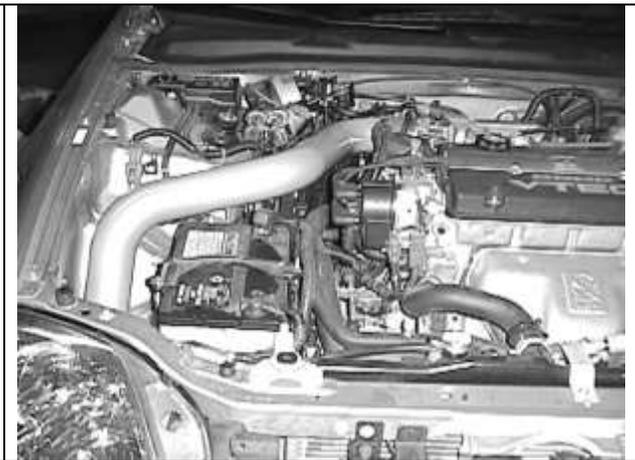
Fig 8: Intake tube installed
