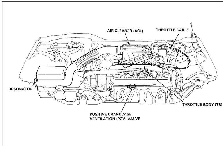
Fig.3: Air inlet layout
