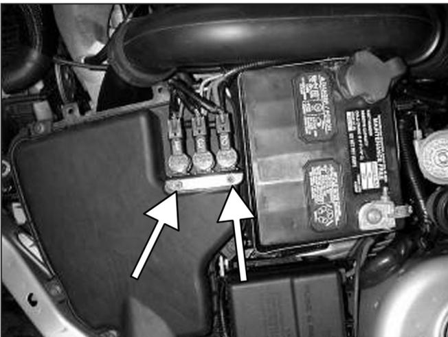
i. Remove the 2 screws holding down the vacuum assembly to the air box.
