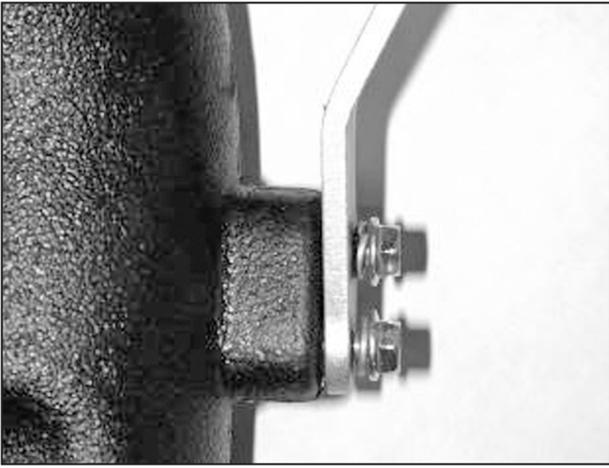
t. Attach the bracket for the plastic lower intake pipe with the provided hardware. Use two of the M6 hex/ flange bolts and lock washers.
