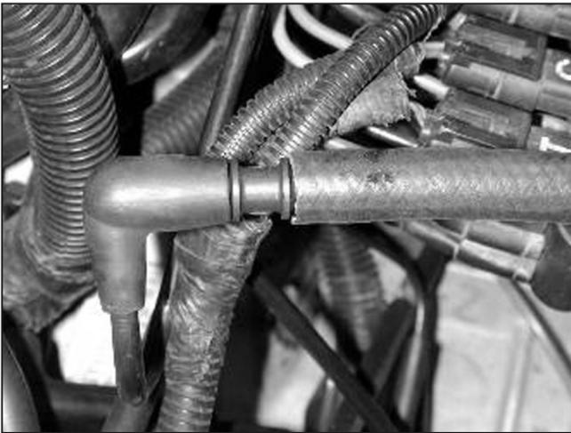
l. Insert the straight barded fitting into the vacuum cap from step 2d. Attach the 3/8" diameter breather hose to the other end of the barbed fitting.
