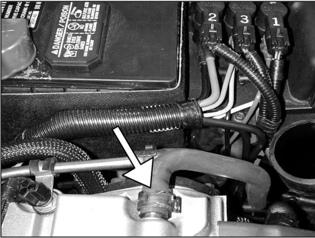
e. Remove the breather hose from the nipple on the valve cover. Check for oil, if present clean as necessary.
