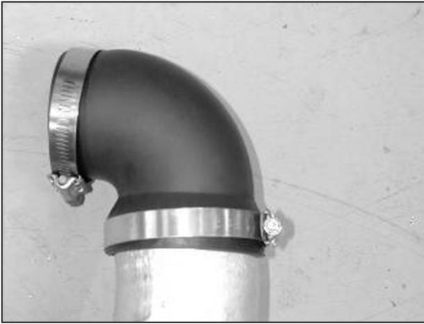
f. Attach the 3" side of the silicon elbow to the inlet pipe. Secure the elbow to the inlet pipe with the included hose clamp. The open end connects to the turbo inlet which sits horizontal. This opening is furthest away from the bracket.
