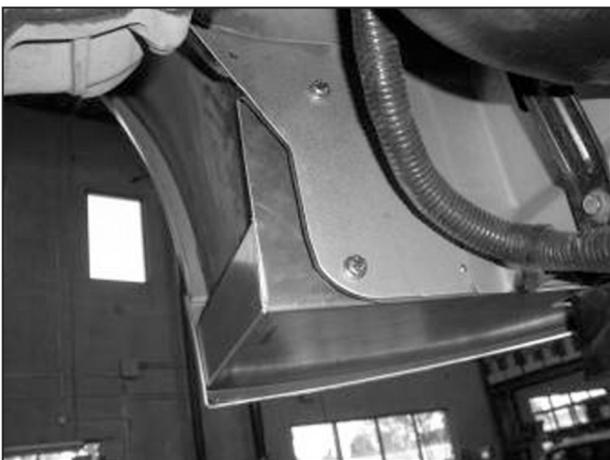
ad. Secure the splashguard with the flange bolt, washers and nut. The fender liner will tuck inside the splashguard.
