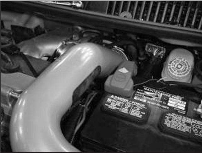
j. Check for clearance around the battery, all breather hoses and hard lines. You should have at least 1" of clearance from the inlet pipe and the positive battery terminal. If not you will need to readjust the battery to the further most right position on the battery tray. **If the terminal cover is damaged, cracked or melted you will need to replace immediately before installation. Failure to abide by Step 3j will void all warranty.**
