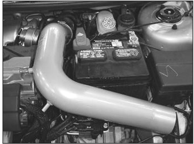
i. Insert the inlet pipe. Attach the coupler to the turbo and line up the bracket to the rubber mount.
