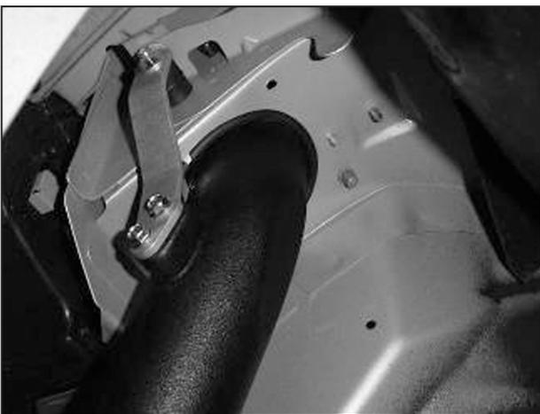
x. Secure the bracket on the rubber mount with a washer and nut.
