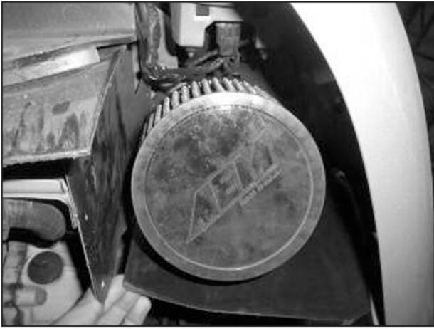
z. Attach the air filter element to the lower end of the intake pipe. Secure with the a hose clamp.
