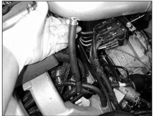
m. Secure the other end of the breather hose to the upper inlet pipe with the provided hose clamp.
