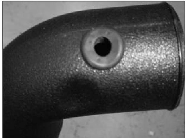
s. Insert the rubber grommet into the small hole in the plastic lower intake pipe.
