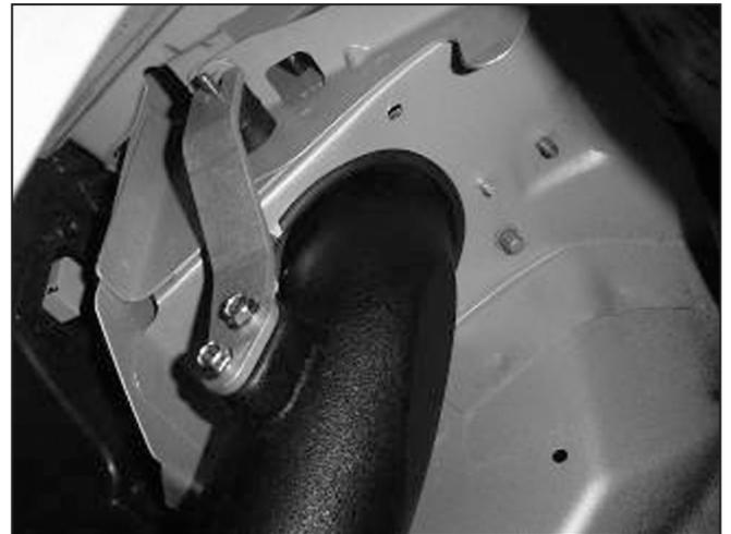
w. Line up the bracket with the 1" rubber mount from the inner fender side.
