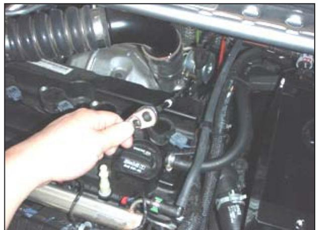
ac. Position the inlet tube, air horn and filter assembly for clearance around surrounding components. Once the optimal position is set, tighten the hose clamps on the hose adapter at the turbo-charger and the nut on the inlet tube bracket.
