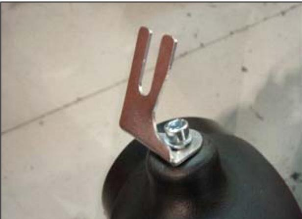
h. Bolt the inlet tube bracket to the inlet tube and secure with a socket head M6 screw and M6 x 12 O.D. washer.
