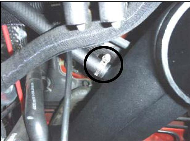
t. Install the PCV hose on the nipple on the inlet tube and secure with the 1" hose clamp.
