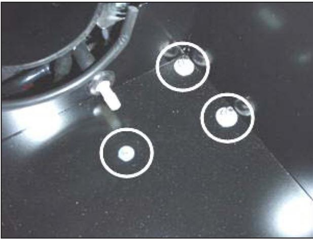
x. Seat the air box on the three threaded M6 studs and install a M6 hex nut on the bolt to the left. Install the M6 hex nuts removed in step 2o on the two studs to the right.
