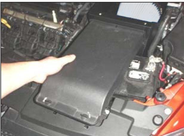
ab. Install the factory air inlet duct by inserting the duct into the air box opening and then the two clips into their factory mounting position. Twist the two clips to secure the duct.
