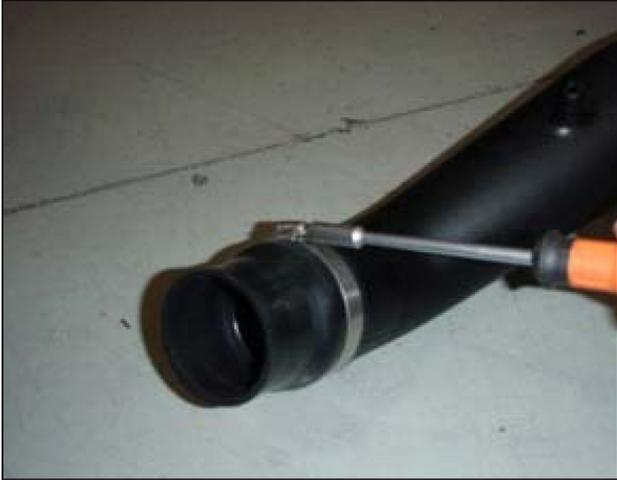
b. Install the 2.50" to 3.00" hose adapter on the inlet tube and make sure it's fully seated. Place a #48 hose clamp on the larger diameter side of the hose adapter and lightly secure allowing the clamp to be rotated but not able to slip off.
