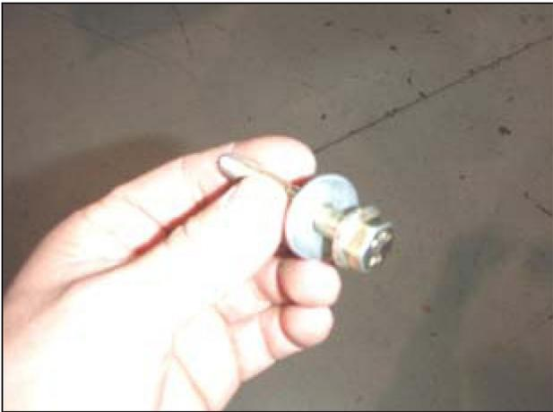
d. Prepare a M8 washer on the flanged M8 bolt for the following step.
