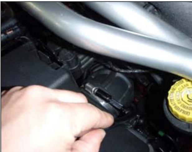
k. Loosen hose clamp securing the factory inlet tube to the air box assembly. Disconnect the inlet tube from the air box.
