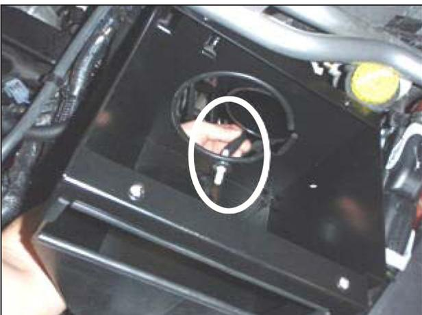
v. Place the air box into the engine bay close to where the factory air box originally sat and at the same time, reach under the box and connect the rubber hose that was disconnected in step 2j to the white plastic connector.
