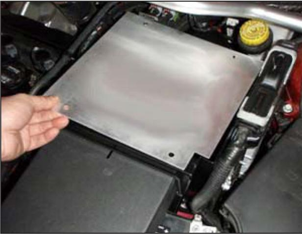
ad. Place the AEM® lid above the air box and make sure the tab on the upper left hand corner holds the factory sensor bracket in place.
