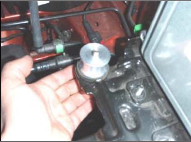
f. Slide the .93" tall aluminum stand on to the grommet and the hardware, support the bolt from the bottom so it doesn't slip out (Two aluminum stands are provided in this kit, this step uses the taller one).
