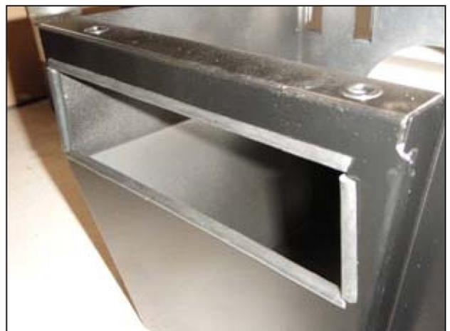
k. With the rubber edge trim, cut and install on all four edges of the air box opening as shown.
