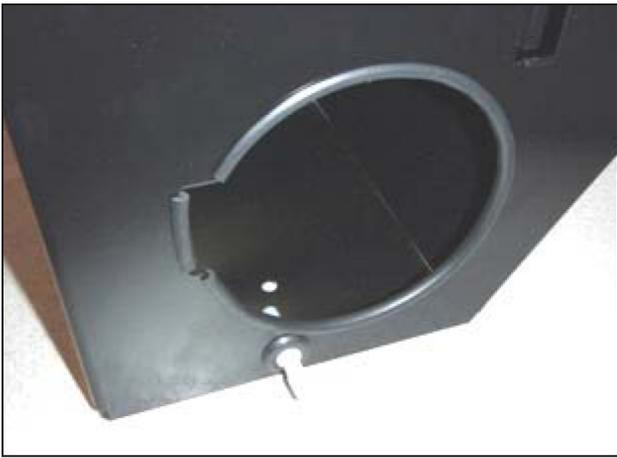
l. With the rubber edge trim, cut and install on the large circular opening as shown. Install the  $\frac{3}{4}$ " ID grommet in the hole below the large opening and slip in the white plastic connector as shown, the fit will be snug.
