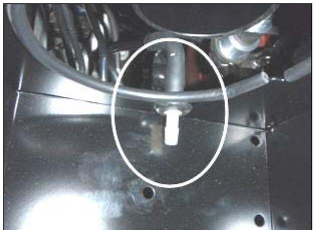
w. Properly connected rubber tube in previous step should look like this, make sure the plastic connector is snug and centered in the grommet.
