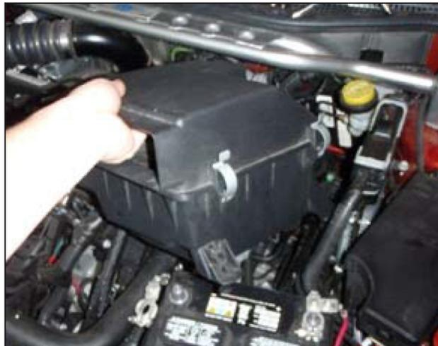
l. Remove factory air box assembly as a whole by pulling upward; the air box is held in place with rubber grommets.
