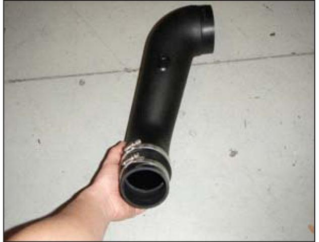
c. On the smaller diameter side of the hose adapter, place a #40 hose clamp and lightly secure. Make sure the clamp can still be rotated. Angle both clamps in the position as shown, this will allow them to be tightened down in the vehicle with ease.
