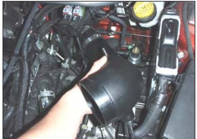
i. Install the inlet tube. Start by lining up the hose adapter to the turbocharger inlet and then the bracket to the rubber mount installed in step 3g.
