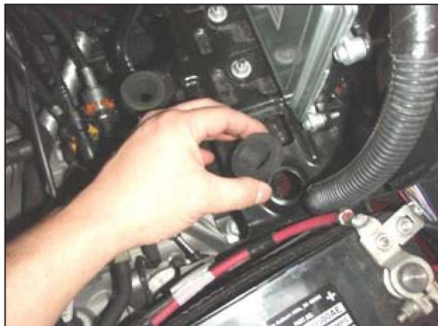
n. There are 3 grommets on the pan that hold the factory air box. The center and rear one will need to remain on the vehicle for the AEM® air intake system. Remove the grommet that is closest to the battery.
