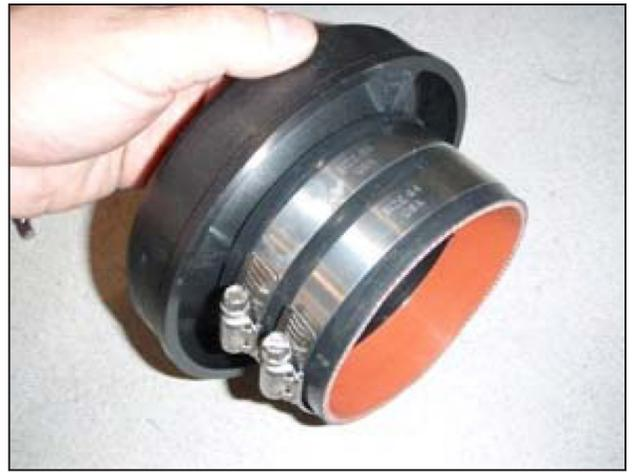
y. Assemble the air horn and 4" diameter coupler, place two size 64 hose clamps in the exact position as shown. Tighten down the clamp closest to the air horn.
