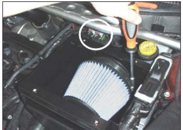
aa. Install the air filter onto the air horn and use a size 104 clamp to secure. Slide the sensor assembly (circled) on to the rear of the air box.
