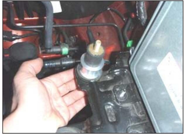
g. Install the 8mm x 1" tall rubber mount and tighten the assembly.
