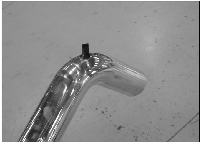
f. Install the supplied duck-bill drain into the 1/2" hole on the lower intake pipe. This drain prevents water from building up in the bottom of the intake pipe due to the angle in which the filter is placed.
