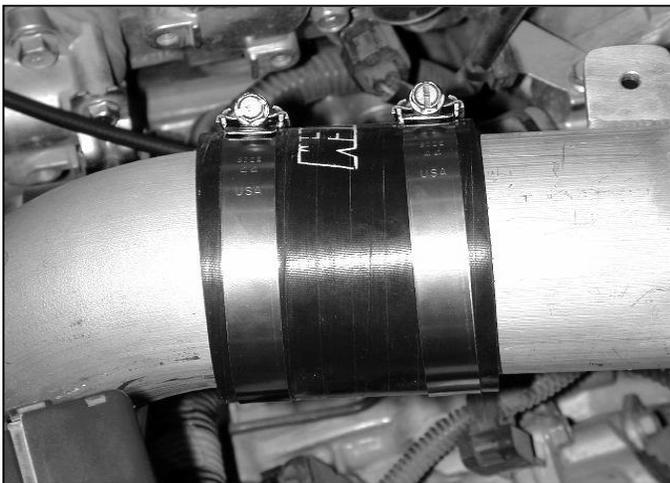
g. Attach the upper and lower pipes together with the coupler installed in the previous step.
