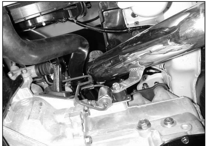
l. Ensure the air filter is not touching any part of the vehicle. Position the AEM<sup>®</sup> intake for best fitment. Be sure that the pipe or any other component is not in contact with any part of the vehicle. Tighten the hose clamps at the throttle body and silicone coupling. Tighten the nut on the mounting bracket. Re-adjust the pipe if necessary.
