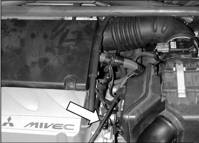
c. Remove the breather hose from the valve cover by pulling it off.
