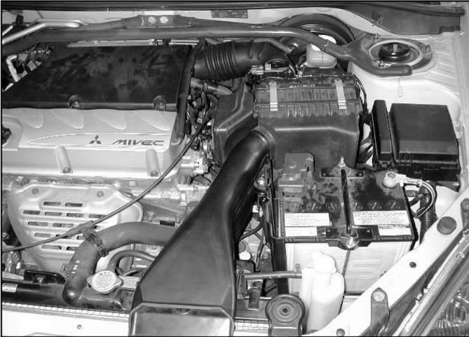
Factory air box system installed
