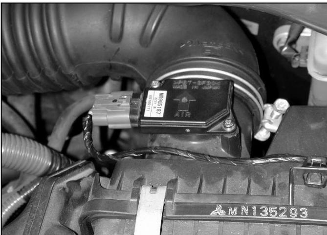
g. Unplug the MAF sensor from the engine harness.
