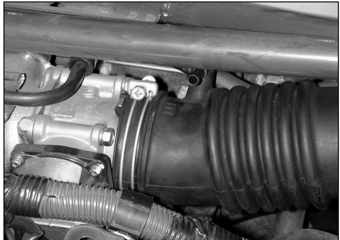
f. Unscrew the inlet tube from the throttle body and pull the inlet tube off the throttle body.
