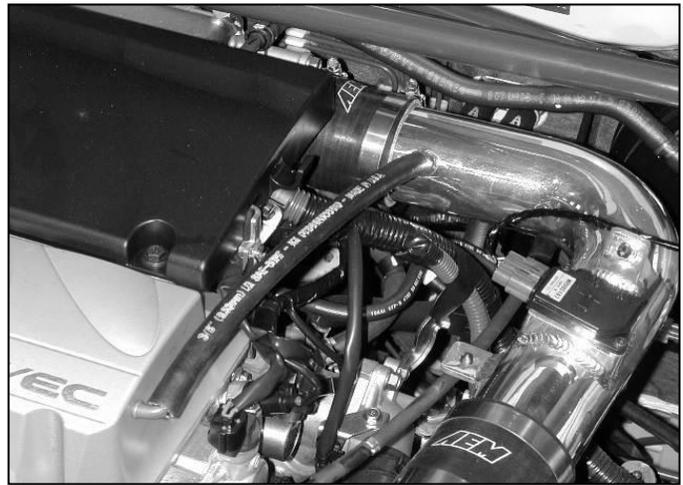
j. Plug in the MAF sensor and secure the wiring harness using the supplied tree mount zip tie. Install the supplied 3/8" breather hose onto both the valve cover nipple and the pipe nipple. Use the supplied 3/4" hose clamps to secure. Trim for proper fitment. Secure the throttle cable using the supplied tree mount zip tie. Trim the excess plastic zip strap.
