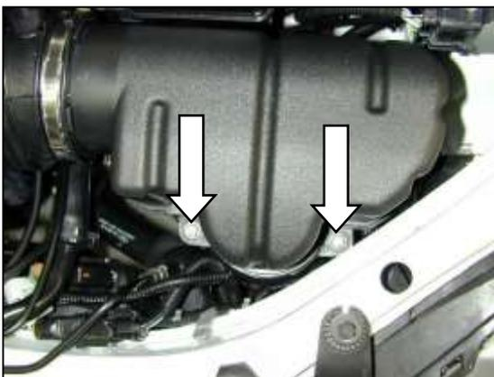
c. Loosen the two bolts that secure the upper airbox.
