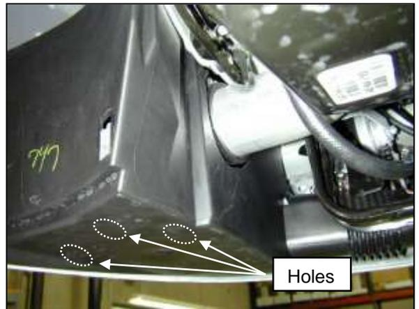
k. Reinstall the splash shield. Drill 1/2" holes in the bottom of the splash shield to facilitate water drainage.
