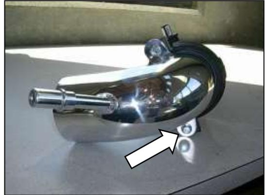
c. Secure the upper inlet pipe to MAF housing with the supplied bolts.
