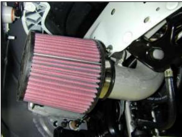
j. Secure the AEM<sup>®</sup> air filter onto the end of the lower intake pipe with the provided hose clamp.
