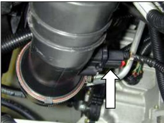
f. Connect the MAF sensor wire harness to the MAF sensor.
