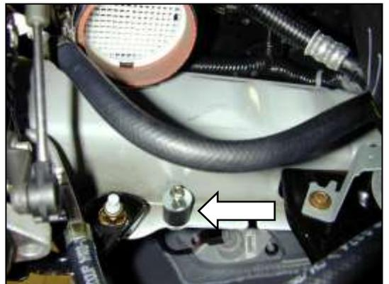
g. Install the rubber mount into the frame rail with a supplied washer and lock nut.
