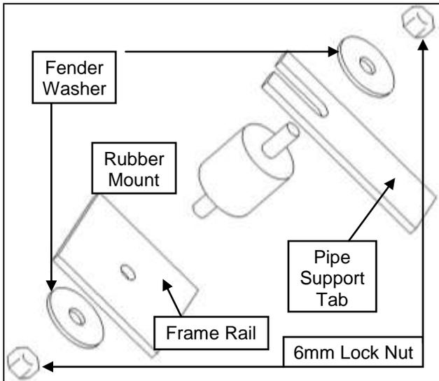
h. Proper installation of the rubber mount assembly.
