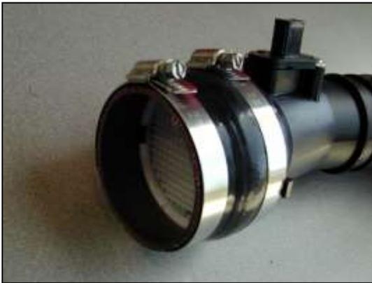
d. Attach the silicone reducer onto the MAF sensor housing.
