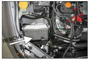
10. Remove the remaining half of the factory airbox.
