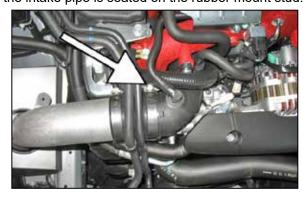
22. Slide the silicone coupler onto the compressor inlet pipe. Orient the hose clamps on the compressor inlet as shown and tighten securely.
