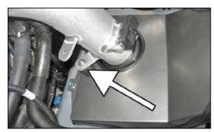
24. Secure the inlet pipe to the rubber mount with the supplied fender washer and M6 nut, but do not completely tighten.
