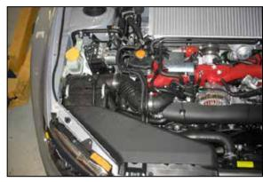
2. Remove the two plastic clips and factory fresh air inlet duct.
