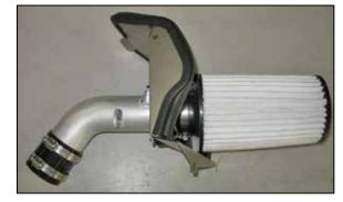
20. Install the silicone coupler and two #44 hose clamps onto the intake pipe. Orient the hose clamps as shown but do not completely tighten.
