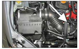
8. Loosen the hose clamp securing the factory airbox inlet to the compressor inlet tube.
