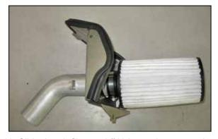
18. Slide the air filter and #48 hose clamp onto the end of the pipe until the pipe hits the intake pipe stop.
