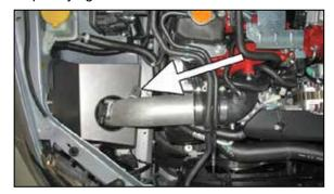
25. Align the intake pipe so it is centered within the heat shield's inlet hole. Tighten the M6 nut to secure the rubber mount assembly.
