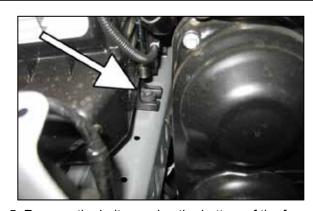
5. Remove the bolt securing the bottom of the factory airbox.
