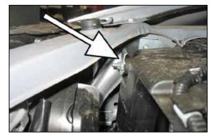
3. Loosen the nut securing the factory airbox mounting bracket but DO NOT remove the nut.
