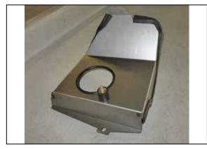
14. Install a M6 rubber mount on the heat shield and secure with supplied M6 nut.
