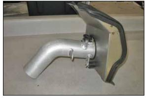
17. Insert the AEM® intake pipe through the large hole in the heat shield.
