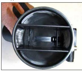
16. Apply four drops of the provided super glue around the lip of the Maf insert and then insert the maf insert into the intake tube so that it aligns with the maf sensor as shown.
