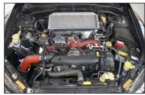
30. AEM® intake system installed
