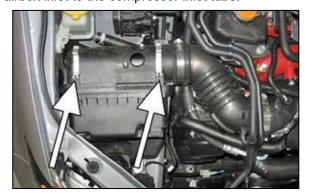
9. Unclip the airbox clips and remove the rear half of the factory airbox assembly.
