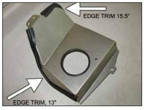
13. Install the rubber gasket trim on the heat shield as shown.
