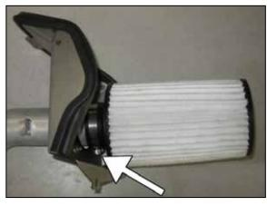
19. Orient the hose clamp as shown in the picture, and tighten.
