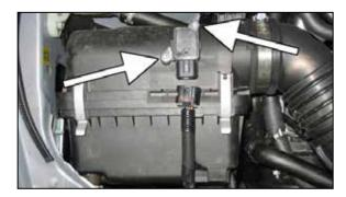
7. Remove the MAF sensor from the airbox by removing the two screws. Set the MAF sensor aside in a safe area for later use.
