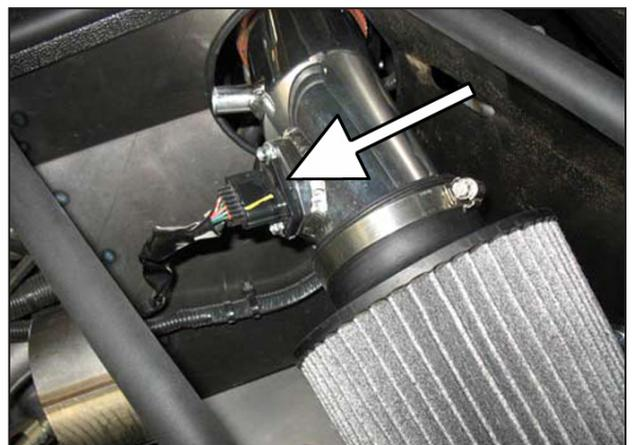
s. Plug in the MAF sensor harness connector to the MAF sensor
