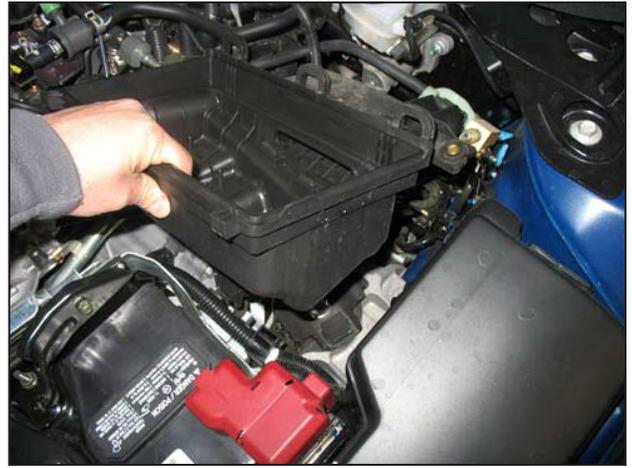
r. Remove the air box base by lifting upwards, this will require some effort because the base is secured in place with two rubber grommets on the bottom side.
