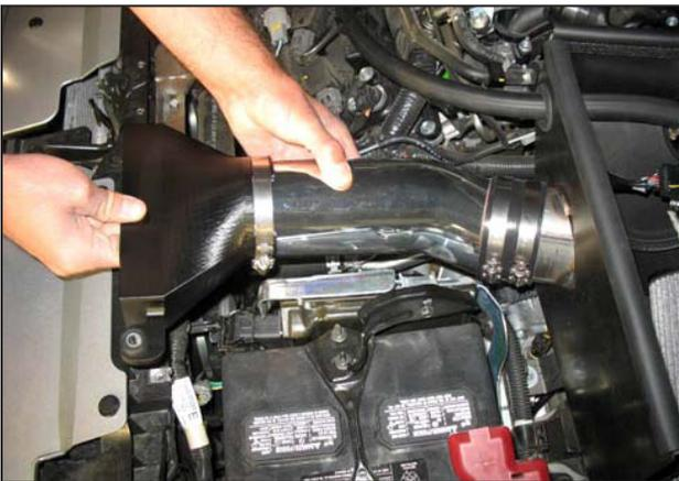
ab. Secure the air supply duct to the air supply scoop with a #9456 hose clamp. Install the assembly as shown.
