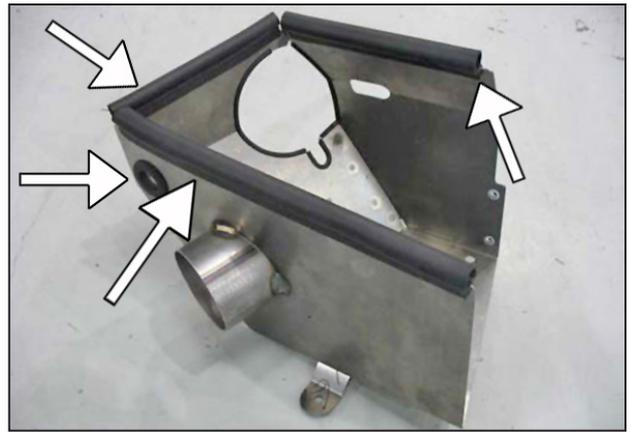
i. Install the edge trim onto the top edges of the heat shield and trim to fit. Install the rubber grommet in the heat shield hole as shown.
