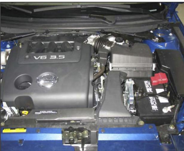
Factory air box system installed
