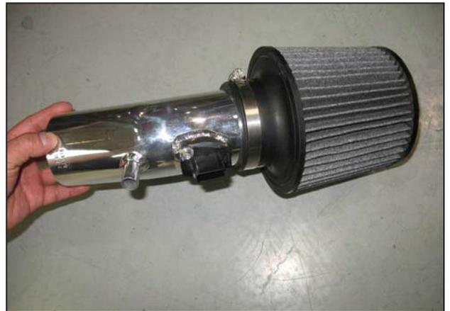
q. Remove the MAF sensor from the factory air box lid. Install the MAF sensor into the intake pipe with the factory screws. Install the air filter onto the intake pipe and secure it with a #9452 hose clamp.
