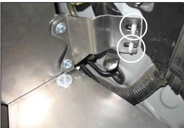
l. Remove the two nuts from the circled studs on the shock tower. Install the rear bracket as shown, use two M6 fender washers and M6-1 x 12mm hex head bolts to secure the bracket to the heat shield. Do not completely tighten the bolts.
