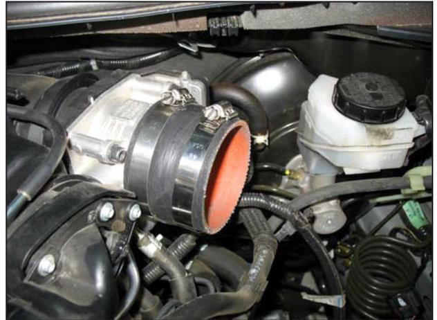
g. Install the 3.25" to 3.00" diameter hose adapter onto the throttle body. Secure the adapter in place with a #9452 hose clamp. Slide a #9448 hose clamp onto the smaller diameter side of the adapter hose.
