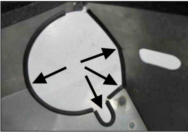
h. Line the edges on the heat shield with the supplied rubber edge trim.
