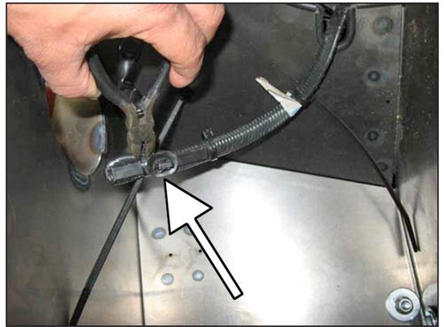
o. Cut the factory zip tie securing the wiring harness to the plastic push-in mounting tab.
