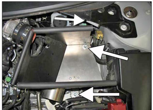
k. With the heat shield in place, install M6 fender washers and M6 nuts over each mounting stud. The black box mounted to the firewall near the heat shield may need to be adjusted for clearance. Carefully bend the black box's bracket towards the firewall to allow enough clearance.
