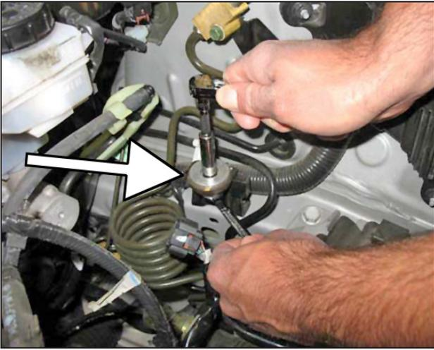
d. Install the cone shaped aluminum stand in the grommet. Secure the hardware from step 3c with a M6 serrated nut.
