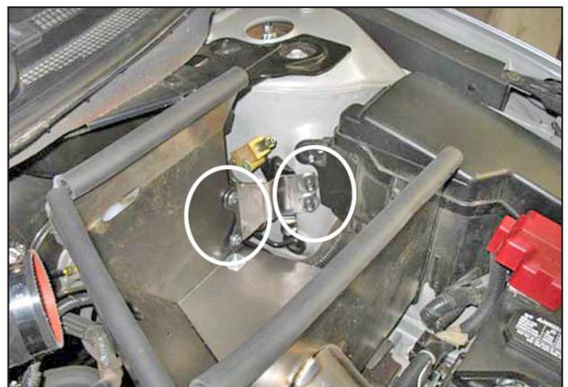
m. Place two M6 fender washers over the two shock tower studs. Reinstall the two nuts that were removed in the previous step. Completely tighten the two bolts and two nuts securing the bracket.
