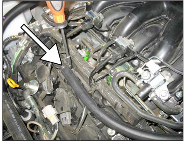
u. Connect the other end of the PCV hose to the port on the engine. Secure the PCV hose with a 1-1/16" hose clamp.
