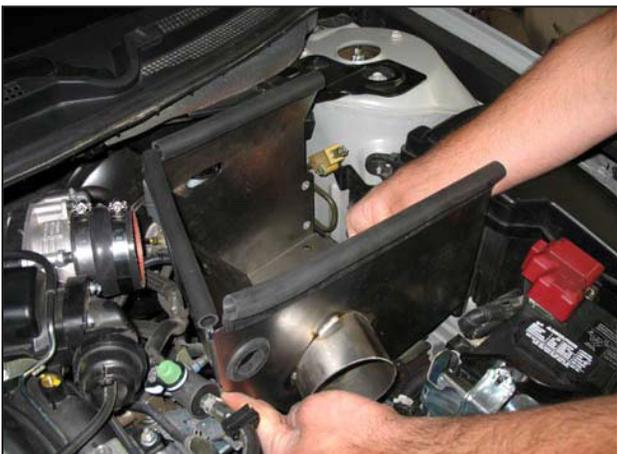
j. Install the heat shield in the vehicle, aligning the holes of the heat shield base with the aluminum mounts that were installed in steps 3d-3f.
