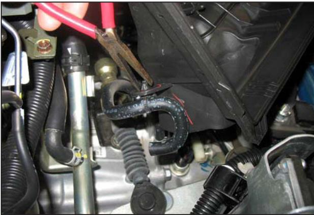
s. Remove the clip securing the rubber tube.
