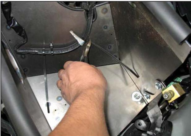
p. Route the MAF sensor wiring as shown and secure the wiring harness with the two zip ties. Trim the excess zip tie ends.
