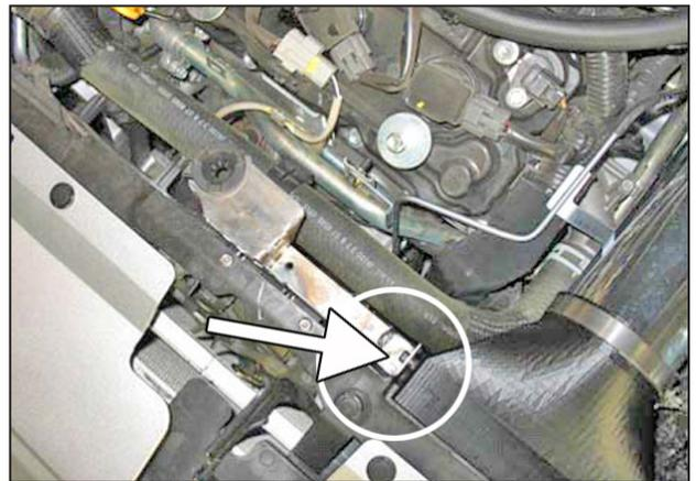
ac. Insert the nub of the air supply scoop into the hole of the bracket.
