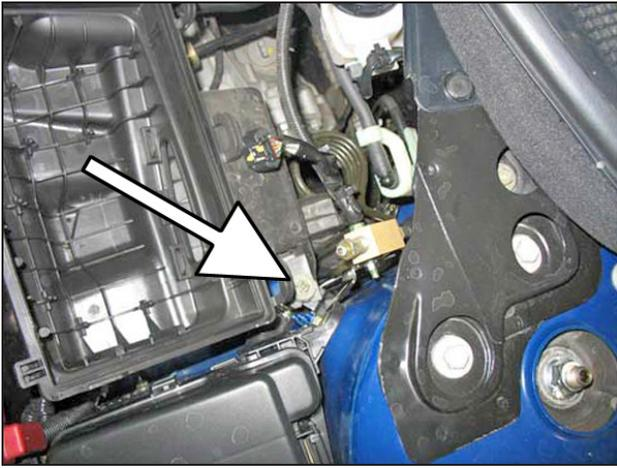
q. Remove the hex head screw securing the air box base.
