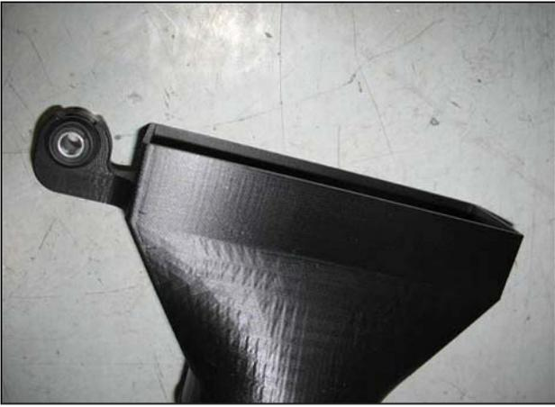
z. Install the rubber grommet and metal sleeve into the air inlet scoop as shown.
