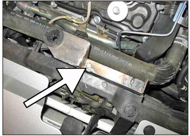
aa. Install the bracket with a M6-1x 12mm hex head bolt. Tighten the bolt enough to hold the bracket in place, but do not completely tighten.
