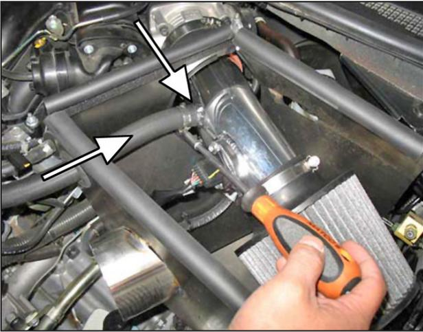
t. Insert the 5/8" I.D. PCV hose through the heat shield grommet and connect it to the intake pipe's nipple. Secure the PCV hose with a 1 1/16" hose clamp.
