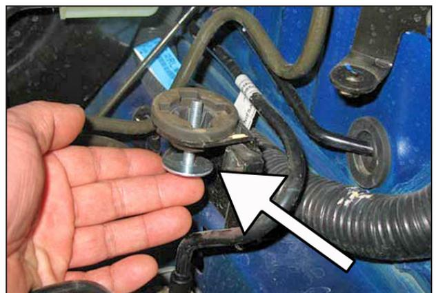
c. The hardware prepared in step 3b will slide through the factory grommets as shown. If the factory grommets are missing, check the bottom of the air box base or the engine bay as they may have fallen out when the air box was removed.
