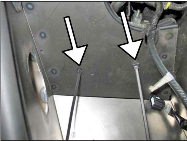
n. Install two push in zip ties on the inside wall of the heat shield. Route the MAF sensor wiring into the heat shield as shown.
