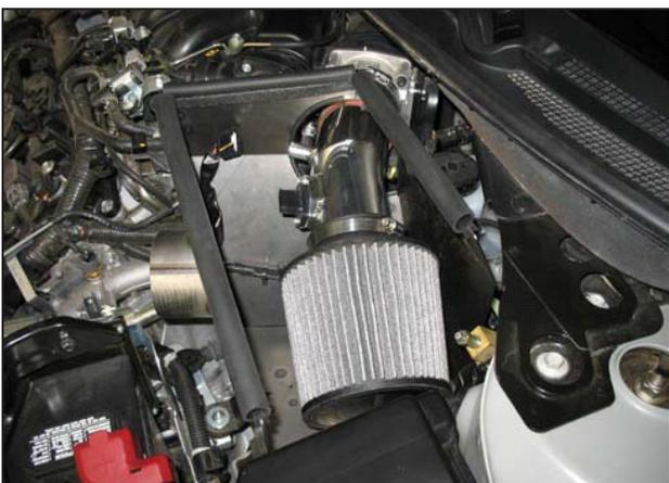
r. Install the intake pipe assembly as shown. Position for optimal clearance, ensuring that the assembly does not contact any surrounding parts. Secure the intake pipe to the coupler installed on the throttle body.
