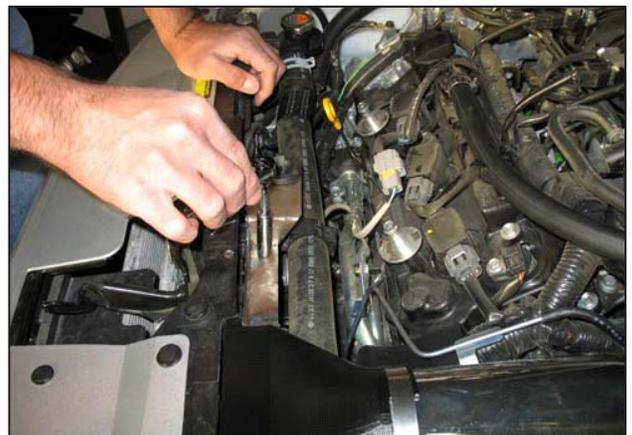
ae. Tighten the M6 hex head bolt securing the bracket.
