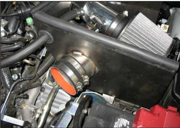
v. Install the 3.50" x 2" silicone coupler onto the heat shield inlet tube. Slide two #9456 hose clamps onto the silicone coupler.
