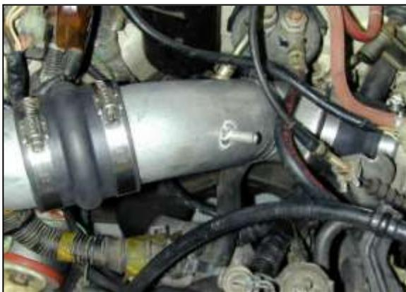
i. Install the upper inlet pipe as shown. First, attach the hump hose side of the inlet pipe onto the upper end of the lower inlet pipe. Then attach the upper end of the upper inlet pipe onto the throttle body.
