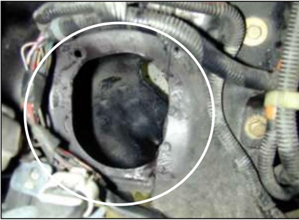
d. The factory hole that the inlet pipe passes through must be enlarged for clearance of the AEM® intake pipe. The use of a specialized power tool will be needed to cut through the inner fender so the AEM® intake pipe is able to clear the inner fender opening. A minimum of at least a 3.50" diameter is recommended. Ensure that any rough or sharp edges are smoothed and that the AEM® intake pipe is able to clear the opening without touching any part of the inner fender.
