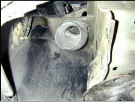
k. Ensure the lower inlet pipe clears the newly enlarged opening. Attach the air filter and secure to the inlet pipe with the provided hose clamp.
