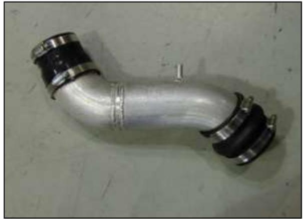
h. Assemble the upper inlet pipe as shown. On the throttle body side, attach the reducer coupler and hose clamps. On the nipple side, attach the hump hose and hose clamps. Do not completely tighten the hose clamps.
