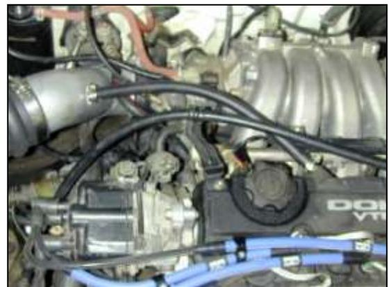
j. Attach the breather hose to the upper inlet pipe and the valve cover inlet. Secure each end of the breather hose with the provided hose clamps.
