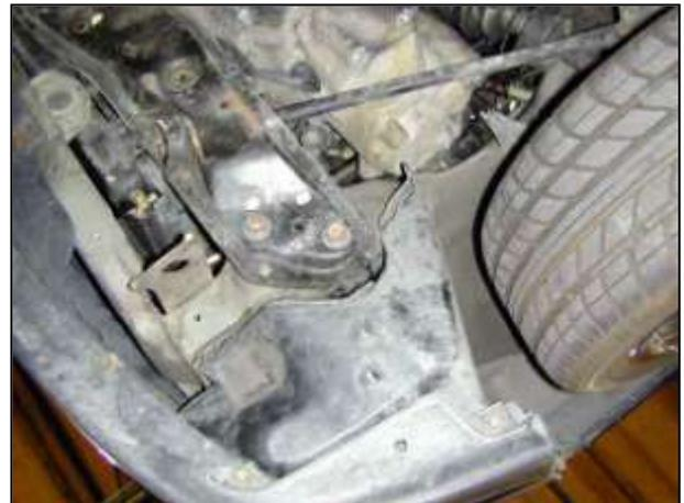
c. Remove the two tabs that secure the lower splash shield. Move the splash shield out of the way to gain access to the inner fender well where the factor resonator is located. Save the plastic tabs, they will be reused in a later step.
