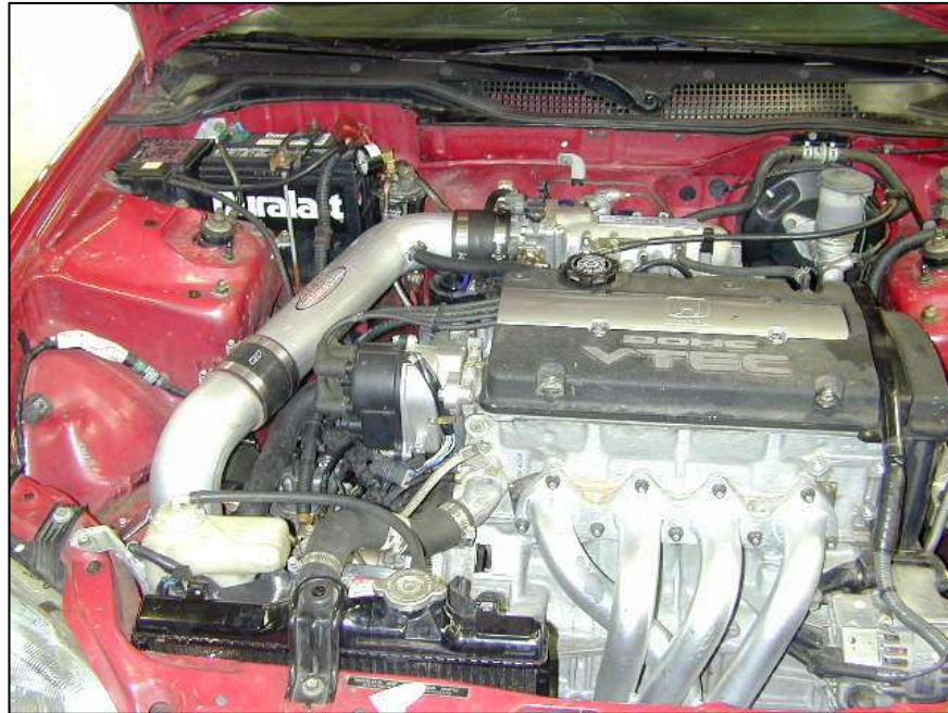
AEM® intake system installed
