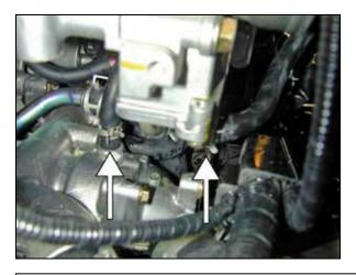
I. Another view of tubing loom routing. Use pliers to slide the spring clamps over the breather and coolant hoses. A flat-head screwdriver may be needed to pry the hoses off the coolant line nipples.
