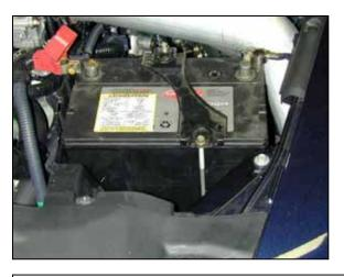
k. Reinstall the plastic battery under-tray, the battery, and the battery tie down bracket. Do not install the plastic battery cover. Check for proper clearance between the battery and the intake pipe. Use the supplied zip-ties to make sure no wires are in contact with the intake system.
