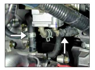
k. CAUTION: Ensure the engine is completely cool before removing the coolant hose, or hot coolant will escape from the cooling system and cause injury or damage. Be sure to capture any lost coolant in a clean container.
