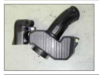
q. Remove the two bolts securing the resonator box to the frame. Remove the resonator box.
