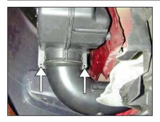
n. Removal of the stock intake resonator requires drilling. Start by drilling the two aluminum rivets shown.
