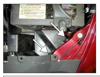
b. Remove plastic shrouding covering the battery. Remove the plastic air scoop in front of the battery by pulling out the two retaining clips and lifting scoop straight out.
