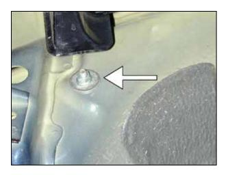
e. Secure the rubber mount using the supplied washer and nylok nut.
