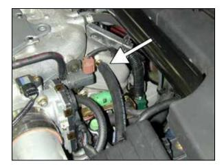
j. Install the supplied  $\frac{1}{2}$ " breather hose between the intake pipe and the valve cover. Secure with provided 1" hose clamps.
