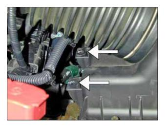
f. Remove the plastic clips holding the wiring harness to the throttle body side of the air filter housing.
