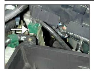
h. Remove wire clamp from the lower air box bracket.
