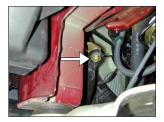
o. Remove the bolt securing the inlet tube to the frame. This can be reached through the wheel well.
