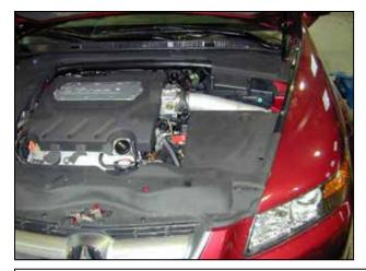
AEM<sup>®</sup> intake system installed
