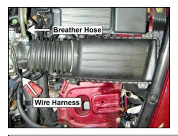
e. Loosen the hose clamp on the throttle body and unhook the wiring harness. Remove the stock breather hose from the inlet tube.
