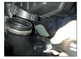
p. Using either a large screwdriver or a pry bar, pry the inlet air tube from the resonator box. Remove the inlet air tube.
