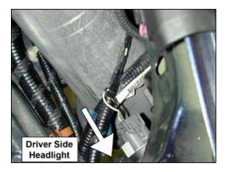
f. Install the AEM<sup>®</sup> intake pipe by routing the air filter end of the pipe through the opening in the engine bay between the battery location and the fender. Use rags to prevent scratches to the pipe.
