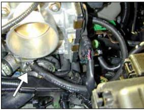
b. Install the provided 5/16" hose where the factory coolant line was removed. Use the supplied 3/4" hose clamps to secure the hose. NOTE: Replace any coolant recovered during hose removal by replenishing the recovery tank.
