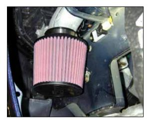
i. Install the AEM<sup>®</sup> air filter onto the end of the intake tube. Push the air filter over the intake pipe until the stop in the air filter is reached. Then install one hose clamp and secure the air filter onto the intake pipe. Once fitment is checked, tighten the hose clamp.
