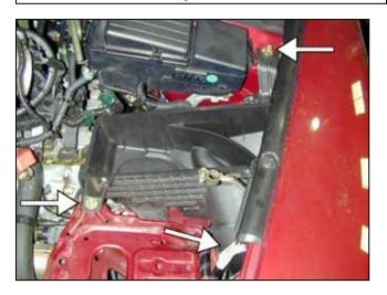
i. Remove the two bolts securing the lower air filter housing and remove housing. Pull up and remove the rubber sleeve connecting the air filter housing to the resonator below.
