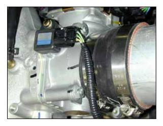
g. Install the silicone coupler attached to the  $\text{AEM}^{\circledast}$  intake pipe over the throttle body.
