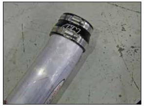
c. Check to see that the inside of the AEM<sup>®</sup> inlet pipe and air filter are clean and free from any foreign objects and/or obstructions. Install the 3"-3.25" silicone reducer over the throttle body end of the intake pipe using the 3" hose clamps.
