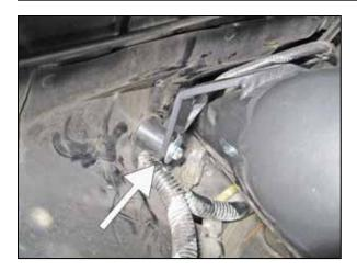
h. Guide the bracket on the intake pipe over the stud on the rubber mount. Once aligned, install the supplied washer and nylock nut onto the stud.
