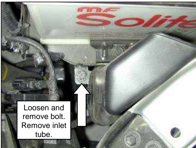
e. Loosen and remove mounting bolts to the fuse box to remove air tube connector. Reinstall mounting bolts for the fuse box.
