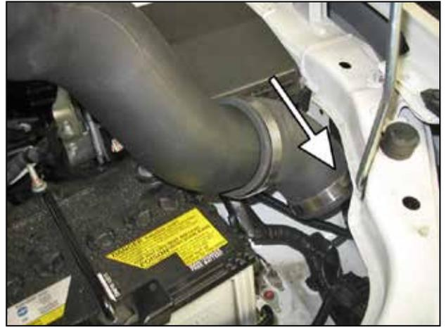
o. Route the intake tube down through the wheel well hole as shown.
