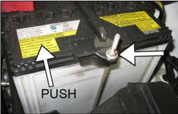
b. Remove the factory j-hook on the front side of the battery tie down. Push battery towards the back of the vehicle.
