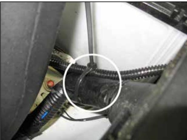
v. Secure the MAF sensor wire harness in place with a zip tie as shown.
