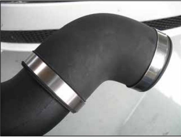
n. Attach the 90° elbow onto the upper intake pipe (side opposite of the nipple). Slide the provided hose clamps onto each end of the 90° elbow.
