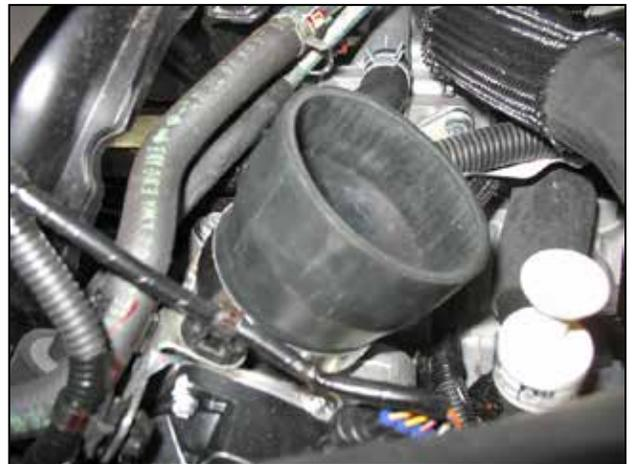
m. Place the coupler (5-253-54) onto the throttle body and secure it in place with a #40 hose clamp.
