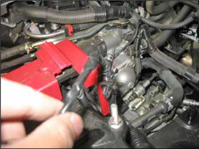
j. Wrap the remaining section of the wire harness with electrical tape.
