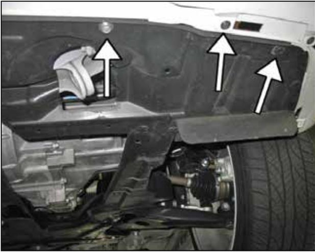
k. Raise the front of the vehicle with a jack. Refer to your owner's manual for proper jack and jack stand placement to properly support vehicle. Support your vehicle using properly rated jack stands before wheel removal or while working under the vehicle. **NEVER WORK UNDER A VEHICLE WITHOUT USING JACK STANDS.** Remove the plastic trim underneath the front of the vehicle on the driver side.
