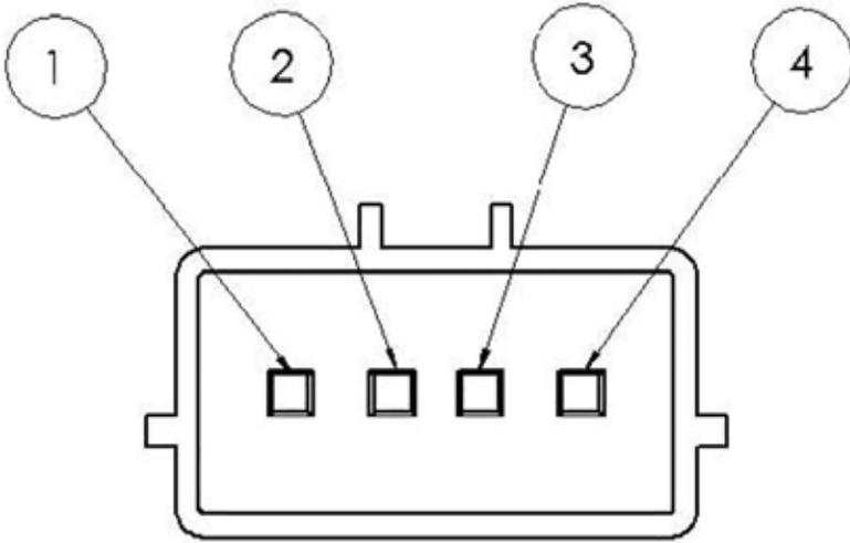
NOTE: PIN 4 on the female MAF sensor plug corresponds to the flow of the MAF sensor.
