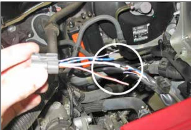
d. Locate the MAF sensor wire harness connector, measure 2 inches from the back of the connector and cut the four wires.
