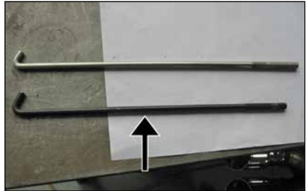
c. Replace the factory j-hook with the shorter j-hook that is supplied with installation kit.
