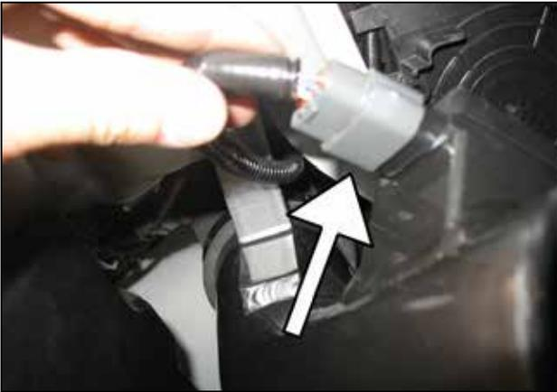
t. Plug the MAF sensor connector into the MAF sensor.
