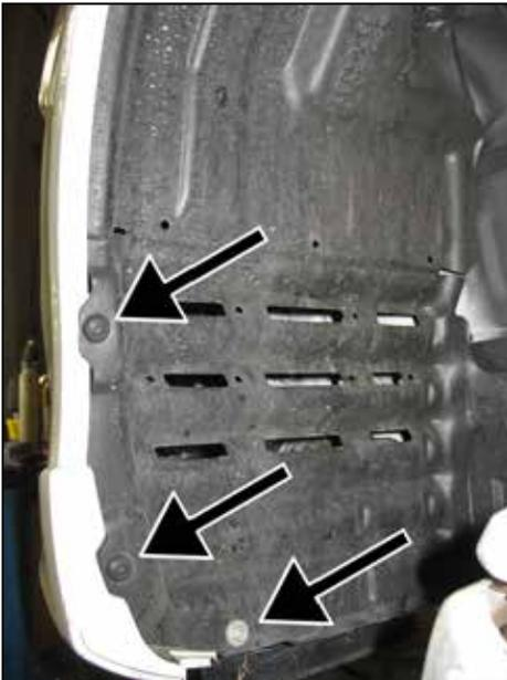
m. Remove the driver side fender well liner, it is secured to the wheel well with plastic clips and a 10mm hex bolt.
