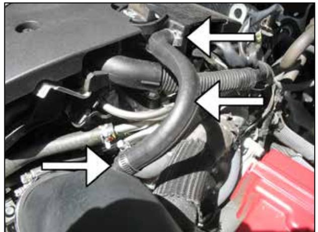
w. Attach the provided PCV hose onto the crankcase inlet and intake pipe nipple. Secure each end with a provided hose clamp.
