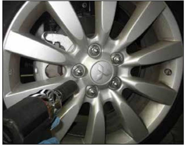
l. Remove the front drivers side wheel with a 21mm socket.
