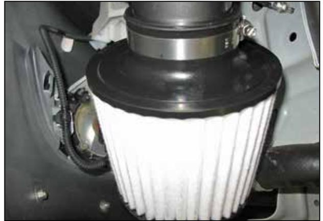
u. Install the air filter (21-2027DK) onto the lower end of the lower intake pipe (2-6792). Secure the air filter onto the intake pipe with a provided #44 hose clamp.
