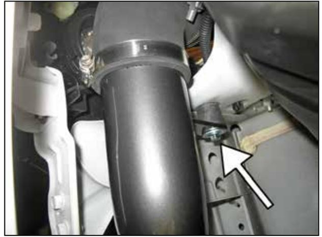
s. Feed the lower intake pipe through the bottom side of the fender well. Align the intake pipe's bracket onto the rubber mount and loosely secure in place with the provided 6mm washer and the 6mm nut.
