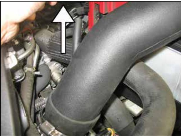
p. Insert the upper intake tube (9-6791) into the throttle body coupler. Position the intake tube so the nipple is pointing upward as shown. Use a provided hose clamp to loosely secure in place.
