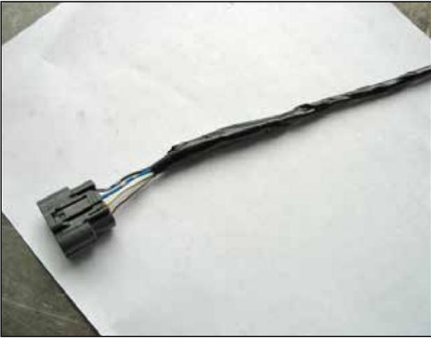
h. Wrap the wires together with electrical tape.
