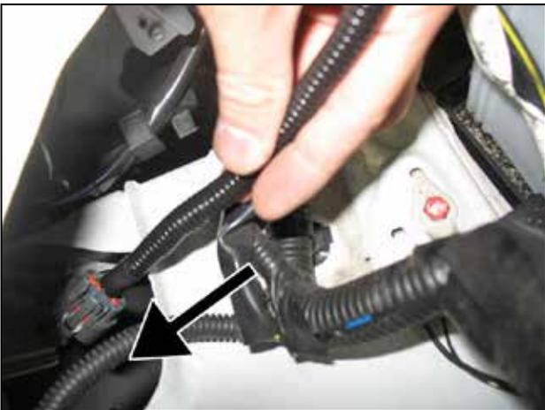
l. Route the MAF sensor harness down into the wheel well area.
