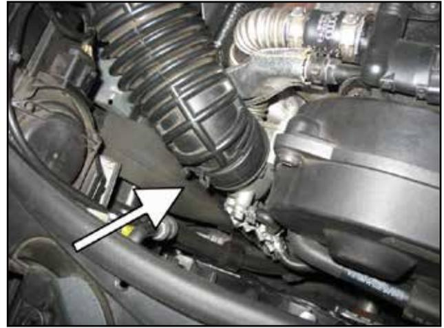
l. This is a good location for the hose clamp to be located once you have moved it away from the rubber inlet tube and turbo inlet joint.
