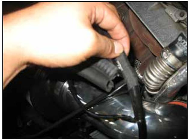
y. Secure the three metal clips located on the MAF harness wire to the heat shield. There are three holes located on the sides near the top.
