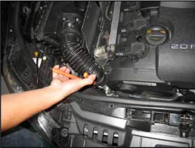
k. **WARNING!** (The hose clamp securing the inlet tube to the turbo inlet is under high compression). Carefully use a pair of pliers to decompress the hose clamp securing the rubber inlet tube to the turbo inlet. Move the clamp up toward you and let it compress on a higher location on the rubber inlet tube.
