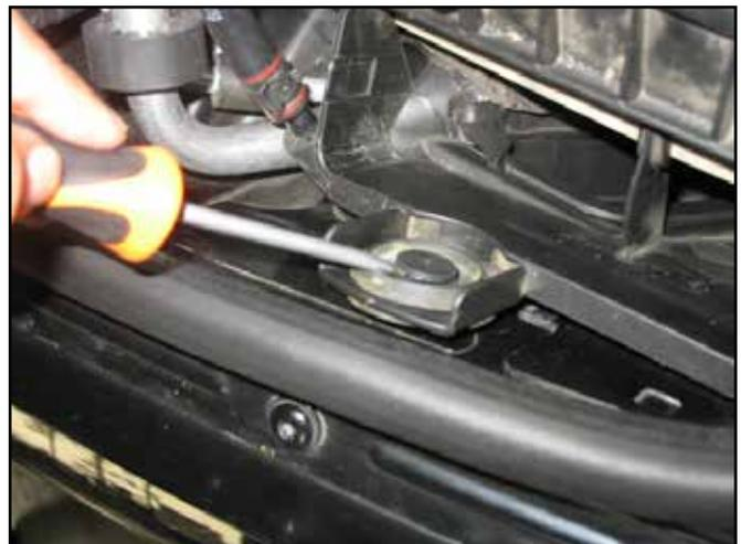
j. Remove the plastic rivet securing the air box to the passenger side fender by using a flat screwdriver to pry it off.
