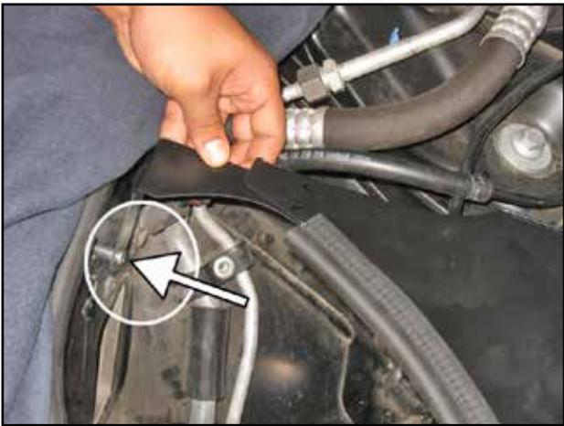
p. Align the wellnut with the hole exposed in step 2p and put it through the hole. Then align the two holes on the other end of the bracket with the two holes on the heat shield.
