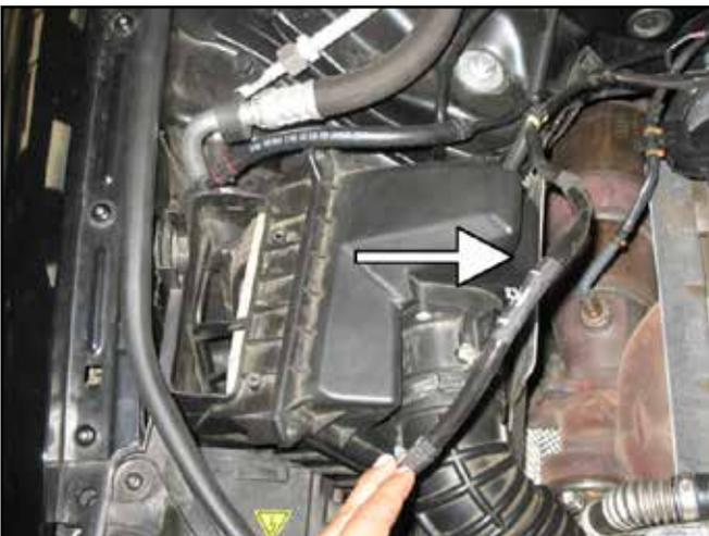
i. Pull the MAF wire harness carefully away from the stock air box.
