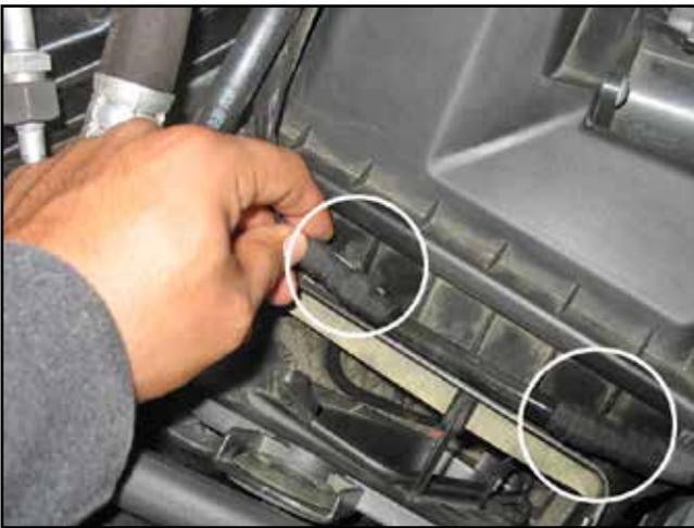
g. Disconnect the metal clips securing the MAF harness to the stock air box. There are 3 clips, 2 are shown in this picture and the third one is in the next step.
