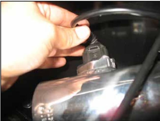
v. Plug the MAF sensor harness into the MAF sensor.
