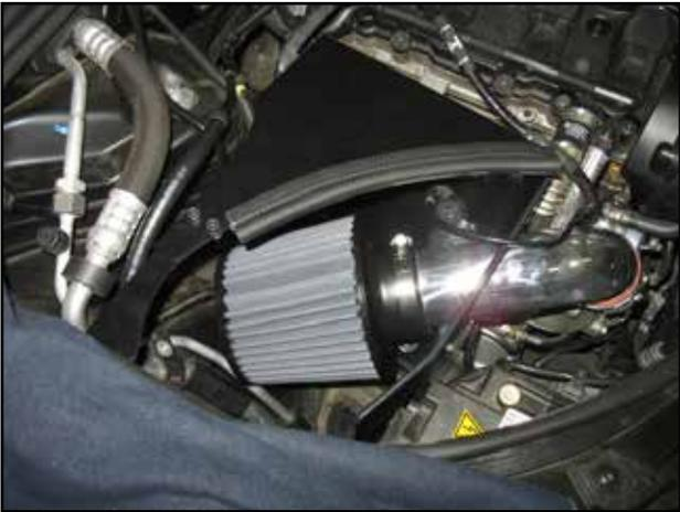
x. Install the Dryflow™ air filter and secure it to the end of the inlet pipe with the #48 hose clamp.
