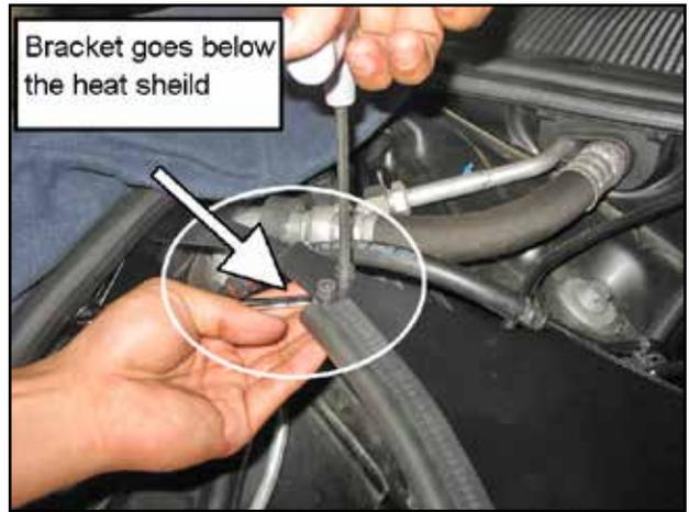
q. Align the M6- 1.0X14 socket bolts with the two holes on the heat shield and bracket. Secure the M6 bolts with the supplied M6 nuts.
