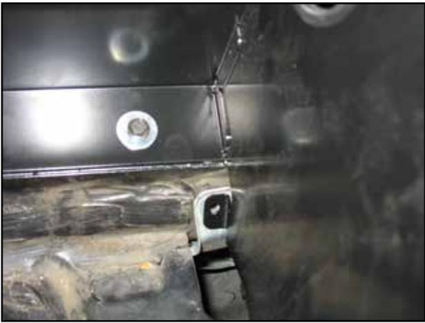
j. Install the heat shield in the vehicle by aligning the two heat shield mounts with the stock grommets. Push the mounts into the grommets to secure.
