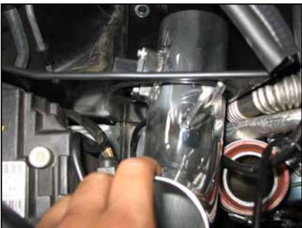
t. Insert the inlet pipe into the heat shield as shown with the bracket facing up and MAF sensor facing toward the passenger side of the car.
