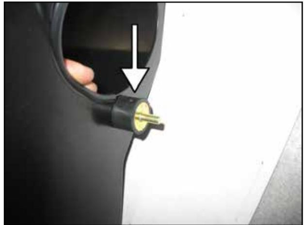
g. Install the shorter piece of rubber edge trim on the pipe inlet hole. Start right next to the rubber mount and work your way around.
