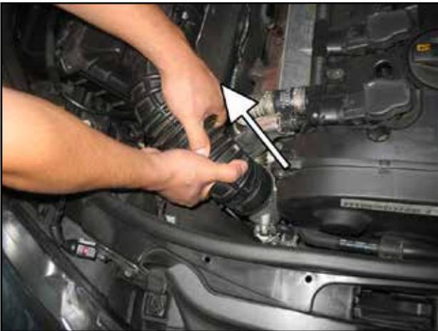
m. Firmly grip the rubber inlet using two hands to pull the rubber inlet away from the turbo inlet.
