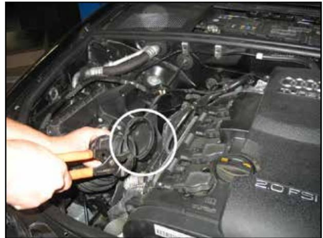
n. Carefully decompress the hose clamp again and remove it from the rubber inlet tube.
