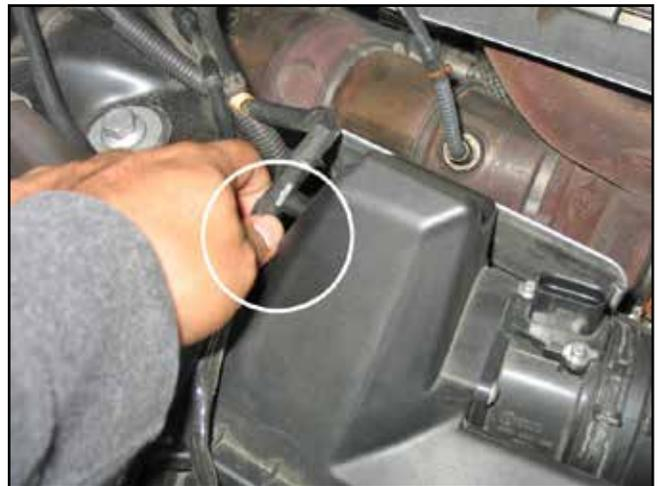
h. The third clip is located on the firewall side of the air box.
