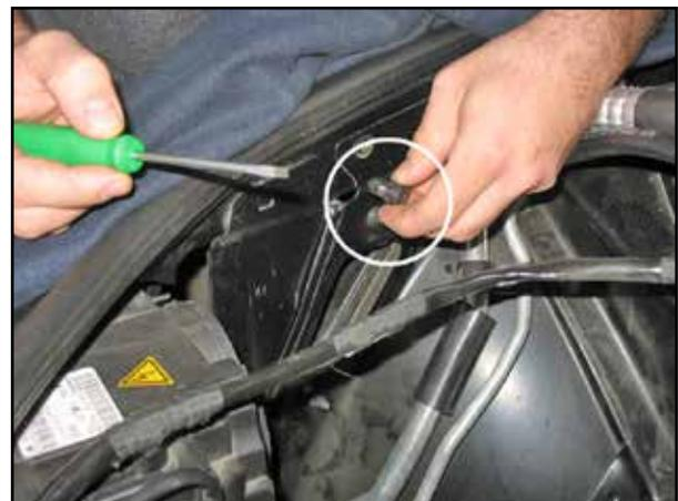
p. Using a small flat screwdriver, remove the plastic receiver off of the plastic rivet removed in step 2j.
