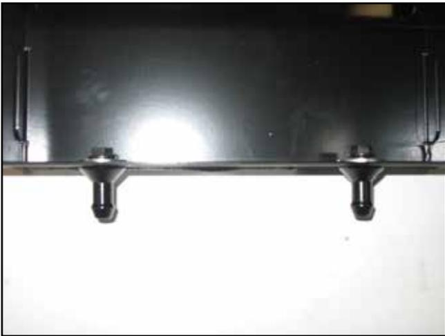
d. Insert the two M6X12 bolts and washers into the two holes on the bottom of the heat shield. Screw the heat shield mounts onto the bolts holding the heat shield mount with your hand. Then tighten the bolts with a 10mm wrench or socket.
