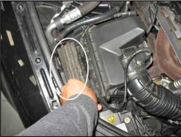
e. Remove the prefilter from the stock air box. This may still be in the fresh air duct.
