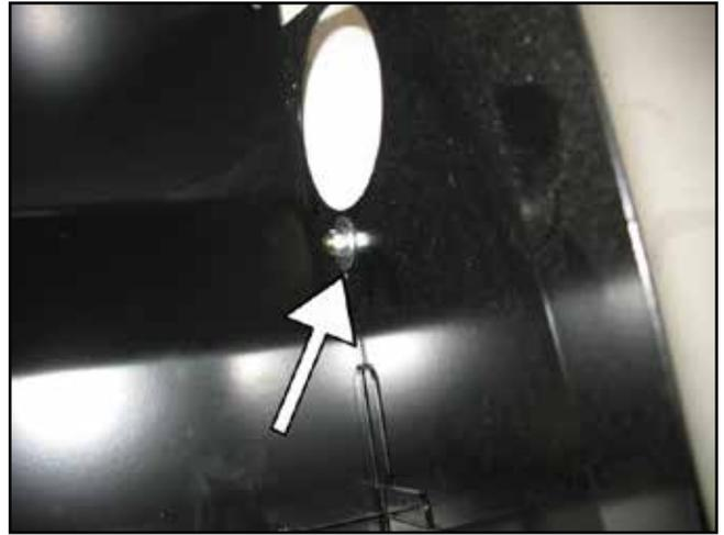
e. Insert the rubber mount into the hole located just below the pipe inlet hole and secure the rubber mount with a washer and an M6 nut.
