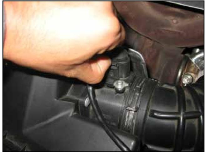
f. Disconnect the mass airflow (MAF) sensor harness from the MAF sensor.
