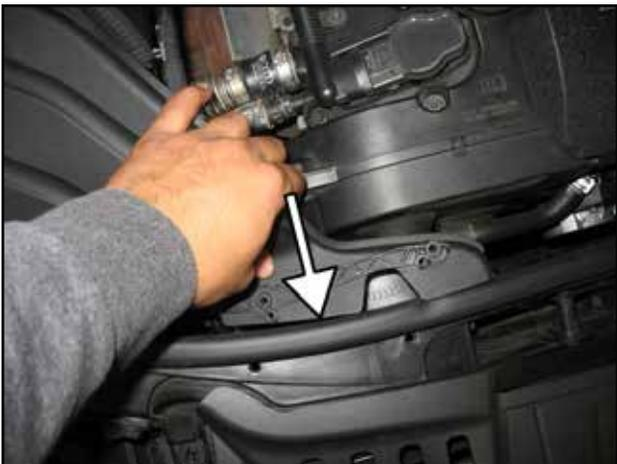
z. Slide the stock fresh air duct back into the fresh air scoop.
