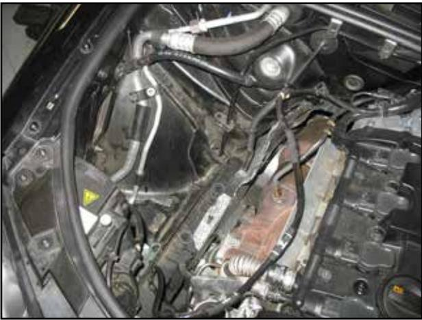
s. Factory air box system removed from the vehicle.
