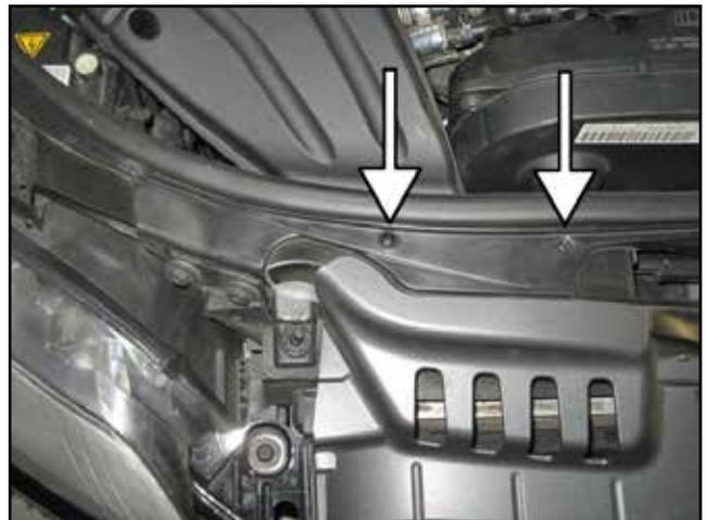
aa. Slide the plastic arm located on the fresh air duct into the grommet installed in step 3m.
