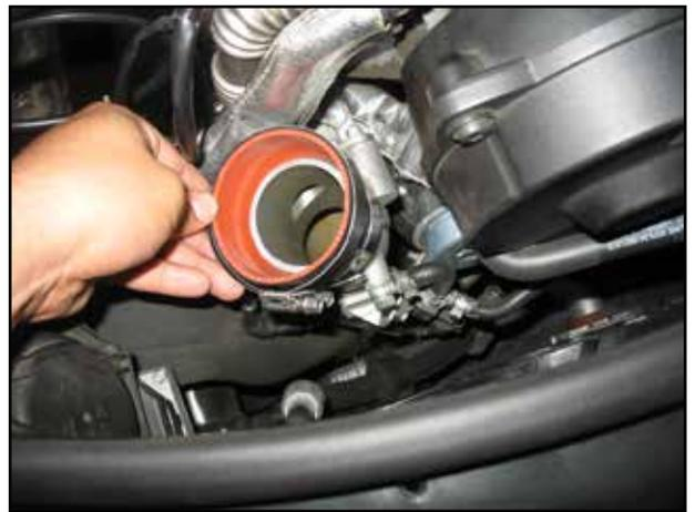
s. Put the transition coupler on the turbo inlet. The #40 hose clamp goes on the turbo inlet side and the #44 hose clamp goes on the inlet pipe side.
