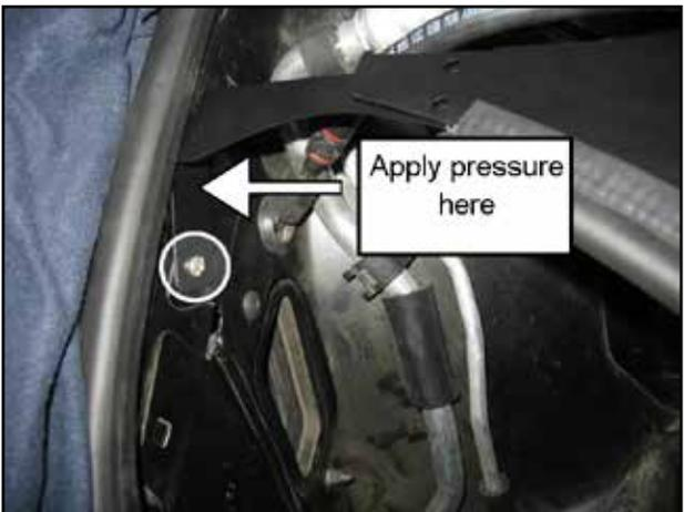
r. Apply pressure with your hand on the bracket toward the passenger side fender and tighten the machine screw with a phillips head screwdriver until it feels secure.
