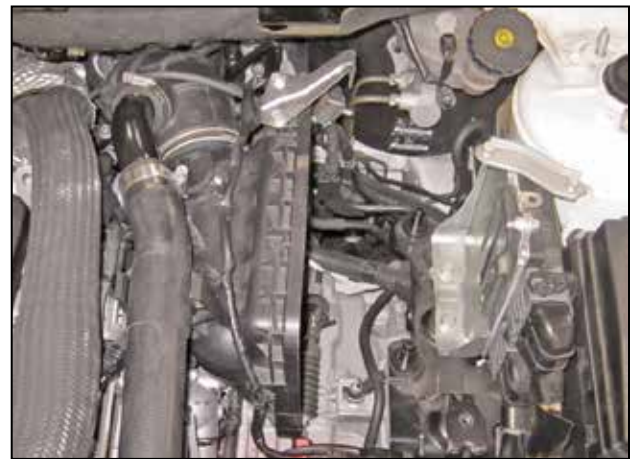
h. Remove the right half of the air box assembly by sliding it up and off of the two mounting studs.
