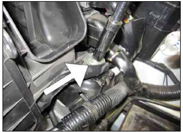
f. Remove the washer and mounting bolt retaining the front of the stock air box.
