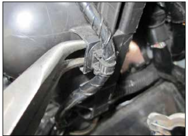
j. Unfasten the 3 plastic clips retaining the MAF wiring harness to the left half of the air box with a pair of pliers.
