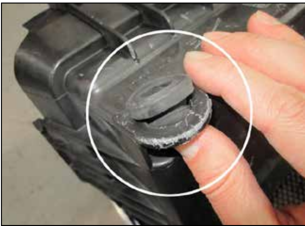
i. Remove the 2 rubber isolator grommets from the bottom of the right half of the air box assembly. These will be reused during the installation of the AEM® intake system.
