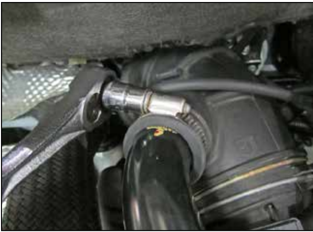
e. Unfasten the hose clamp securing the recirculation pipe to the intake tube, then disconnect the pipe from the intake tube. If needed, use a metal pick to break the seal between the pipe and the rubber bypass port.
