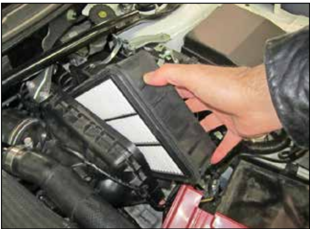
g. Unfasten the 2 air box retaining clips and remove the panel air filter from the air box assembly.
