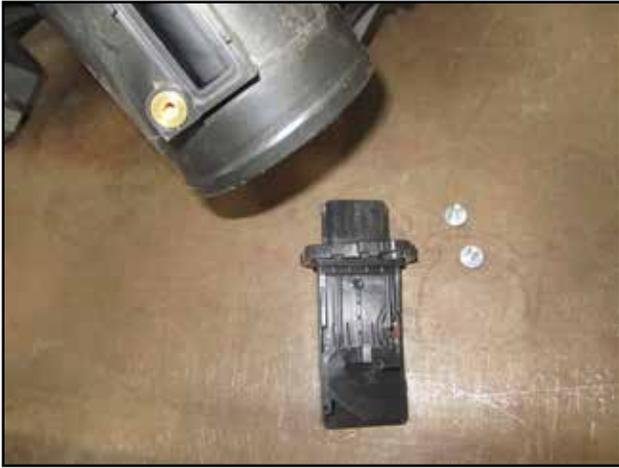
k. Remove MAF sensor from the air box.
