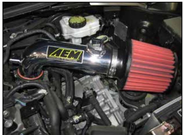
k. Install the intake pipe (1) into the throttle body coupler and align the bracket in place on rubber mount.
