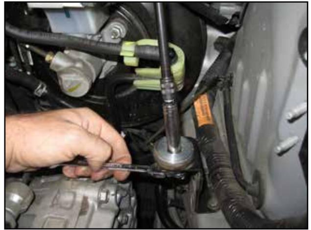
g. Once properly assembled, tighten the nuts and bolts to secure the adapter assembly.
