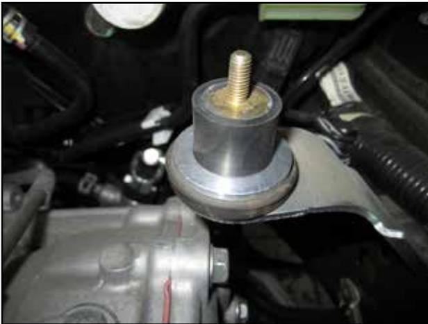
h. Install rubber mount (14) onto the (12) bolt.
