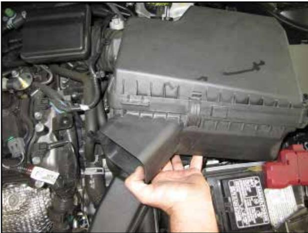
g. Lift up on the bottom of the airbox to disengage but do not remove from the engine bay.
