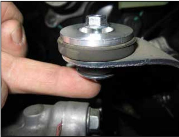
f. Slide bolt (12) and washer (10) through the rubber grommet and use the M6 (11) nut to keep the assembly together.
