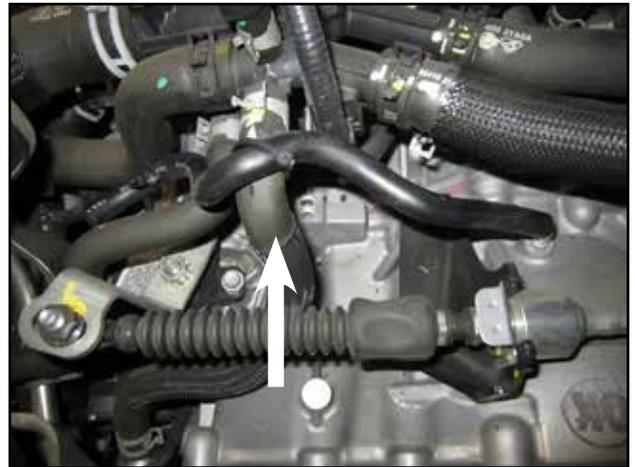
i. Use the provided zip tie (15) to attach the transmission vent tube to the coolant line as shown.
