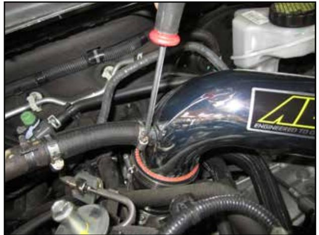
o. Tighten the provided (7) vent hose and (8) hose clamp to the intake tube.
