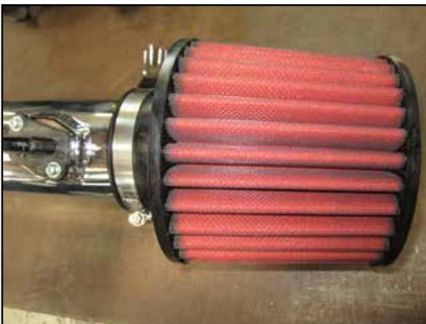
j. Mount the AEM air filter (2) onto the intake tube (1) using the (6) hose clamp. Tighten Hose clamp.
