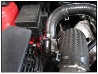
a. Remove the recirculation hose on the OEM intake pipe.
