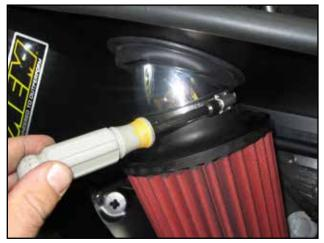
t. Align the filter and tube then tighten hose clamps (F) and (I).
