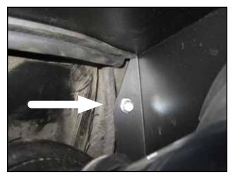
m. Install the M6 Bolt (M) and washer (Q) onto the bottom of the heat shield. Do not fully tighten at this time.
