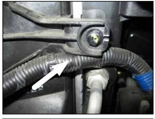
Remove the bolt on the fan shroud.
