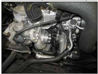
Remove the intake tube from the engine bay.
