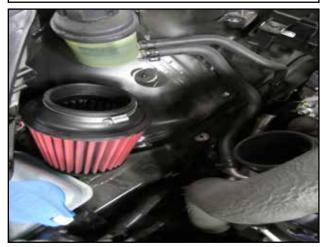
h. Place filter (E) and hose clamp (F) in the engine bay as shown.
