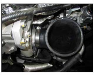
d. Install the coupler (H) onto the Turbo inlet using the provided hose clamps (G) and (I).
