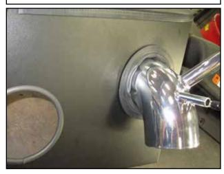
Place intake tube (B) through the hole in the heat shield (O) as shown.
