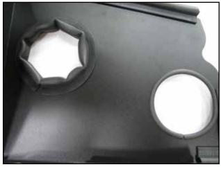
g. Install edge trim (C) and (D) on the two large holes as shown.
