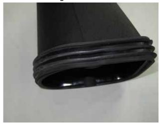
Install the OEM rubber gasket on the AEM scoop adapter (A)
