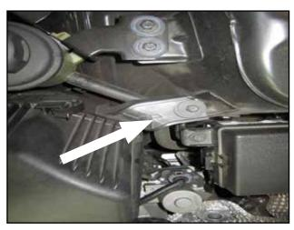
d. Remove the M6 bolt holding the airbox in place.
