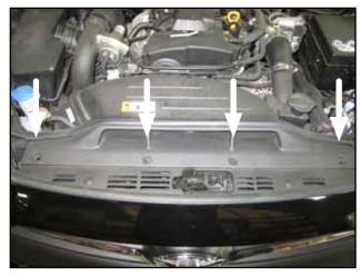
e. Remove the four clips securing the scoop and set scoop aside for use with the AEM intake system.
