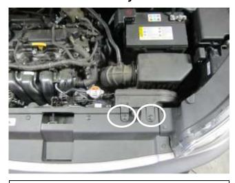
a. Remove the engine cover by pulling it up and out of the vehicle. Remove the two plastic clips (circled) and remove the stock scoop.
