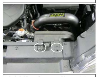
j. Re-install the engine cover and the two plastic clips holding the stock scoop in place.
