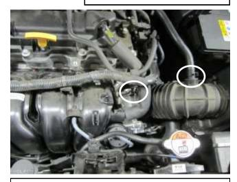
b. Loosen the hose clamp at the throttle body, then release the pressure on the spring clamp and disconnect the valve cover breather hose from the stock intake tube.
