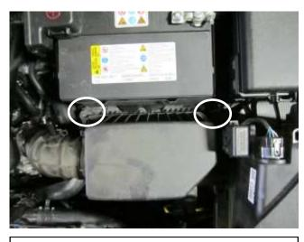
c. Remove the two bolts that secure the stock air box to the vehicle.
