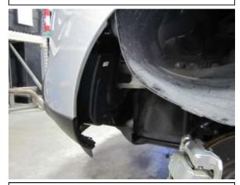
h. Remove the three bolts that secure the resonator to the vehicle. \*See step g for location of the bolts.
