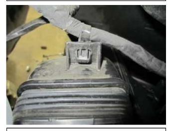
i. Squeeze the clips together while pulling away from the clip retainer. Remove the resonator from the vehicle.
