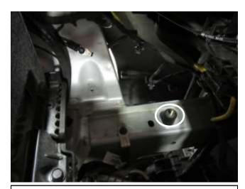
b. Install the rubber mount (1228599) onto the vehicle in the location shown.
