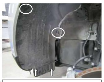
f. Remove the four plastic clips securing the inner wheel well liner. Two of the plastic clips are on the bottom of the liner.
