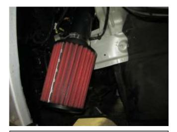
e. Install the AEM filter (21-2027DK) and hose clamp (9448) onto the AEM intake tube through the wheel well and tighten the hose clamp at this time.
