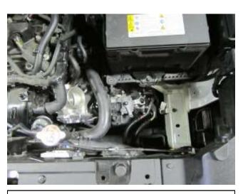
d. Remove the stock air intake system from the vehicle. **Note:** Do not discard any of your stock intake components.
