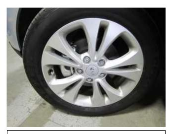
e. Raise the drivers side wheel and secure the vehicle with proper safety equipment. Remove the drivers side front wheel.
