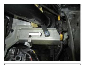
f. After the filter is installed, make sure tube alignment and filter clearance are good before tighten the two hose clamps at the throttle body. Then, tighten the nut securing the bracket to the rubber mount.
