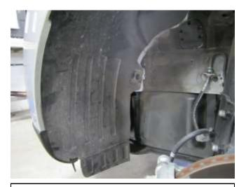
h. Re-install the four plastic clips securing the inner wheel well liner that were remove in step 2f.
