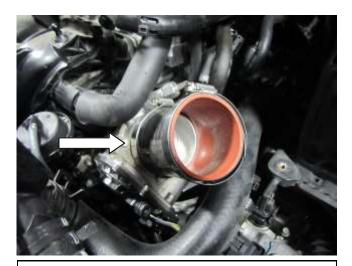
a. Install the supplied hose (5-277) and hose clamps (9444) onto the throttle body. The hose is angled, so make sure that the hose is angled up.
