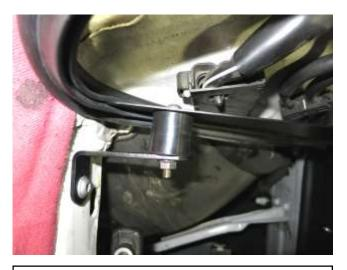
c. Install the included bracket and soft-mount using the factory bolt as shown.
