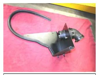
a. Assemble the lower heat shield components as shown according to the graphic on page 2 of this document leaving the edge trim loose at the upper left corner.
