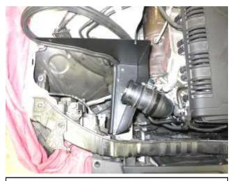
b. Lower the assembly into the vehicle being careful to orient the hose clamps such that they can be accessed by tools to be tightened.
