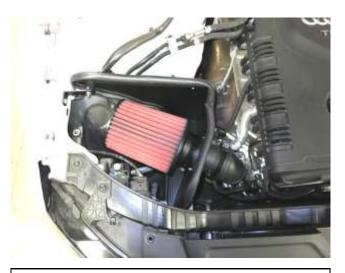
d. Install the air filter. If an open element kit is desired, the edge trim can be installed around the lower heat shield edge as shown above. For better performance via colder air supply, add the upper heat shield/duct and hardware according the graphic on page 2 of this document continuing the edge trim along the edge of the upper heat shield as shown in step f (next page).
