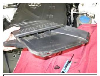
d. Remove the pre-filter from the opposite end of the duct assembly as shown.
