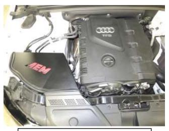
f. Finished installation of AEM Intake System.
