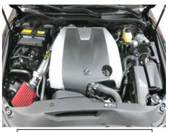
p. Finished installation of AEM Intake System.
