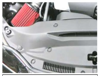
I. Reinstall the plastic fascia from step 2b and along with the 8 fastening clips.
