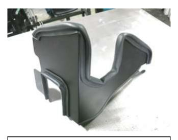
d. Install the 3 provided edge trim pieces onto the AEM heat shield as shown.
