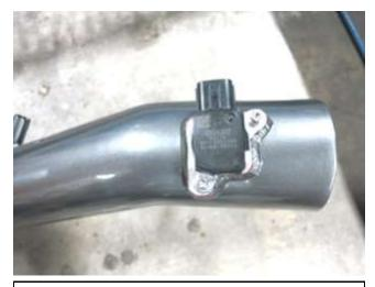
a. Reinstall the MAF sensor into the AEM tube and fasten using the provided bolts(07733).
