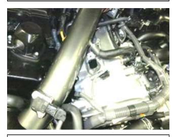
i. Reconnect the PCV hose to the AEM tube provision and the harness to the MAF sensor.
