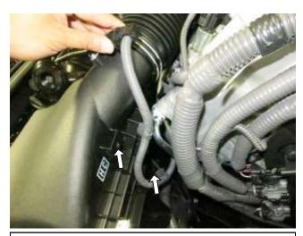
d. Disconnect the two tree mount clips securing the MAF harness to the stock airbox. Unclip the harness from the MAF sensor as shown.
