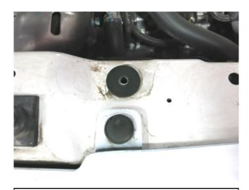
d. Place the provided rubber washer on the front core support over the mounting hole.
