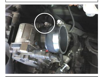
i. Install the provided coupler and hose clamps onto the throttle body. Tighten the hose clamp circled at this time.
