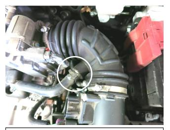
b. Loosen the spring clamp and remove the vent tube from the stock intake tube. The spring clamp will be reused in step 3k.
