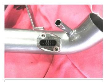
a. Install the Mass Air Flow sensor into the AEM intake tube that was removed in step 2h. with the provided hardware.
