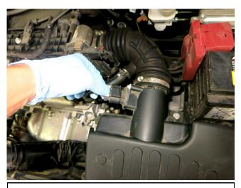
a. Disconnect the mass air sensor connecter by sliding the gray locking tab and depressing the tab.
