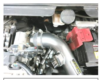
j. Install the AEM intake tube into the coupler.
