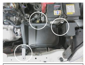
e. Place the heat shield into the vehicle aligning all three mounting locations as shown.
