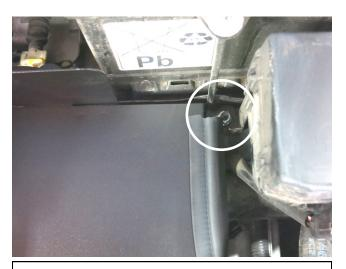
h. Install the nut that was removed in step 2g. to secure the heat shield in front of the battery tray.
