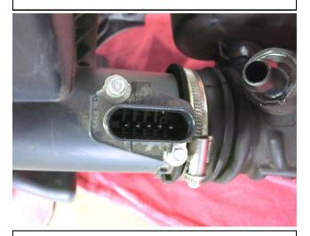
h. Remove the two bolts securing the Mass Air Flow sensor from the stock intake. The sensor will be reinstalled in step 3a. **NOTE: DO NOT DISCARD ANY OF YOUR STOCK EQUIPMENT.**
