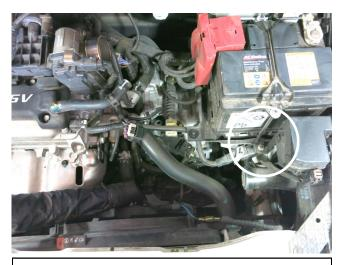
g. Remove the M6 nut in front of the battery as circled. This nut will be reused in step 3h.
