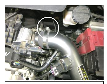
n. Tighten the other hose clamp at the throttle body at this time.
