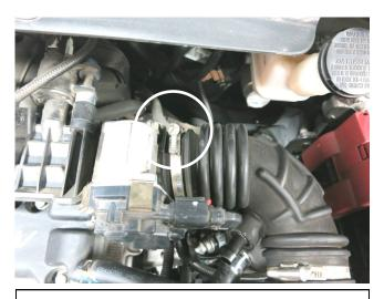
e. Loosen the hose clamp at the throttle body and disconnect the stock intake from the throttle body.
