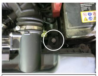
d. Remove the single bolt holding the rear of the stock air box to the vehicle.
