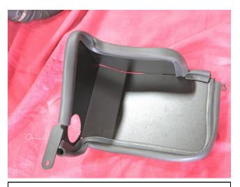
b. Install the provided edge trim onto the heat shield. Trimming of the edge trim may be necessary.
