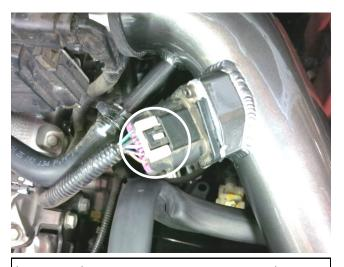
l. Connect the mass air sensor connecter onto the sensor and slide the gray tab to lock it into place.
