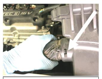
f. Push in the clips on the stock air box to remove the fresh air tube from the lower air box. Then remove the stock intake system from the vehicle.
