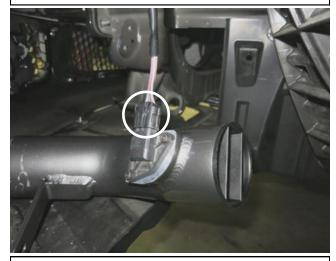
j. Plug the MAF extension harness into the MAF sensor.
