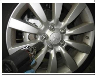
o. Re-install the wheel that was removed in step 2k. onto the vehicle and torque the lug nuts to the manufactures torque specifications.
