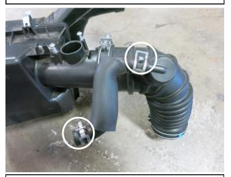
n. Remove the two springs clamps circled. These will be reused in step 3m.
