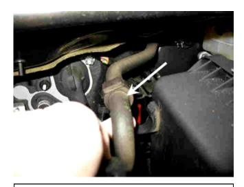
d. Unclip the hose from the air box retainer.
