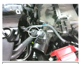
f. Unplug the electrical connector from the mass air sensor.
