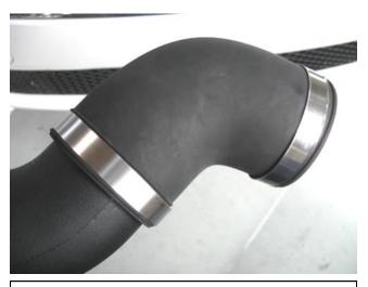
f. Attach the 90° elbow coupler onto the upper intake tube (side opposite of the nipple). Slide the supplied hose clamps onto each end of the coupler.
