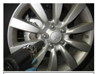
k. Remove the front drivers side wheel with a 21mm socket. This will be re-installed in step 3o.
