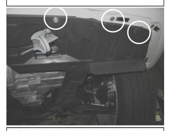
p. Re-install the plastic trim with hardware that was removed in step 2j. Remove the jack stands and lower the vehicle back onto the ground.
