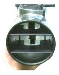
e. Install the supplied MAF insert into the AEM intake tube as shown. Note: Apply a few drops of super glue to the lip of the MAF insert to secure it in position.
