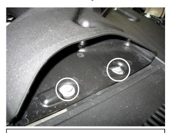
a. Remove the two Phillips fasteners that secure the fresh air duct to the core support and remove the fresh air duct com the engine compartment.
