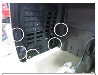
I. Remove the driver side fender well liner, it is secured to the wheel well with plastic clips and a 10mm hex bolt. This will be re-installed in step 3n.
