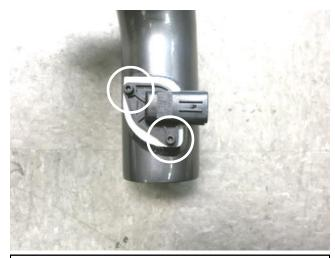
d. Install the MAF that was removed in step 2m. into the AEM intake tube and secure with the supplied hardware.
