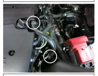
m. Attach the supplied PCV hose onto the crankcase inlet and intake pipe nipple. Secure each end with the spring factory clamps removed in step 2n.
