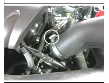
h. Insert the upper intake tube (9-6791) into the throttle body coupler. Use the supplied hose clamp to loosely secure in place.
