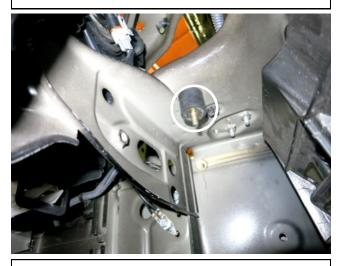
c. Install the rubber mount in the indicated hole, secure with a provided washer and nut.
