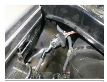
i. Connect the extension harness to the factory connector and route the MAF sensor harness down into the wheel well area.
