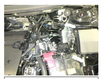
h. Remove the factory intake from the vehicle. Note: Do not discard any of your stock equipment.
