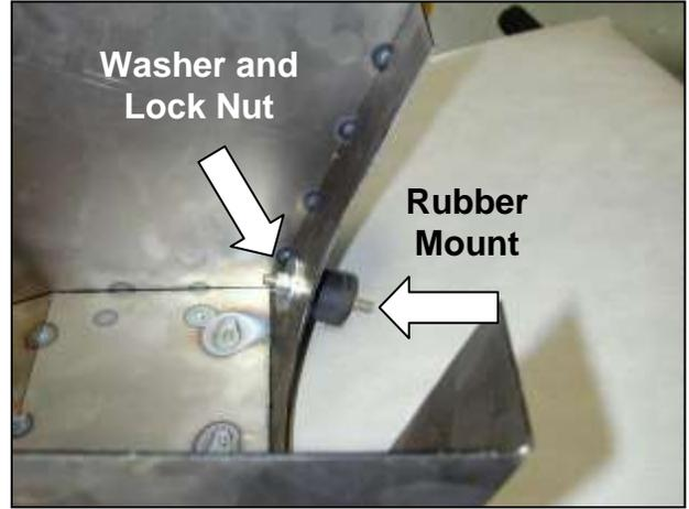
g. Install the supplied rubber mount onto the AEM® heat shield using one each of the supplied M6 washers and lock nuts.
