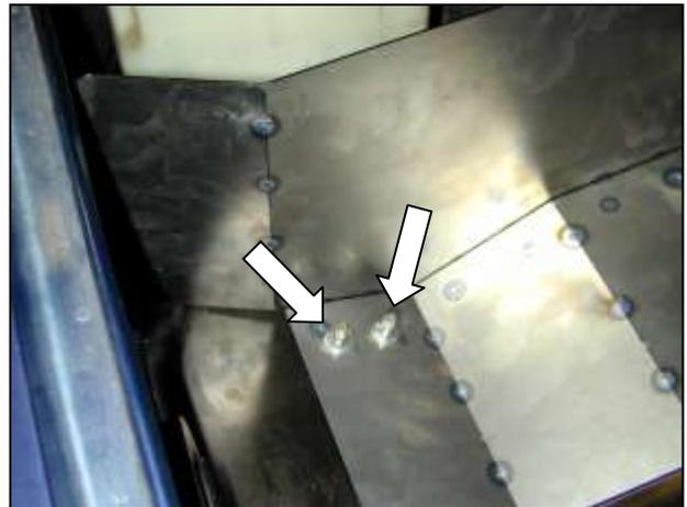
i. Align the hole in the heat shield with the heat shield bracket installed in step 3f. Secure using the supplied M6 bolt, fender washers and lock nut. Once the heat shield is in place, all three mounting bolts may be tightened.
