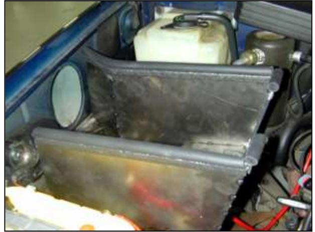
k. Install the foam rubber edge trim on to the top edge of the heat shield. Trim excess as necessary.
