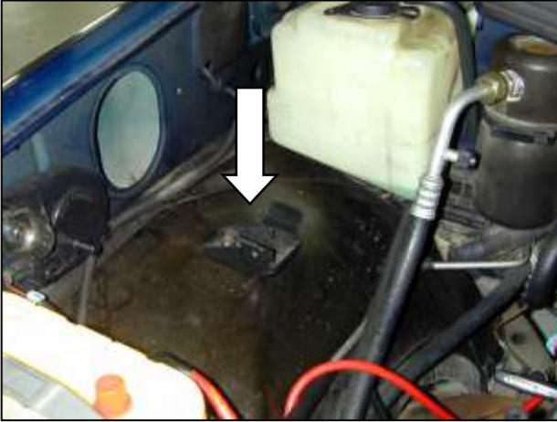
c. From inside the passenger side fender well, remove the two bolts holding the resonator hold down strap bracket. Remove the bracket.
