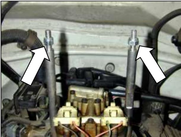
l. Thread two of the supplied 5/16-18 lock nuts on to the standoffs installed in step 3c. Leave approximately  $\frac{3}{4}$ " of thread exposed above the top of the nut. Place one 5/16" washer on top of each nut.
