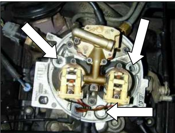
e. Remove the three bolts securing the throttle body to the intake manifold. Make note of the vacuum line connections at the front of the throttle body. Lift the throttle body and remove the old gasket.
