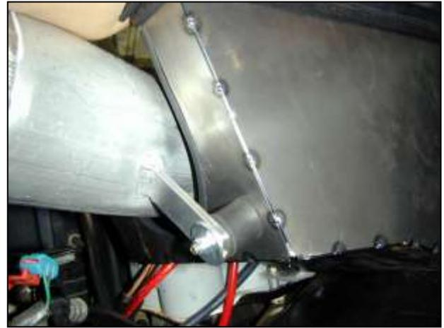
o. Install the AEM<sup>®</sup> inlet pipe into the coupler installed in the previous step. The bracket will line up with the rubber mount on the heat shield. Loosely secure the bracket with an M6 washer and lock nut. Refer to the following diagram for proper rubber mount installation.
