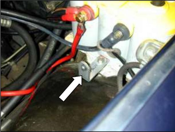
f. Remove the factory battery hold down bolt. Place the AEM® heat shield bracket under the head of the bolt and reinstall.
