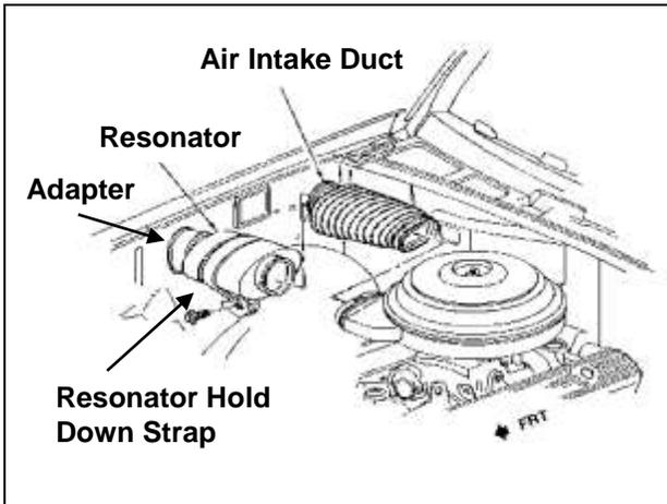
a. Remove the air intake duct, resonator, and adapter from the engine bay. The adapter is removed by gently squeezing the sides in to release the lip from the inner fender.
