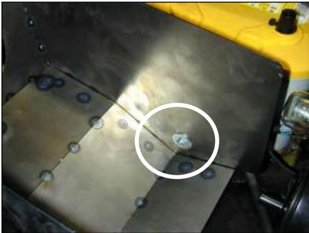
h. Loosely secure the heat shield in the engine bay using the supplied 5/16-18 bolts, washers and lock nuts. Insert the bolts up from the wheel well through the holes exposed in step 2c.
