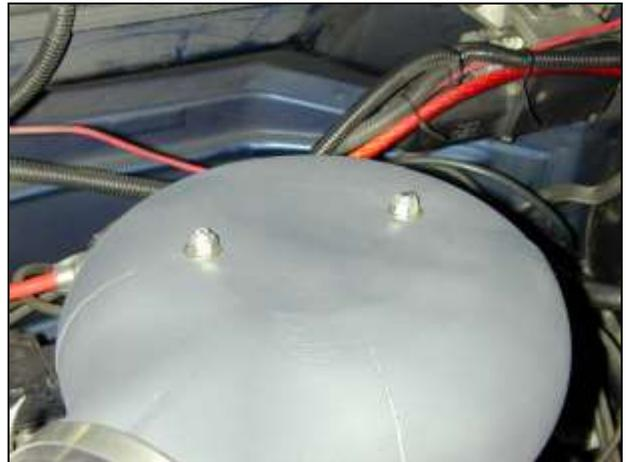
m. Install the air cleaner extension removed in step 2b. Reconnect the breather line on the back side. Test fit the AEM<sup>®</sup> intake plenum. The plenum should not rest on the washers installed in the previous step. Adjust the lock nuts until the top of the plenum compresses approximately  $\frac{1}{4}$ " for gasket sealing. Use the remaining washers and lock nuts to tighten down the plenum.
