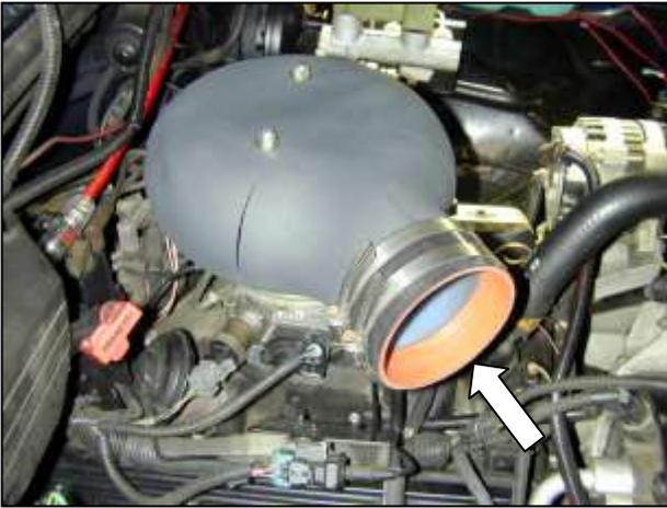
n. Loosely install the silicone coupler and two hose clamps onto the intake plenum.
