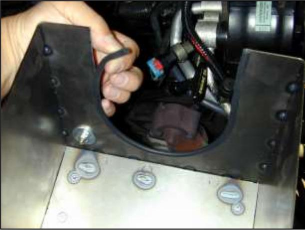
j. Install the rubber edge trim on to the heat shield where the intake pipe passes through.
