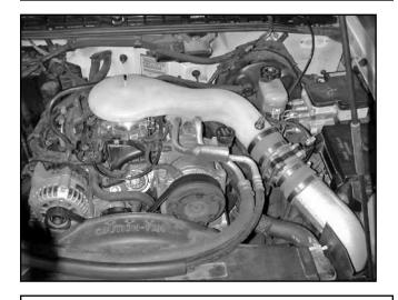
AEM® intake system installed
