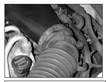
d. Loosen the hose clamp securing the stock intake tube to the plastic throttle body adapter. Remove the entire air box lid / MAF sensor / intake tube assembly from the vehicle.
