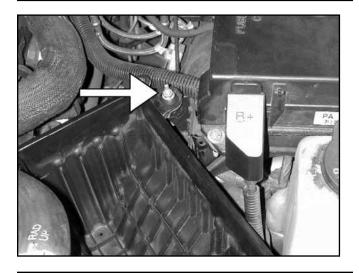
g. Remove the lower air box mounting nut. Remove the lower air box from the vehicle. Remove the lower air box mounting stud. This stud will be replaced with a rubber mount for the AEM® intake pipe later in the installation.
