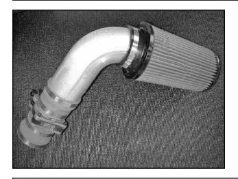
I. Install the AEM® air filter on to the end of the inlet pipe.
