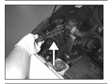
h. Remove the plastic air box mounting bracket located next to the radiator. The bracket is released by sliding it straight up.
