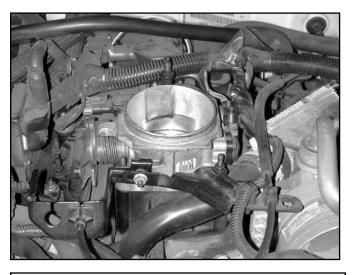
k. Remove the plastic throttle body adapter from the throttle body.
