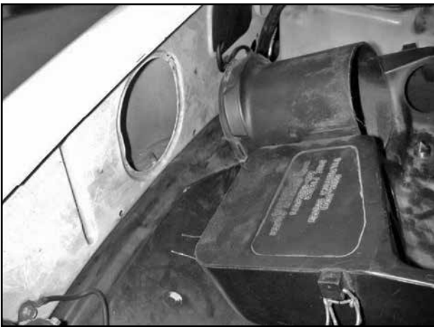
g. Unsnap the air box base from the inner fender and remove it from the engine compartment.
