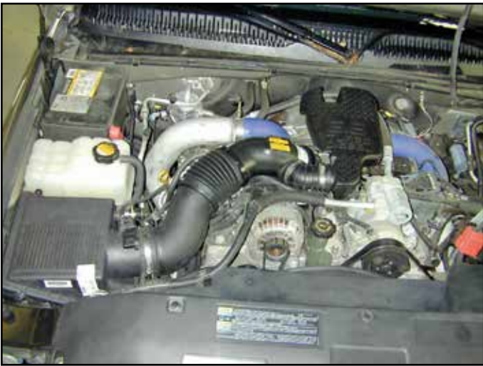
Factory air box system installed
