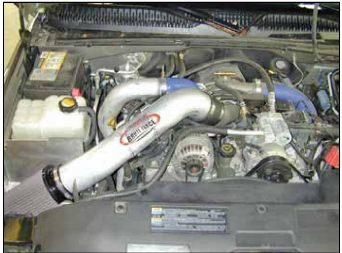
AEM® intake system installed
