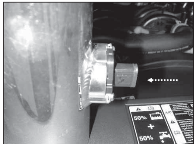
i. Insert the MAF sensor. The airflow direction should be pointing towards the nipple on the pipe. Secure the sensor with the provided washers and bolts.
