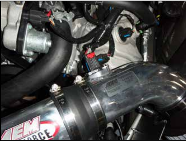
z. Re-connect the mass airflow sensor wiring harness.
