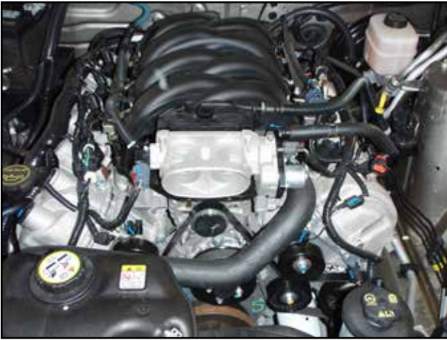
j. Throttle body spacer fully installed and torqued to specifications.
