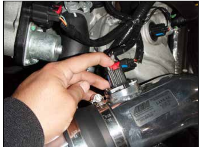
Aa. Lock the mass airflow sensor wiring harness.
