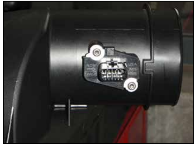
m. Remove the mass air flow sensor from the stock housing, use the supplied torx tool. Immediately install the sensor in the lower AEM® intake pipe.
