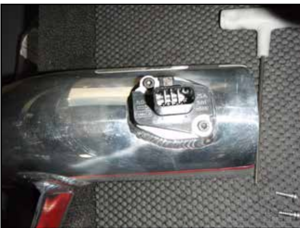
n. Secure the mass air flow sensor in the pipe with the two supplied M4 socket bolts.
