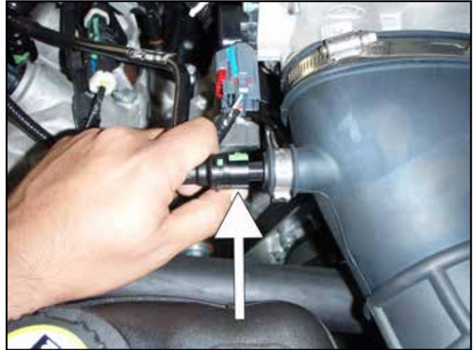
b. Disconnect the PCV hose connected to the inlet tube by pressing on the green retaining clip with your thumb. Then, pull the hose away from the plastic nipple.
