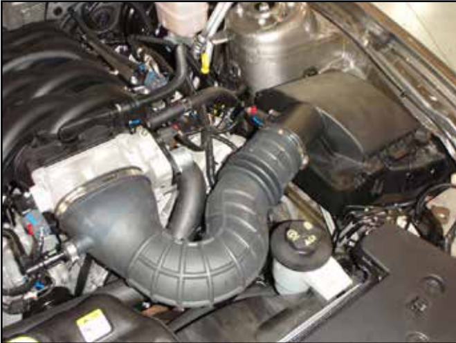
a. Factory air box system configuration.
