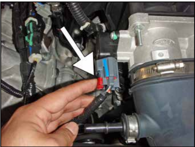
c. With your finger, push the red locking mechanism on the electronic throttle control connector. This is located on the passenger side of the throttle body.
