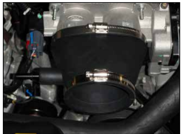
o. Install the #72 hose clamp on the oval side of the coupler and then install the coupler onto the throttle body. Install the #56 coupler on the round side of the coupler. Keep all of the hose clamps loose.
