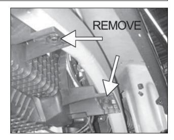
d. Remove the two bolts securing the bottom half of the airbox.
