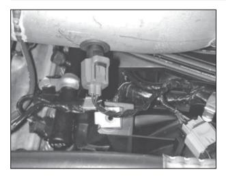
o. Reconnect the wire harness to the IAT sensor. Do not push the grommet through into the intake pipe.
