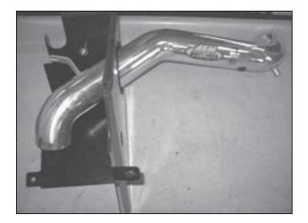
h. Install the intake tube in heat shield. NOTE: Leave the plastic bag over the intake pipe to help prevent damage to the pipe while being installed. Remove the plastic bag after the heat shield is installed.
