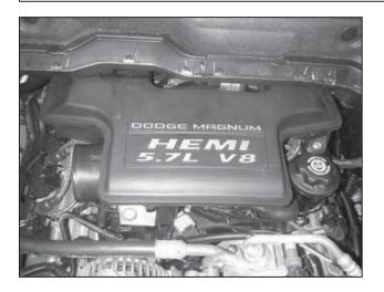
g. Remove the two bolts retaining the intake air resonator (Remove the breather hose if attached to the intake air resonator).
