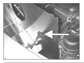
d. Install the rubber grommet in the heat shield's hole as shown. Make sure the groove in the grommet is properly seated in the heat shield.
