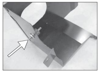
b. Install the supplied rubber mount into the heat shield as shown, place an M8 washer on the stud and an M8 nut to secure.
