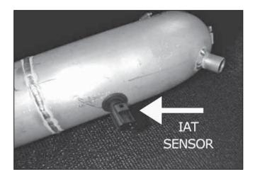
I. Install the supplied IAT grommet into the inlet pipe. Insert the factory IAT sensor into the grommet. Use care to avoid pushing the grommet inside of the pipe.
