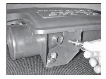
h. Remove the inlet air temperature (IAT) sensor from the intake resonator by gently twisting counterclockwise. Remove the o-ring from the IAT sensor. Keep the o-ring for use if the vehicle ever needs to be returned to stock.
