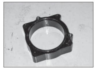
c. Install the supplied o-ring into the groove in the front of the throttle body spacer. Make sure the o-ring is properly seated in the groove around the entire circumference. Use a small amount of grease to trap o-ring in place.
