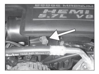
f. Unplug the inlet air temperature (IAT) sensor located on the front side of the intake air resonator.
