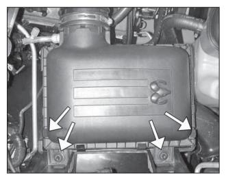
a. Release the four spring clips that hold down the top of the airbox.
