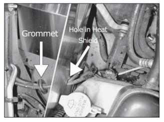
c. Pass both connectors through the supplied large grommet and then through the hole in the heat shield. Reconnect the wire connectors and washer fluid hose to the washer fluid reservoir.
