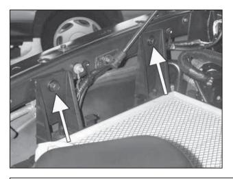
e. From inside the engine bay, remove the two remaining bolts securing the bottom half of the airbox. Remove the bottom half of the airbox and the air filter element.
