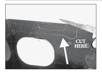
f. On trucks equipped with the optional under hood light on the passenger side, cut the corners on the small section of the top notch in the heat shield using a hacksaw or other suitable tool. Bend the tab back and forth until it breaks free. Clean up any sharp edges with a file. For installation on all other trucks, proceed to next step.
