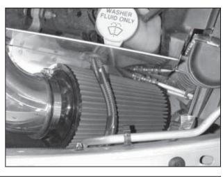
e. Reinstall the AEM $^{\rm \tiny (8)}$  air filter. Adjust the windshield washer hose and wires so they do not rub against the AEM $^{\rm \tiny (8)}$  air filter.
