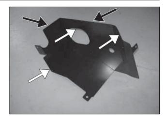
g. Install the rubber edge trim (PN: 8-3034) on the edges indicated with the white arrows. The rubber edge trim will need to be cut appropriately to fit along the heat shield as specified. Install the edge trim (PN: 8-4022) along the top of the heat shield indicated with black arrows.
