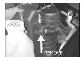
i. Remove the upper radiator fan shroud bolt. On vehicles fitted with a one piece washer radiator overflow reservoir; loosen and remove the mounting bolts and disconnect the overflow tube to gain access. Install the heat shield and intake tube, place the front heat shield tab between the fan shroud and radiator end tank. Replace the factory bolt and overflow bottle if removed.
