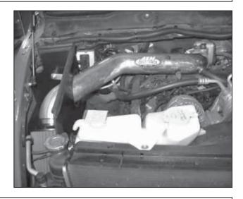
AEM<sup>®</sup> intake system installed
