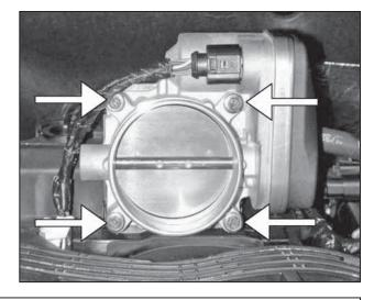
j. Remove the four bolts securing the throttle body. Unplug the electrical connector and remove the throttle body from the intake manifold.
