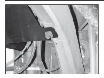
j. The lower heat shield mounting tab will line up with the lower airbox mounting hole. Loosely secure the mounting tab with one of the original bolts.
