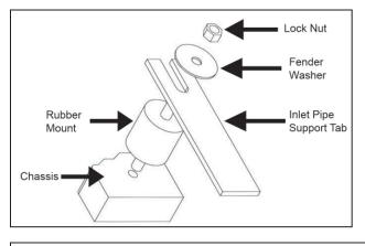
Proper installation of rubber mount assembly.
