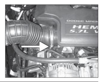
b. Loosen the hose clamp at the intake air resonator (Remove breather hose if attached to the airbox lid). Remove the rubber air hose and the airbox lid.
