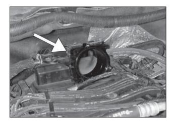
d. Install the throttle body spacer, aligning the pins on the intake manifold with the holes in the back of the throttle body spacer. The o-ring groove on the spacer should be facing forward.
