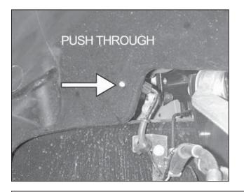
c. From inside the passenger side fender well, release the ABS wire holder. Push the wire holder through the hole towards the engine (if ABS fitted). Remove the plastic fender liner by removing the eight self-tapping screws.
