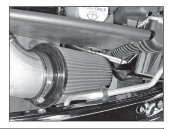
q. Install the AEM<sup>®</sup> air filter from inside the fender well. Slide the air filter onto the intake pipe until it stops. Secure with the supplied hose clamp. Ensure the windshield washer wires and hose do not make contact with the air filter.
