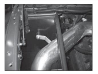
n. Insert the intake pipe as shown. Align the support bracket to the rubber mount and secure. See the diagram below for proper rubber mount assembly installation.
