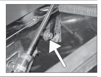
k. The rear mounting tab on the heat shield will line up with one of the lower airbox mounting holes. Install one of the original bolts. Adjust the heat shield for best fitment, then tighten the three mounting bolts.
