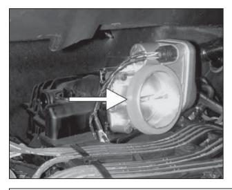
i. Remove the orange rubber gasket from the throttle body.
