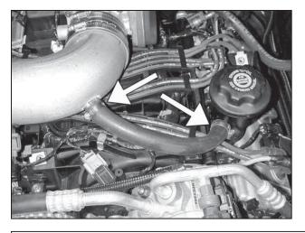
p. Install the supplied breather hose and secure with the two supplied hose clamps.
