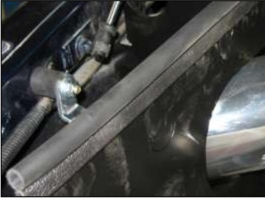
n. Route the intake pipe through the heat shield and line up the bracket with the rubber mount installed earlier. Loosely tighten the supplied washer and serrated nut on the rubber mount securing the bracket.
