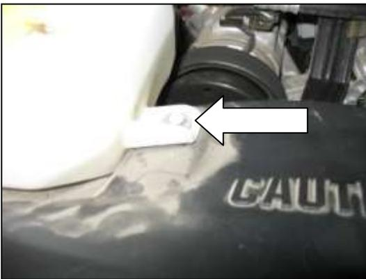
m. Remove the second bolt securing the radiator overflow and windshield washer tank.
