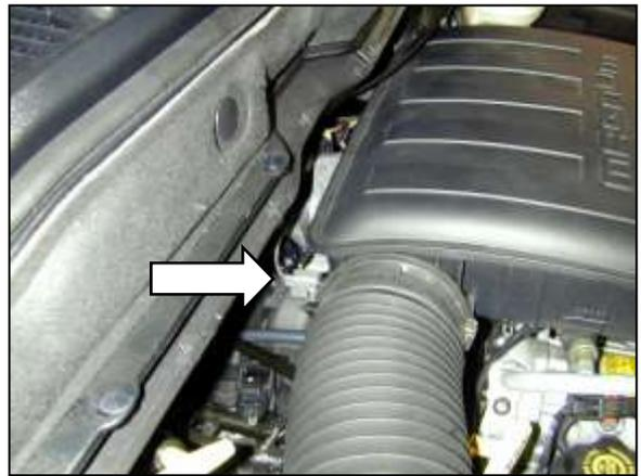
b. Unplug the Inlet Air Temperature Sensor located on the back of the resonator. And remove the bolt securing the resonator to the engine.
