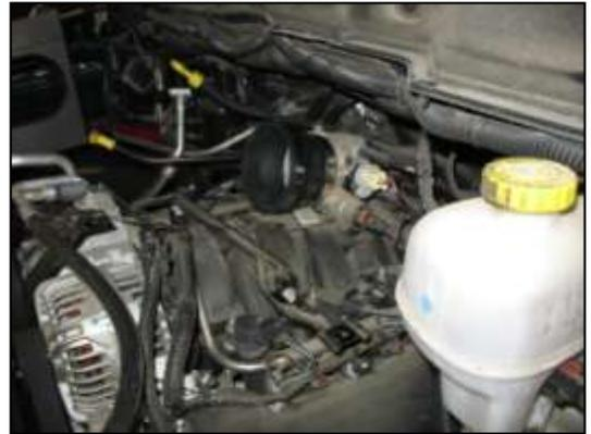
k. Secure the supplied reducing coupler to the throttle body using the supplied hose clamp
