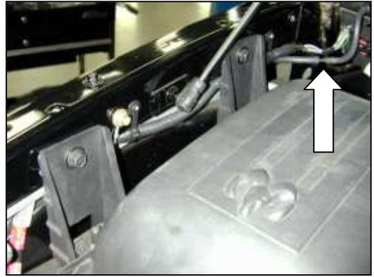
f. Disconnect the breather hose connected to the filter lid. Pull up on the air filter box and remove it from the engine bay.
