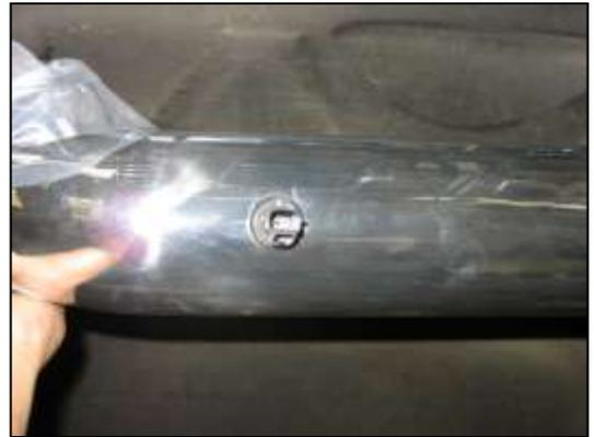
m. Install rubber grommet and Inlet Air Temperature sensor (IAT) in the intake pipe.
