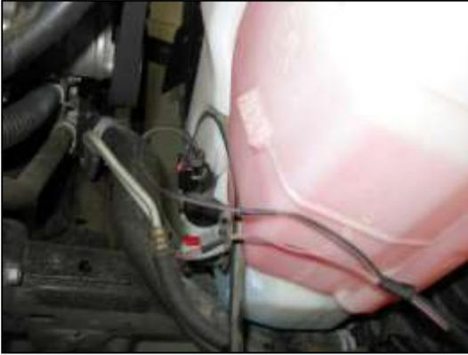
k. Disconnect both wiring harnesses connected to the radiator overflow and the windshield wiper fluid tank.
