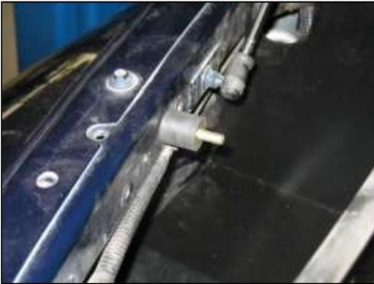
j. Screw in the supplied rubber mount in the threaded hole as shown.
