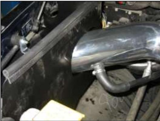
p. Attach the stock breather hose to the nipple on the pipe and secure with the supplied 3/4" hose clamp.
