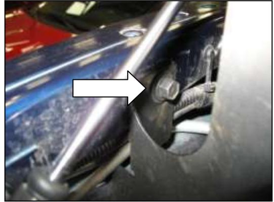
c. Use the stock bolt removed in step 2(h) to secure the heat shield on the passenger side fender.
