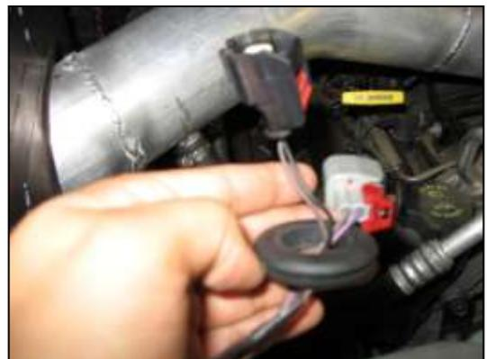
g. Pass the wiring harnesses through the supplied 1" grommet one at a time.
