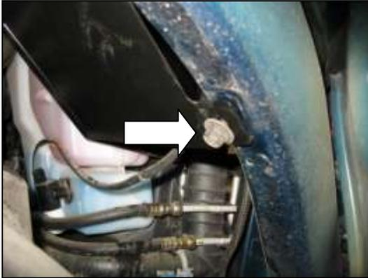
d. Use the stock bolt removed from step 2(j) to secure the final tab on the heat shield.
