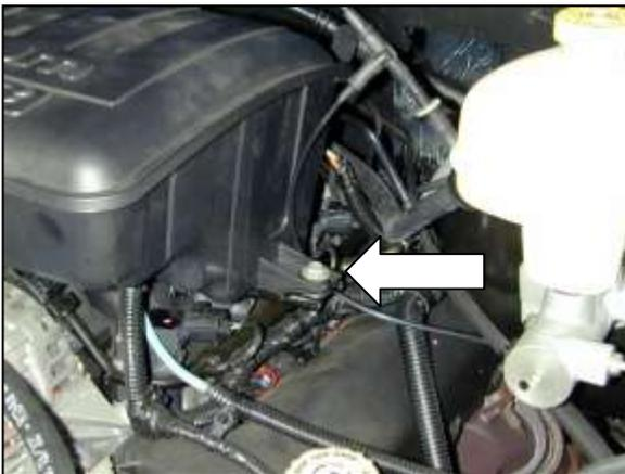
c. Remove the second bolt holding down the resonator
