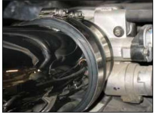
o. Now insert the intake pipe into the already installed reducer coupler. Loosely secure with the supplied hose clamp.
