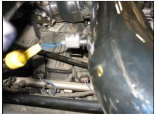
q. Reconnect the IAT sensor wiring harness to the IAT sensor.
