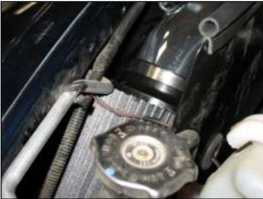
l. Install the Dryflow™ air filter using the supplied hose clamp. Ensure the wires are running through the heat shield go above the air filter. After doing so, install the fender liner that was removed in step 2(g).
