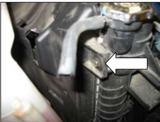
o. Finally, remove the bolt attaching the fan shroud the radiator exposed by the previous step. Keep the bolt, it will be used to install the heat shield.
