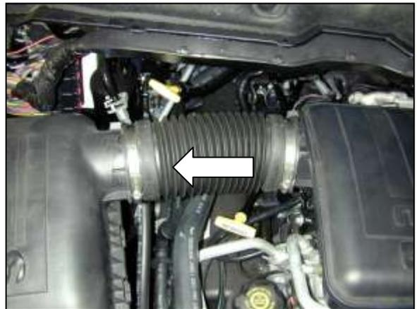
d. Loosen the hose clamp connecting the intake tube to the air filter lid. Then pull off the resonator and the hose connected to the air filter lid.
