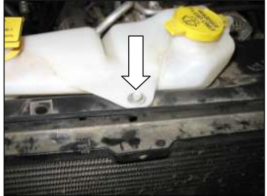
e. Pull the tank back toward the front of the truck and re-secure the tank back to the radiator with the two stock bolts. Reconnect the over flow hose.
