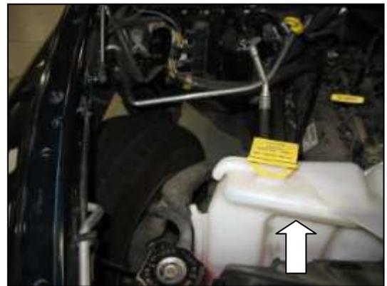
n. When performing the following step Please be sure your vehicle has cooled down. Carefully disconnect the overflow hose to the overflow tank and lean the tank toward the engine as seen in the picture.
