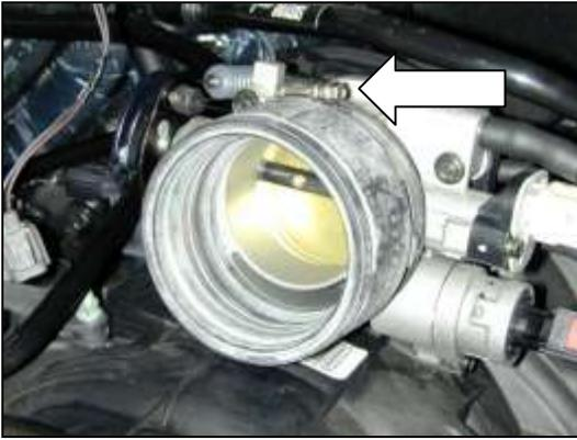
e. Remove the coupler on the throttle body by loosening the hose clamp.
