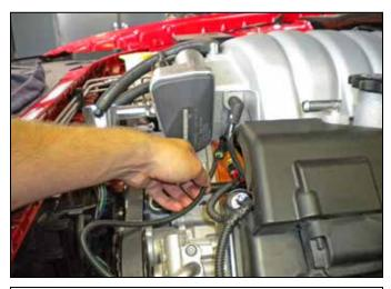
c. Route the IAT extension harness underneath the throttle body and towards the driver side of the engine.
