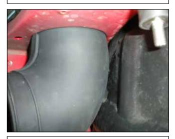
e. Make sure that the hump is all the way through the hole, then release the coupler and manipulate it until the sheet metal "snaps" into the grove in the coupler.
