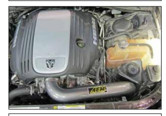
AEM® intake system installed
