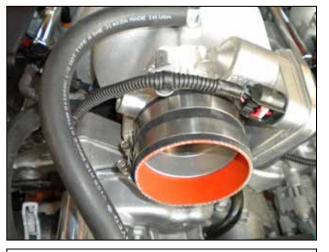
c. Install the silicone coupler and two #56 clamps onto the throttle body. Slide the coupler all the way onto the throttle body and secure it by tightening one of the #56 clamps.
