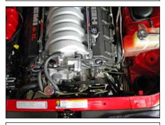
d. Pull the rubber inlet hose off of the throttle body, then lift and remove the OEM air box assembly.
