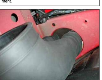
d. From underneath the vehicle, hold the collapsed coupler firmly, then insert it into the large hole in the sheet metal.
