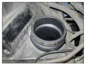
b. Loosely install a #56 hose clamp over the upper opening of the elbow hump hose.
