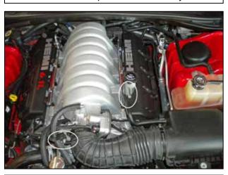
c. Unplug the IAT sensor. To unplug the IAT sensor, slide the red tab back to unlock the latch on the plug, then press in on the latch and pull the plug off of the sensor. For "grey" tabbed connectors, push the top of the gray tab in and simply pull the connector off.
