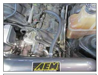
f. For Most Applications: Install the supplied  $\frac{1}{2}$ " ID hose between the crank case vent on the head cover and the nipple on the upper intake pipe. Secure the  $\frac{1}{2}$ " hose with two small hose clamps.
