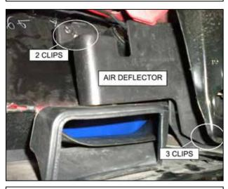
i. For maximum performance from your intake system, you may choose to remove the air deflector. If equipped, the air deflector will be located behind the lower grill on the driver side. Removing this will provide additional cold air flow to the air filter.
