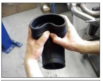
c. Hold the rubber coupler as shown, squeeze the hump end of the coupler to collapse it into itself.
