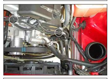
d. Route the IAT extension harness and secure it with the two zip ties as shown. Position the female IAT connector next to the lower intake tube.
