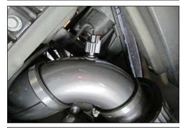
e. From underneath the vehicle, plug the female IAT connector into the IAT sensor in the lower intake tube. Pull the red lock tab up to secure the connector.
