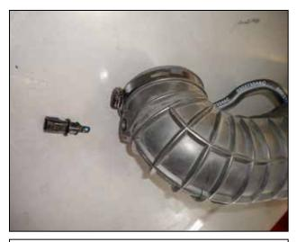
e. Carefully remove the IAT sensor from the OEM rubber inlet hose. Set the sensor aside for future use.
