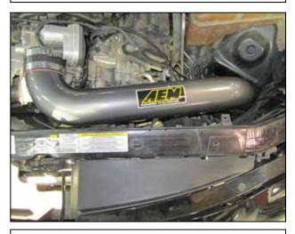
e. The lower end of the pipe should be inserted into the rubber coupler to a depth of about <sup>3</sup>/<sub>4</sub>" to 1". Slide the pipe all the way into the throttle body coupler until it bottoms out. Once proper fitment is achieved, tighten the two remaining hose clamps.
