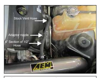
g. **On some 5.7L engines:** Connect the stock crank case vent hose to the supplied plastic adaptor nipple. Connect a 4" section of the ½" ID hose onto the other end of plastic adaptor nipple. Connect the hose to the intake pipe and secure with the small hose clamps as shown.
