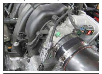
b. Select the appropriate IAT extension harness based on your vehicle's IAT connector. (Item L or O.) Connect the male connector to the factory harness as shown. Pull up on the red tab to lock it.
