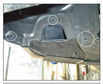
f. In the wheel well area on each side, remove the 3 clips securing the belly pan.
