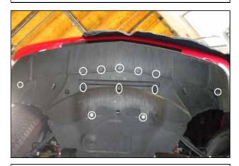
h. Install the belly pan with the 9 clips, 7 screws, and 2 bolts removed in steps 2f and 2g.
