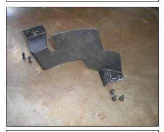
j. To remove the air deflector, remove the five plastic rivets securing it to the fascia. The rivets can be removed by pulling the center pin out from the back side of the rivet.
