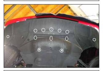
g. From underneath the car, remove: 3 clips, 7 screws, and 2 bolts from the belly pan. (May vary with each vehicle.)
