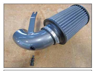
g. Install the grommet into the lower pipe and attach the filter with one #56 clamp as shown.
