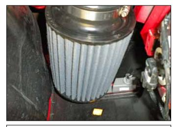
j. Adjust the lower pipe assembly so that there is equal space between the filter, bumper support, fender liner, and marker lamp. When a good fit is achieved, tighten both nuts on the rubber mount and the #56 clamp.
