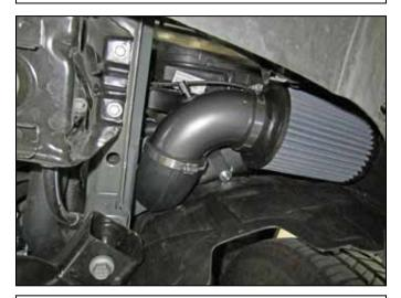
i. Install the lower pipe assembly as shown using one M8 washer, one M8 nut, and one #56 clamp.
