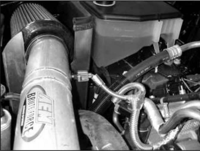
q. Reattach IAT sensor wire harness connector.
