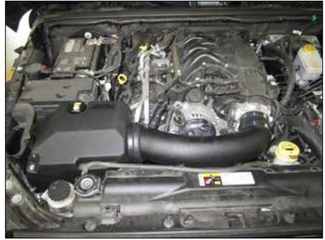
t. Insert the 4 M6 by 30mm bolts into the bolt holes in the top of the airbox lid. Place the airbox lid carefully onto the lower air box, aligning the 4 bolt holes.
