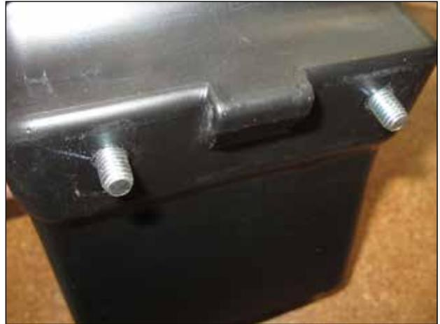
b. Insert two M6 buttonhead bolts into the drilled out holes inside the stock inlet tube you removed in Step (2-1) above.
