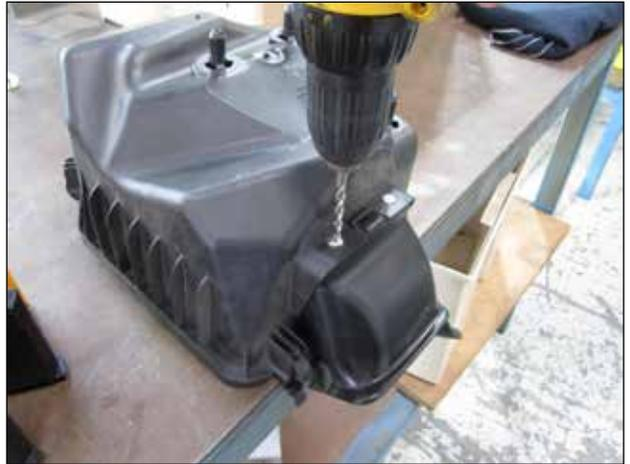
l. Use a 1/4" drill to remove the rivets mounting the stock inlet tube to the lower air box. Remove the inlet tube for use with your AEM intake.
