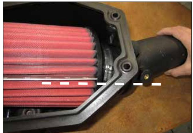
l. Insert the straight end of your AEM intake tube thru the airbox lid outlet hole and into the Dryflow air filter inside. Align the hose clamp hex nut with the mounting boss on the bottom of the AEM intake tube and tighten clamp.
