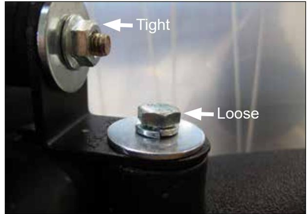
p. Install a flat washer, split washer, and M6 x 12mm bolt through the slotted hole in the "L" bracket and into the mounting boss on the intake tube. Tighten the bolt by hand until snug to allow for adjustment. Now fully tighten the M6 nut installed in the previous step.
