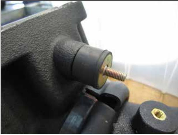
g. Install the M6 rubber isolator mount onto the boss on the airbox lid as shown. Tighten by hand.
