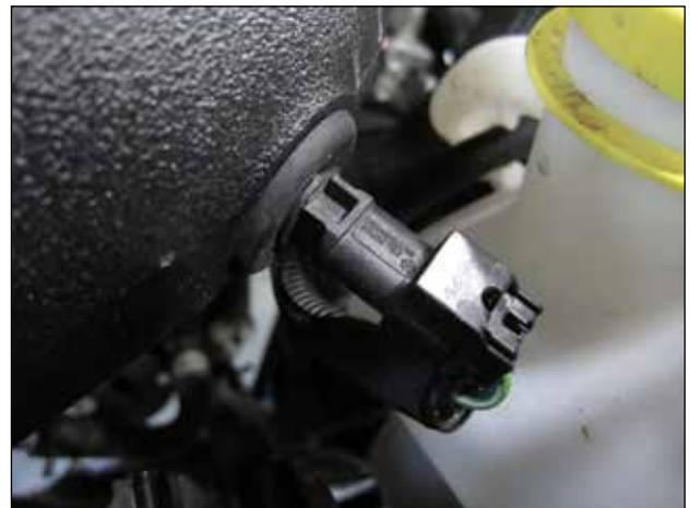
r. Bring the intake tube and upper lid assembly into the engine bay. First, connect the IAT sensor to the stock wiring harness.
