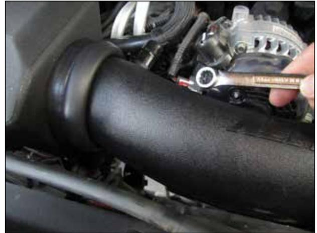
v. Using a 10mm box wrench, reach under the intake tube to tighten the M6 bolt that you installed by hand through the "L" bracket in Step (3-p) above to secure the tube to the airbox.
