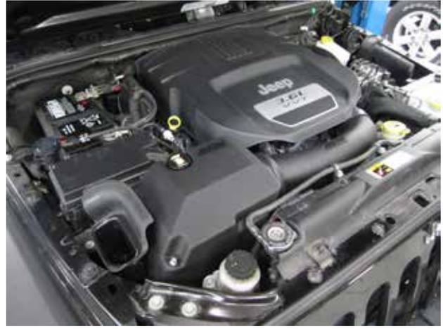
z. Re-install the engine cover. AEM-21-8316 Brute Force Intake System shown installed.
