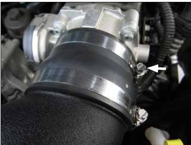
w. Now tighten the smaller hose clamp at the throttle body.
