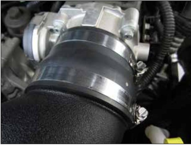
s. Install the rubber adapter over the throttle body as shown. **Do not tighten** the small hose clamp yet.
