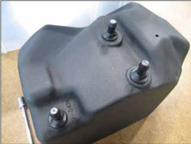
a. Install the 3 plastic air box mounts using 3 M6 X 12mm bolts and 3 split washers inside your new AEM lower airbox and fully tighten them.
