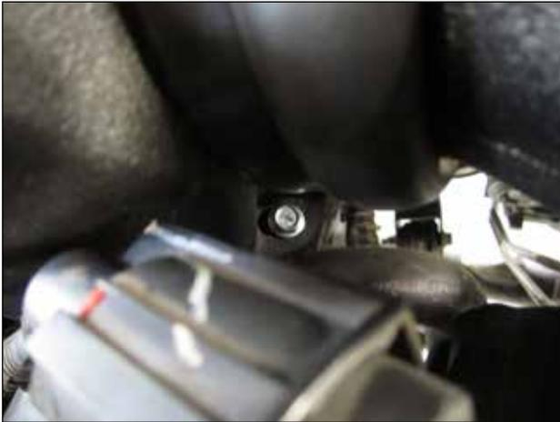
u. Start threading all 4 bolts before tightening. A long  $\frac{1}{4}$ " ratchet extension and U-joint is recommended to tighten the lower 2 bolts with a 10mm socket.
