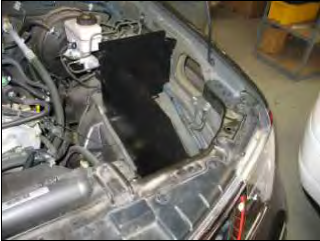
b. Insert the heat shield into the engine bay.
