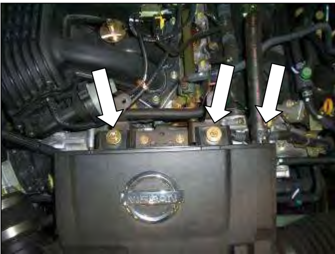
c. Loosen and remove mounting bolts for the combination resonator chamber and inlet tube. Remove crankcase breather tube from the resonator housing.
