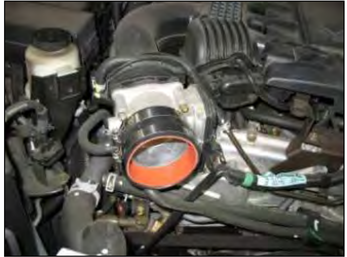
g. Attach and secure coupler at the throttle body with provided hose clamps.
