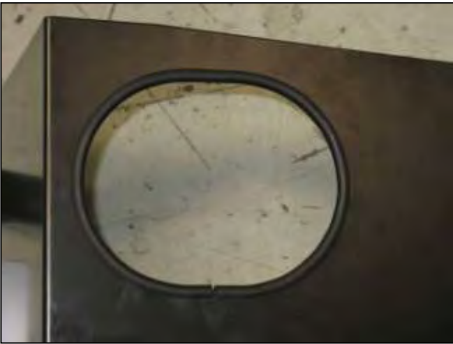
h. Use rubber trim around the intake pipe opening on the heat shield.
