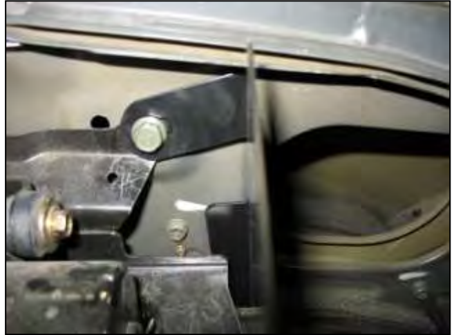
c. Remove stock bolt, then immediately reinstall the stock bolt through the heat shield hole.
