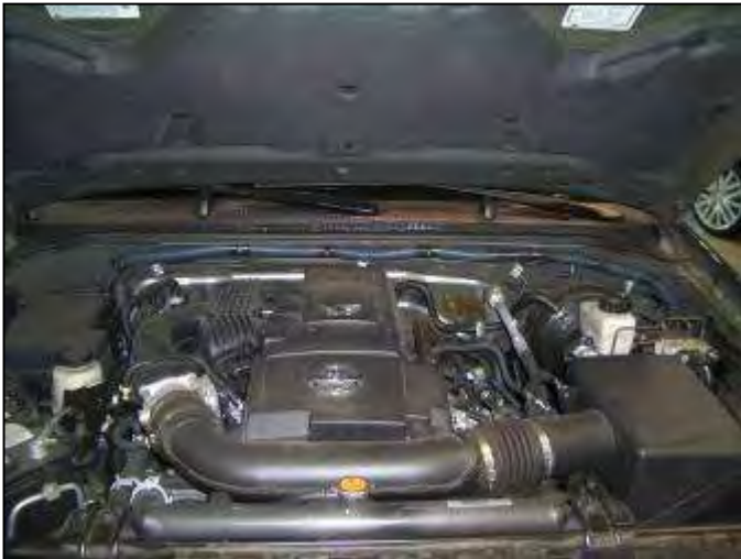
a. The stock engine bay should look like this. Loosen hose clamps at the throttle body.
