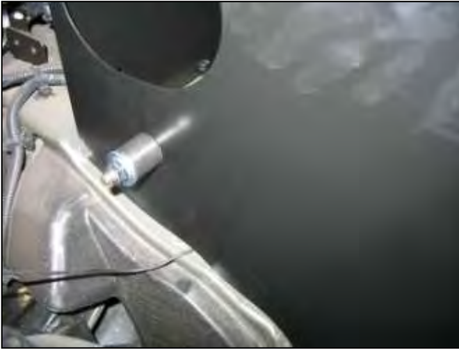
f. Insert and secure the rubber mount through the heat shield.
