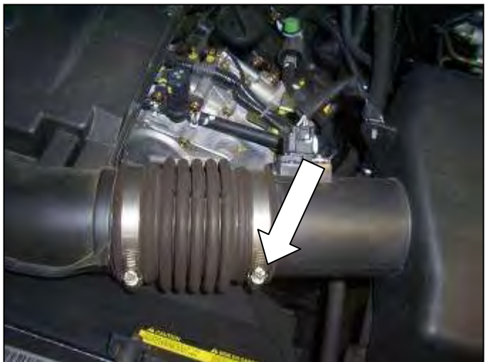
d. Loosen the hose clamp at the air box. Remove the combination resonator chamber and inlet tube.
