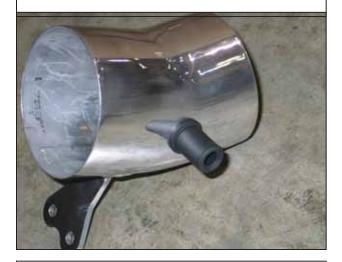
h. Install the rubber adapter into the inlet of the intake pipe as shown.
