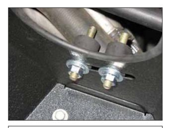
g. Install the two supplied rubber mounts into the slot on the heat shield using two M8 nuts and washers. Secure the mounts with just enough slack for the mounts to slide in the slot.
