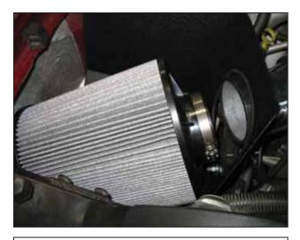
j. Slide the air filter into the heat shield with the filter neck facing the engine. This will ease installation, as the air filter cannot easily be installed if the lower intake pipe is already installed.
