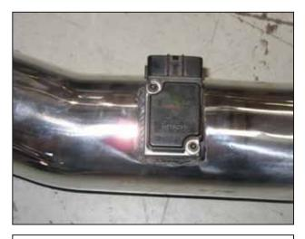
c. Install the previously removed MAF sensor into the upper intake pipe using the two supplied 8-32 bolts.
