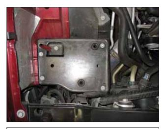
f. Remove the five bolts securing the air filter housing mounting plate to the vehicle chassis.
