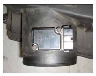
i. Using the supplied tamper-proof torx key, remove the two bolts secuing the MAF sensor to the air filter housing. Carefully remove the MAF sensor from the housing.
