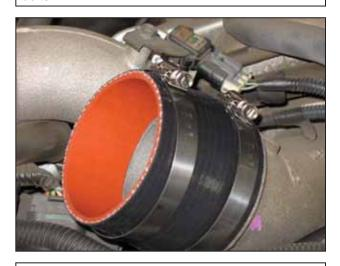
e. Install the 3.50" coupler onto the turbo inlet. Loosely secure the coupler with the supplied #56 hose clamps.
