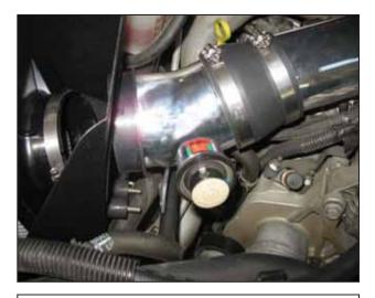
k. Attach the reducing coupler to the lower intake pipe. Install the lower intake pipe into the upper intake pipe's coupler while also aligning the mounting bracket holes with the two rubber mounts attached to the heat shield. Loosely secure the intake pipe in place with a #64 hose clamp.
