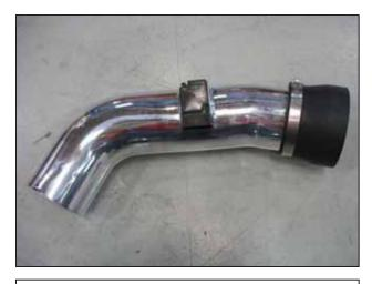
f. Install the reducing coupler onto the upper intake pipe as shown. Slide the coupler all the way onto the intake pipe with a #56 hose clamp; do not tighten the hose clamp.
