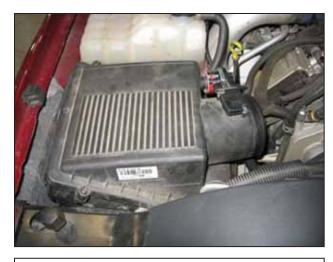
e. The air filter housing is held in plce by two grommets on the mounting plate. Gently lift up on the air filter housing and remove it from the engine bay.
