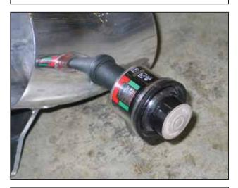
i. Install the previously removed air filter restriction gauge into the rubber adpater in step 3h.
