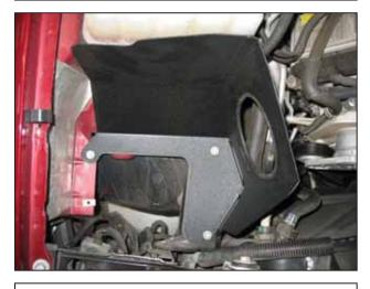
d. Install the heat shield in the engine bay, aligning the holes with the mounting plate bolt locations. Secure it using three of the bolts removed in step 2f.
