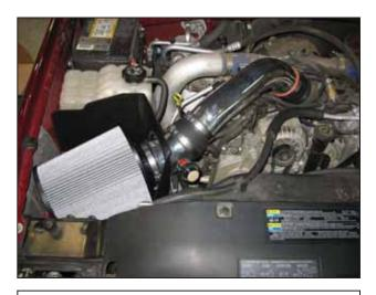
AEM® intake system installed
