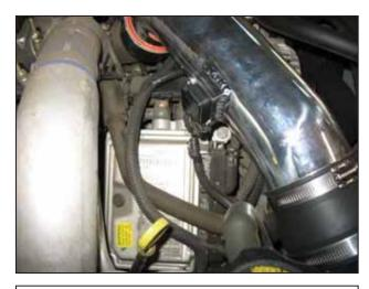
n. Plug the MAF sensor into the wiring harness. Be sure that the harness is not in contact with any hot part of the engine.
