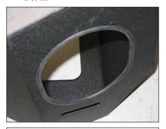
b. Install the supplied rubber edge trim around the edge of the hole in the heat shield. Trim to fit.
