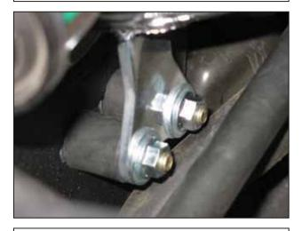
I. Slide the lower intake pipe and reducing coupler down from the upper intake pipe until the mounting bracket face is flush with the rubber mounts. Install the remaining M8 washers and nuts to secure the lower pipe's mounting bracket.
