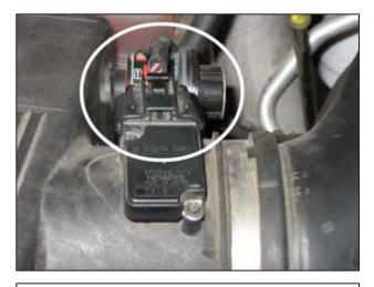
b. Unplug the mass air flow (MAF) sensor wiring harness.
