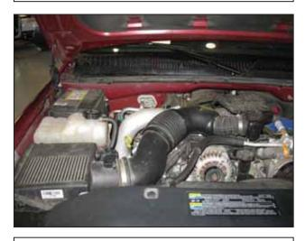
Factory air box system installed
