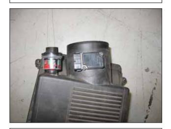
h. Remove the factory air filter restriction gauge.
