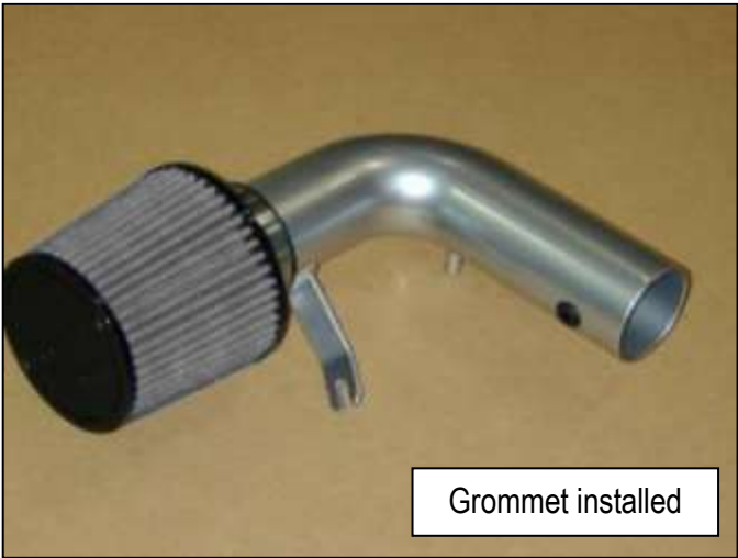
h. Assemble pipe as shown. Install filter to the end of the pipe with the bracket. Install grommet as shown.
