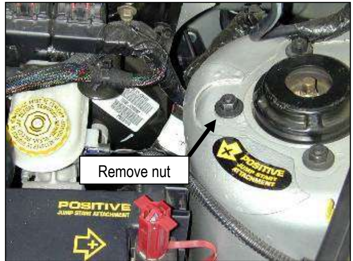
h. Remove the nut from the strut tower and reuse when installing heat shield.
