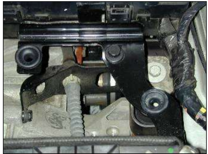
f. Remove the air box by pulling straight up.
