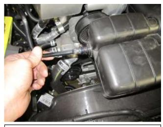
a. Disconnect the plastic breather pipe from the side of the factory intake resonator.
