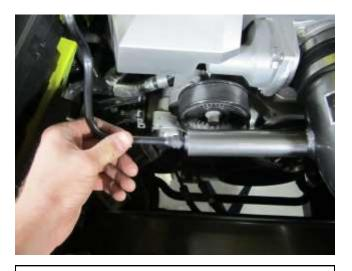
h. Install the plastic breather pipe that was disconnected in 2a. into the AEM intake.
