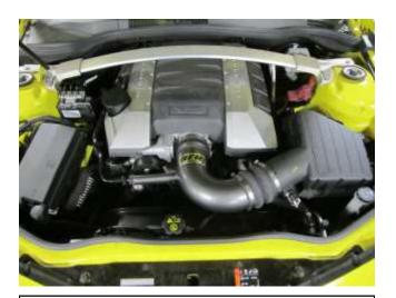
AEM® intake system installed
