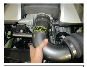
e. Install the intake tube into the throttle body coupler.
