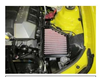
a. Install the AEM air filter into the air box base as shown.
