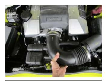
d. Remove the stock intake from the vehicle. **NOTE:** Do not discard any of the factory intake components.
