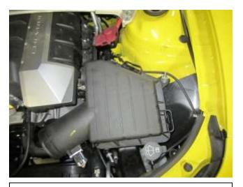
b. Install the air box lid back onto the air box base making sure the tabs latch.
