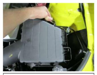
e. Unclip the two tabs retaining the air box lid and remove the lid to expose the stock air filter.
