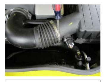
c. Loosen the hose clamp at the air box.
