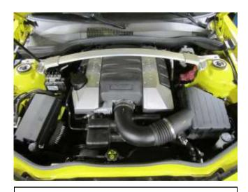
Factory air box system installed
