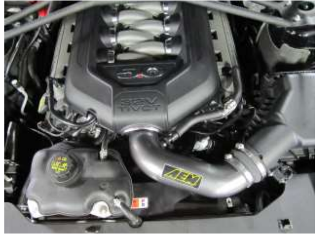
AEM® intake system installed
