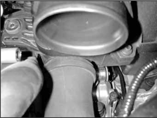
i. Disconnect the lower intake tube from the air filter box. Remove the air filter box.
