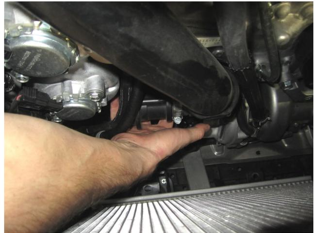
h. Lift straight up on the valve outlet while supporting the inlet to remove the factory charge pipe from the engine.
