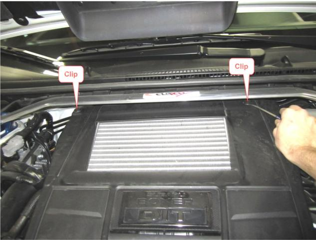
e. Release engine cover clips and remove engine cover by lifting up firmly on the front of the cover.
