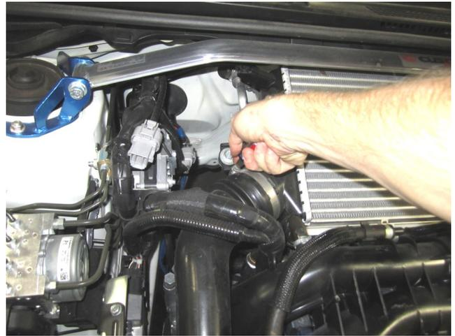
f. Loosen clamp securing the charge pipe to the inter-cooler enough to move the clamp off of the joint.
