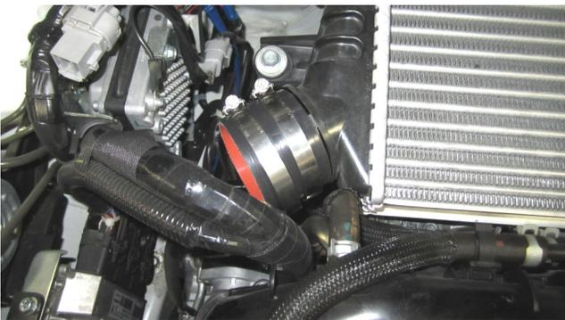
a. Install the 2.75" coupler onto the intercooler inlet with its corresponding hose clamps. Do not tighten.
