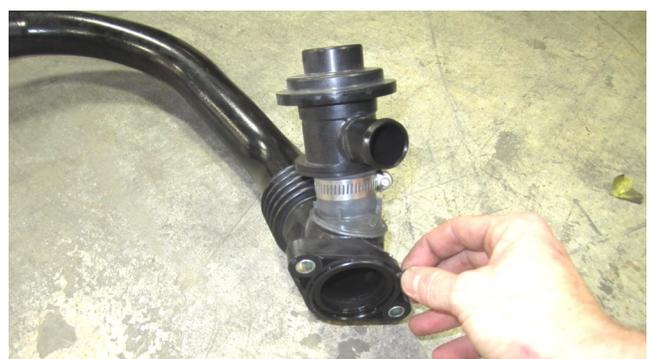
b. Remove the O-ring from the factory charge pipe and install into your new AEM charge pipe with care to orient the tab in its corresponding groove.
