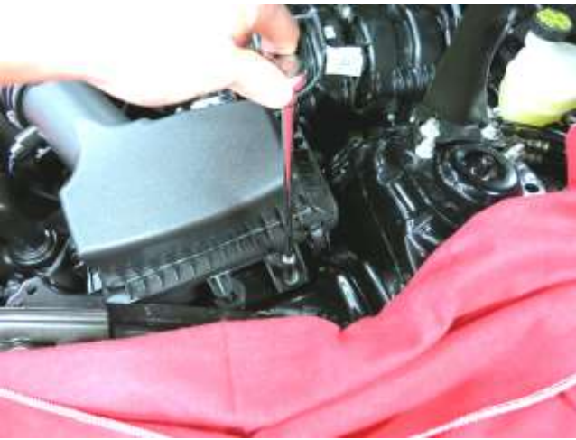
a. Use 10mm socket to remove the bolt securing the factory air box.
