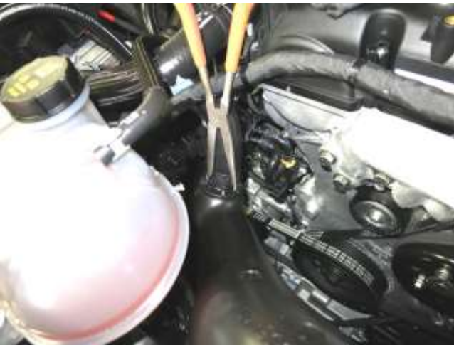
c. Use pliers to release the clamp securing the recirculation hose to the factory intake tube and disconnect the hose from intake tube.
