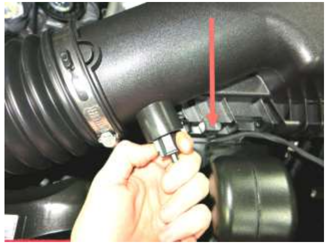
b. Remove wiring harness from the inlet air temperature (IAT) sensor and use pliers to remove the harness from the air box where shown by the arrow above.
