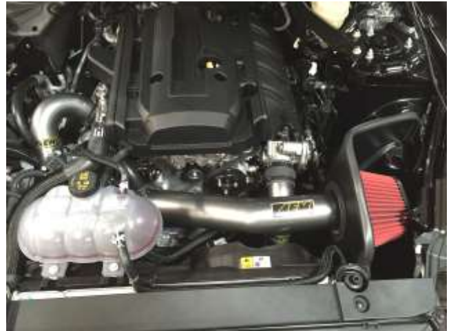
Finished installation of AEM Charge Pipe System (shown with AEM Intake System 21-740C.)
