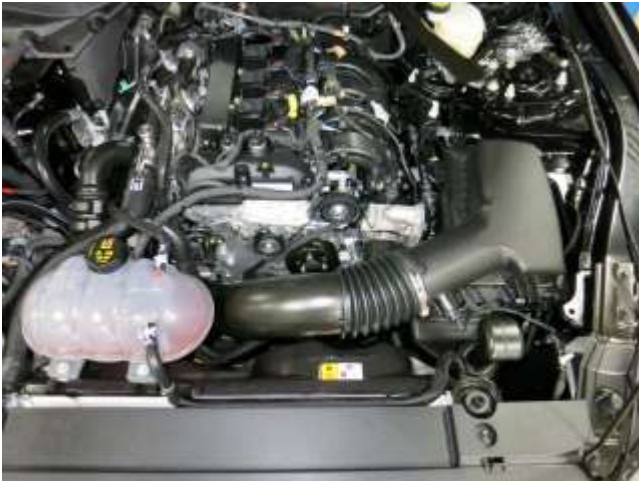
Factory charge plumbing system.
