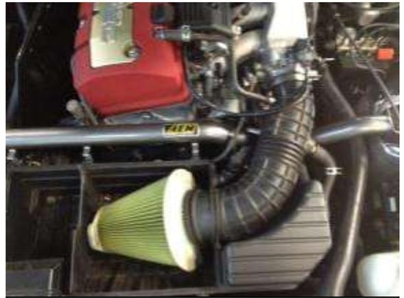
b. Re-install the intake tube/air filter assembly.
