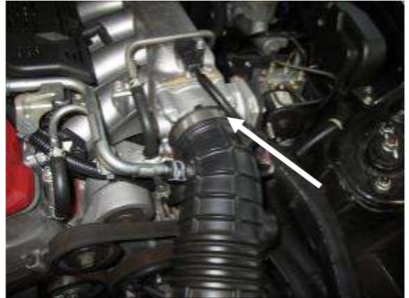
b. Loosen the clamp holding the intake tube to the throttle body.
