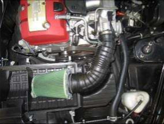
a. Unclip and remove the airbox cover.
