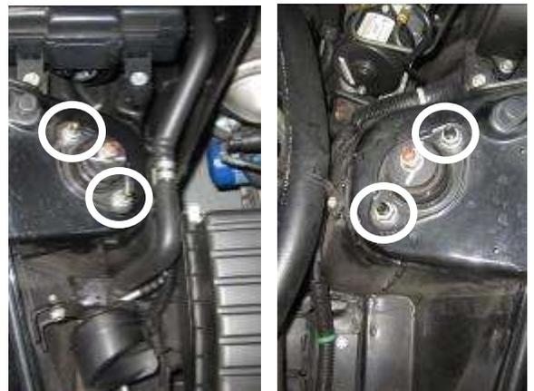
d. Remove the 4 damper nuts.
