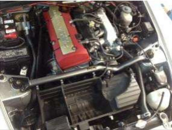
a. Place the AEM strut tower bar over shock studs, replace and tighten damper nuts.
