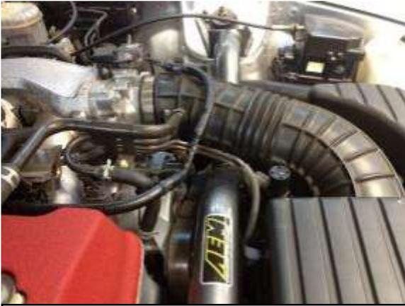
g. On some cars, the metal vacuum lines may need adjustment for clearance
