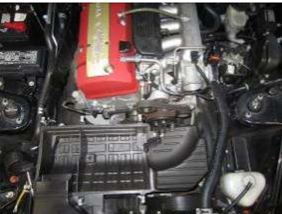
c. Unplug AIT sensor, unclip sensor wires from the intake tube. Loosen the clamp holding the vent tube to the intake tube, and remove the intake tube/air filter assembly.
