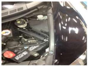
c. Pull the 3 plastic fasteners holding the passenger side fender finisher, and remove the finisher.
