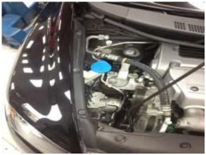
Pull the 3 plastic fasteners holding the drivers side fender finisher, and remove the finisher.
