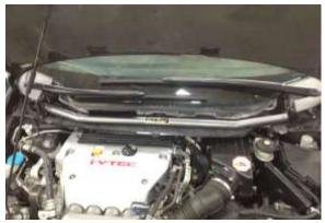
b. Place the AEM strut tower bar over the strut tower studs.
