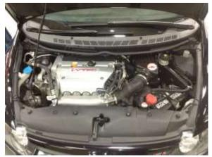
d. Remove the 3 plastic fasteners that secure the center cowl finisher, and carefully pull the finisher up to remove it from the cowl panel.
