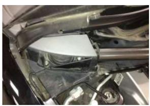
c. Using a 14mm socket, replace the strut tower nuts.
