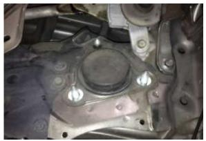
a. Place the 4 included washers over the strut tower studs.
