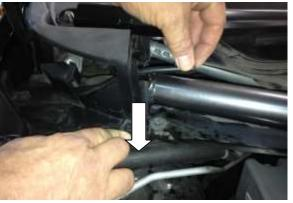
d. Make sure the windshield washer tubing is not pinched between the finisher and the strut tower bar.
