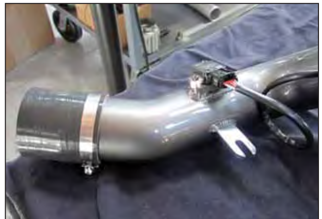
g. Slide coupler (5-273) onto the upper tube about 1-1/8th inch and fasten with #44 hose clamp.
