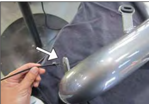
f. Insert the tree mount zip tie into the bracket of the upper intake tube as shown.
