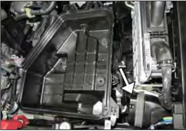
k. Disconnect lower airbox from inlet tube. Remove the lower airbox and set aside.
