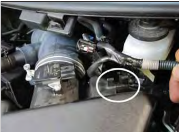
c. Disconnect wire harness from MAF sensor and unclip MAF wire harness from stock airbox.
