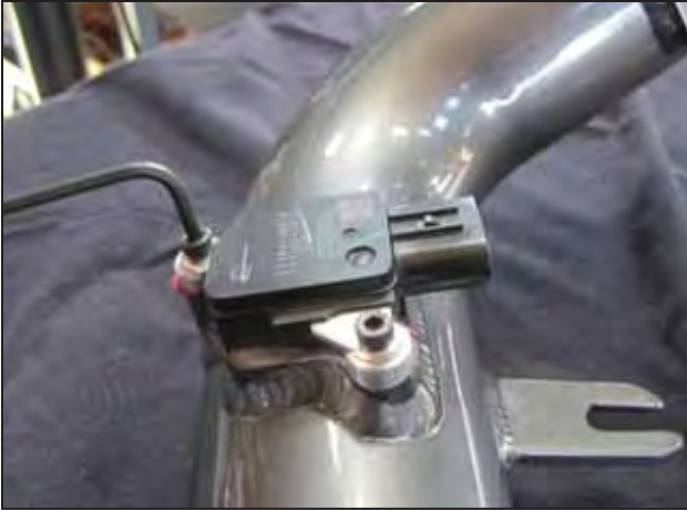
b. Install the MAF sensor onto the upper intake tube (2-1465) using the provided M4 bolts(1-2105), tighten with an allen wrench.
