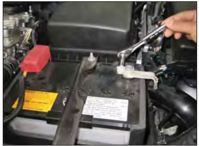
b. Disconnect negative terminal on battery using 10mm socket and tuck away from battery.
