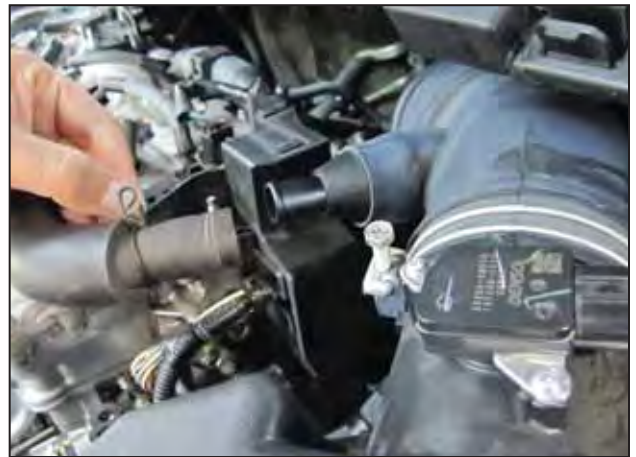
d. Pinch and slide back the black spring clamp on the valve cover hose. Twist valve cover hose to disconnect from intake tube.
