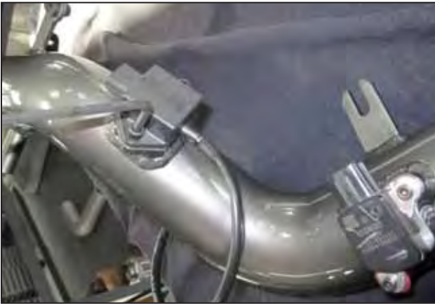
d. Mount the ETI module onto the upper intake tube using the provided M6 bolts(1-2041).
