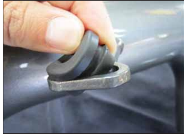
c. Insert the rubber grommet (1675-044) into the VSV bracket as shown.
