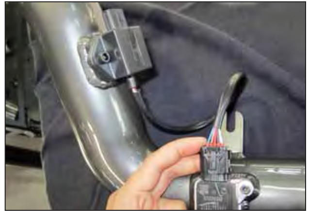
e. Connect the ETI module harness to MAF sensor as shown.
