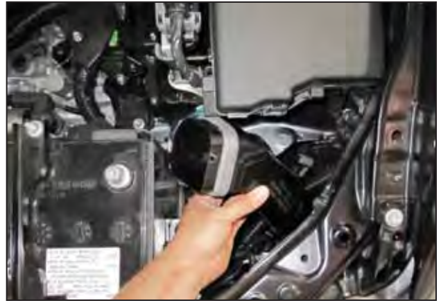
l. Slide the inlet tube down towards the headlight slightly and remove the inlet tube from the vehicle.
