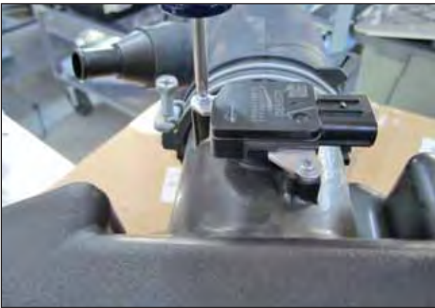
m. Remove the MAF sensor using a Phillips head screwdriver and set aside for later use during the AEM® intake installation.
