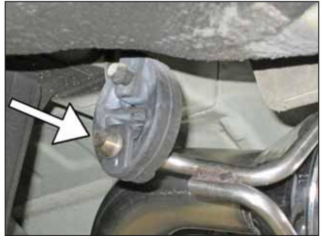
c. Install the exhaust bracket in the single rubber isolator.
