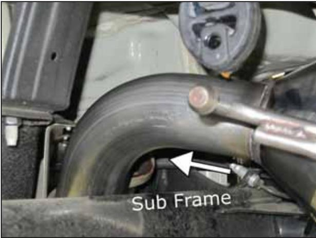
b. Route the exhaust pipe over the rear sub frame.
