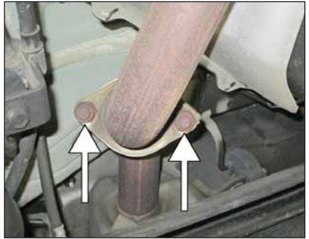
b. Remove the two nuts securing the muffler pipe to the exhaust pipe.
