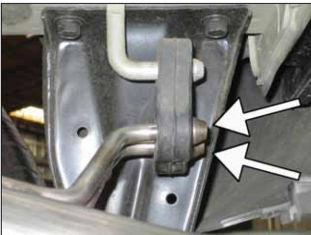
d. Install the two exhaust hangers into the rear rubber isolator.
