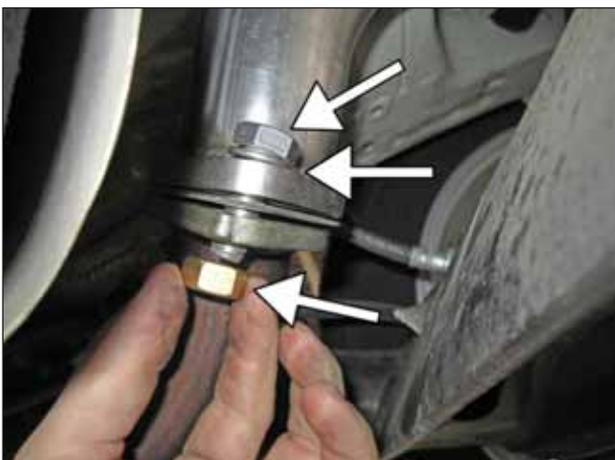
f. On each side of the exhaust flange, install a supplied bolt, washer and nut as shown. Ensure the gasket is properly aligned with the exhaust flanges and the bolts slide through gasket's bolt holes.
