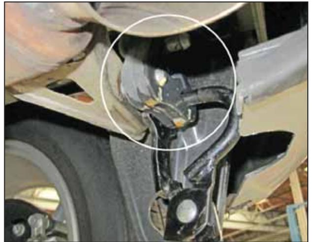
d. Disconnect the two exhaust hangers from the rear rubber isolator.
