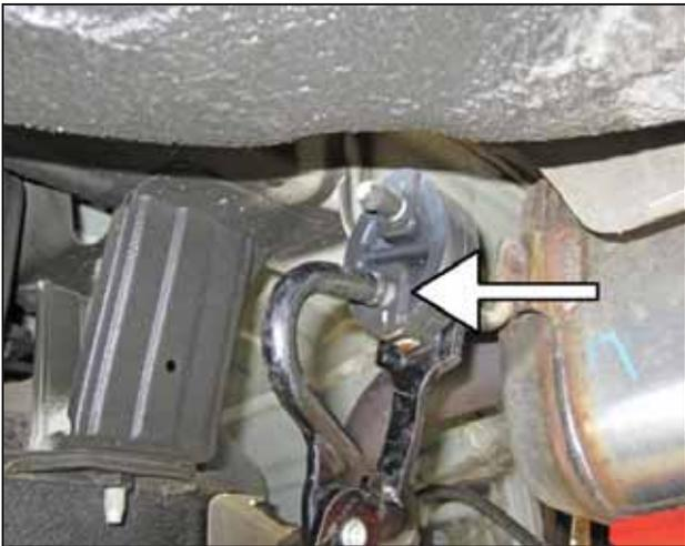
c. Disconnect the exhaust hanger from the rubber isolator.
