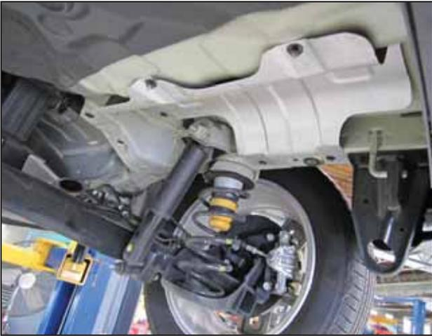
e. Remove the OE muffler, ensure the exhaust gasket is removed and set aside. The gasket will be reused during the installation of the AEM® exhaust system.
