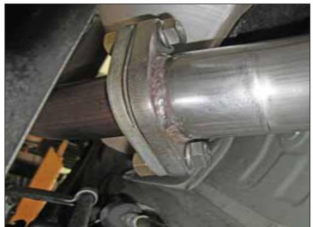
g. Ensure the bolt/nut assemblies are tightened to factory torque specification (see service manual).
