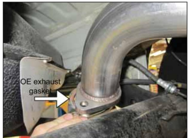
e. Install the OE exhaust gasket between the OE exhaust pipe and the AEM® exhaust pipe.
