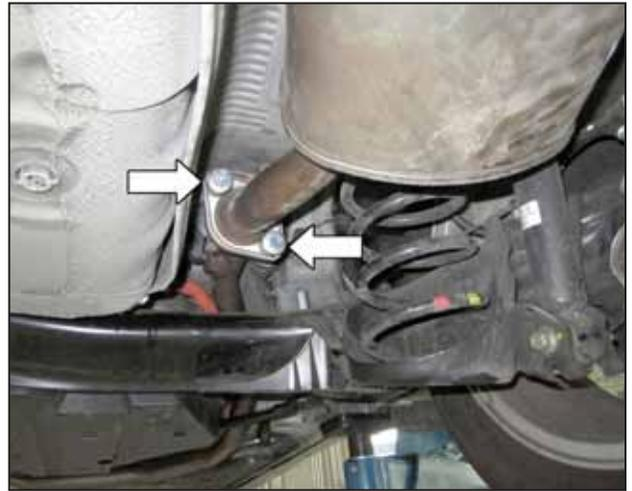
b. Remove the 2 bolts securing the OEM rear section to the mid pipe.
