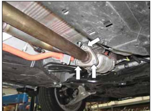
i. Secure the mid pipe to the OEM catalytic converter with the three supplied M10 nuts (RHNA-M10X125).
