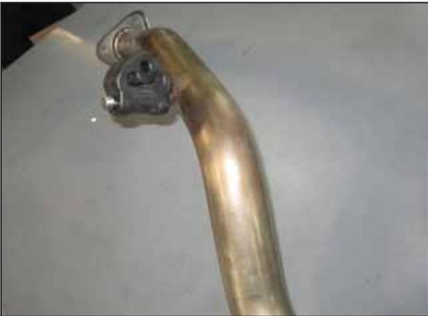
b. Install the OEM rubber mount removed in step 2f, onto the rear section of the AEM® exhaust (83035) as shown.
