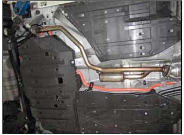
g. Install the AEM® mid pipe (83034) as shown by engaging the two rubber mounts.
