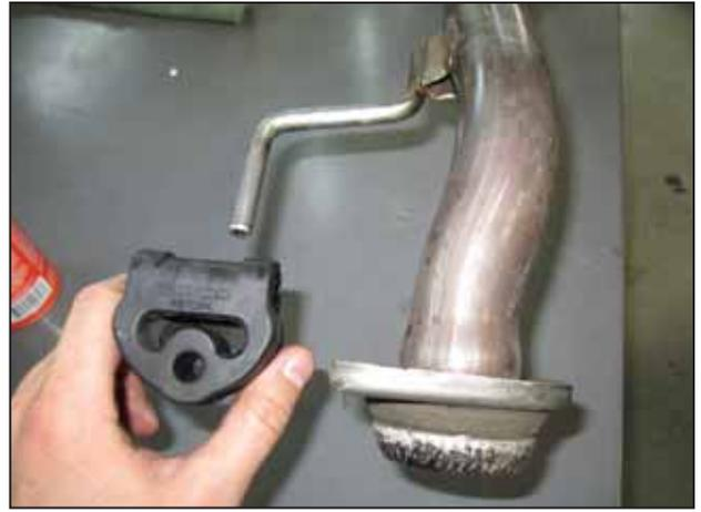
f. Remove the rear most rubber mount from the mid pipe as shown. Silicone spray will help with the removal.
