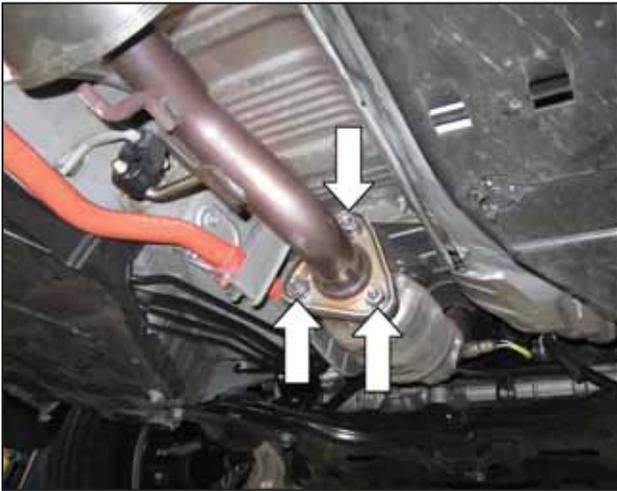
a. Remove the 3 nuts securing the OEM mid pipe to the catalytic converter.
