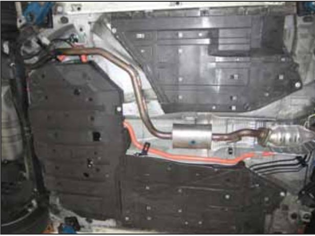
e. Disengage the remaining two rubber mounts and remove the mid pipe from the vehicle.
