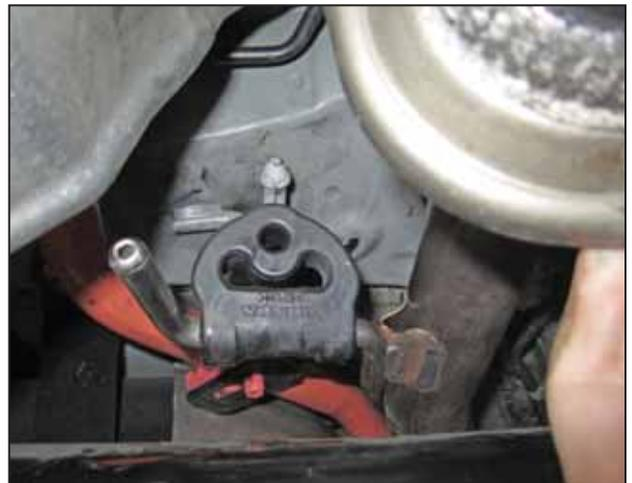
d. Disengage the rear most rubber mount on the mid pipe by sliding it off of the mount on the vehicle's side.
