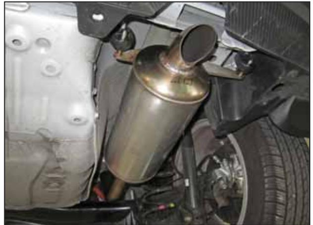
c. Install the rear section of the AEM® exhaust (83035) as shown, by engaging the two rubber mounts at the muffler.
