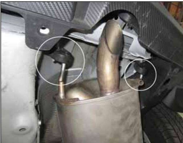
c. Remove the rear section by disengaging the two rubber mounts.
