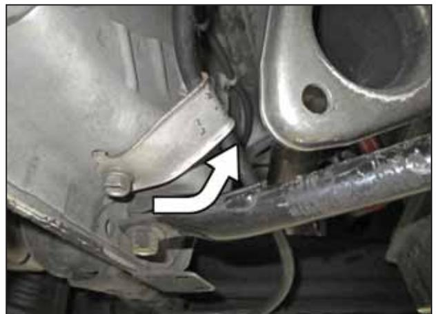
e. Bend the emergency brake bracket up out of the way as shown.
