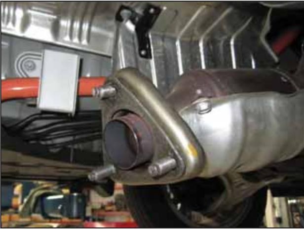
f. Install the supplied gasket (RM-CB84) on the OEM catalytic converter as shown.
