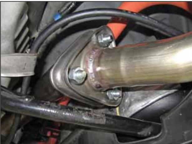
h. Install the supplied gasket (RM-CB84) between the AEM® mid pipe, and rear section. Hold it in place with the 3 supplied M10 bolts (RHBA-M10X125X25) and nuts (RHNA-M10X125).
